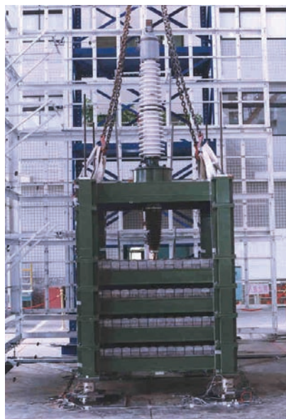
Figure 4-2 Transformer Model with the Bushing Mounted on the Top
