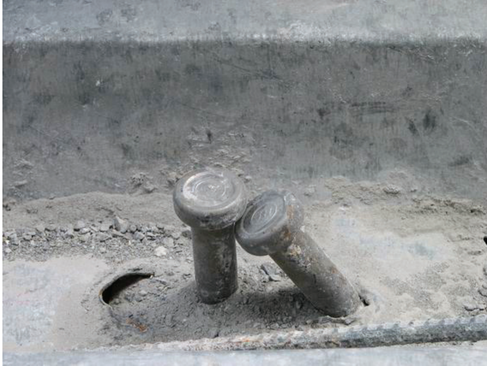
(c) Deformed Shear Stud in the Top Concrete Slab
