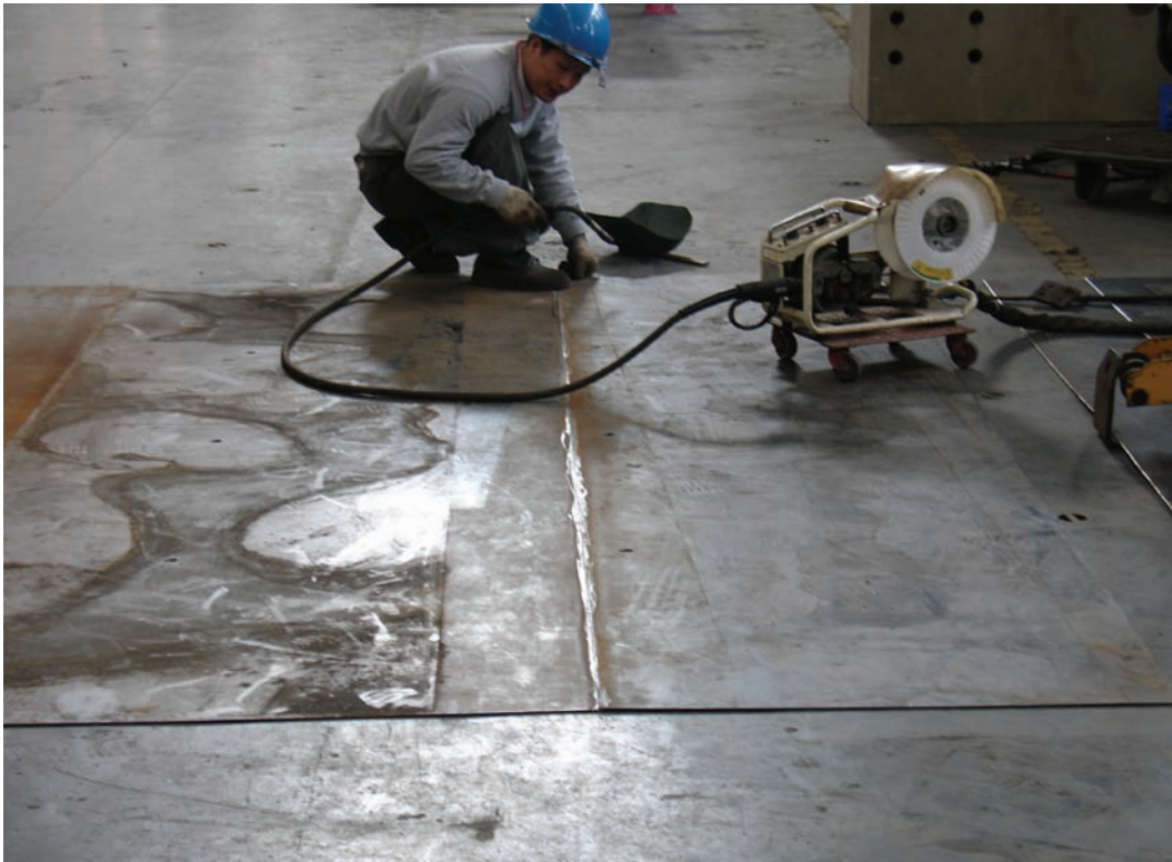
FIGURE 3-9 Manual Welds along Small Plate Segment Edges (Photo Courtesy of C.H.Lin and K.C.Tsai, NCRE)
