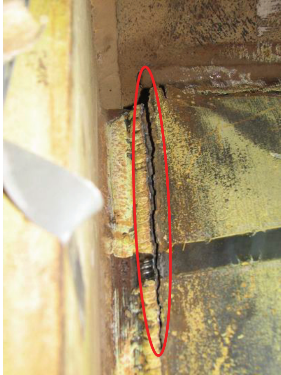
FIGURE 4-48 Vertical Plate Tear at the Upper North Corner of the First-Story Infill Panel
