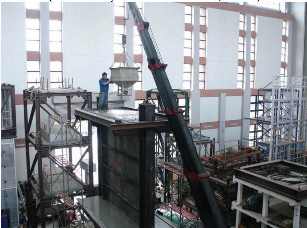
FIGURE 3-14 Casting Concrete Slab (Photo Courtesy of C.H.Lin and K.C.Tsai, NCREC)
