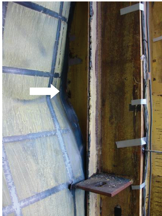
FIGURE 4-54 Failures of the Welds Connecting the First-Story Infill Panel to the Fish Plate Along the North VBE
