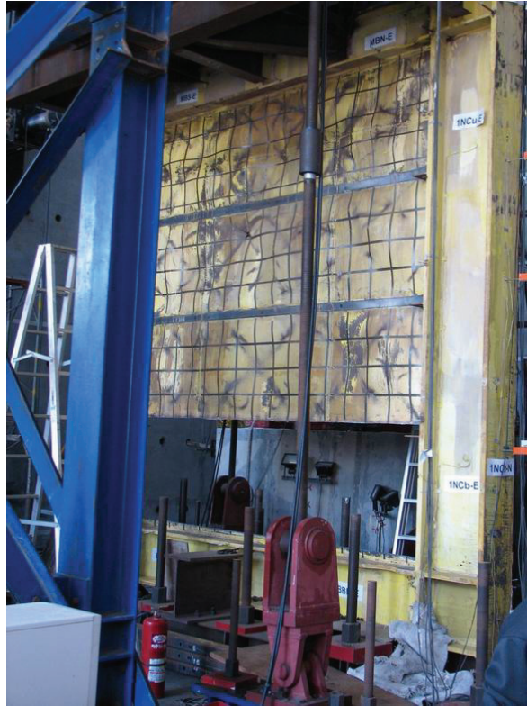
FIGURE 4-26 Specimen during the Infill Panel Removal
