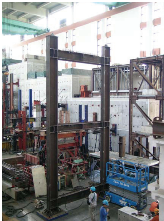
FIGURE 3-8 Installation of HBEs (Photo Courtesy of C.H.Lin and K.C.Tsai, NCRE)
