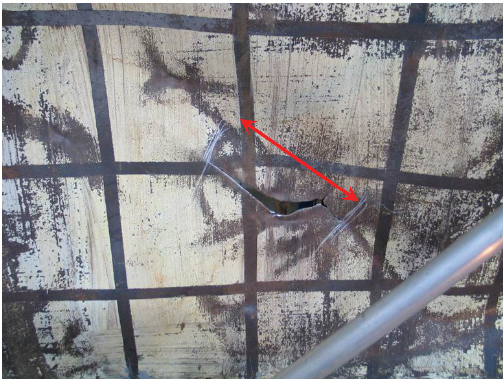
FIGURE 4-25 Panel Tear in the First-Story Infill Panel (at the End of Test 4)
