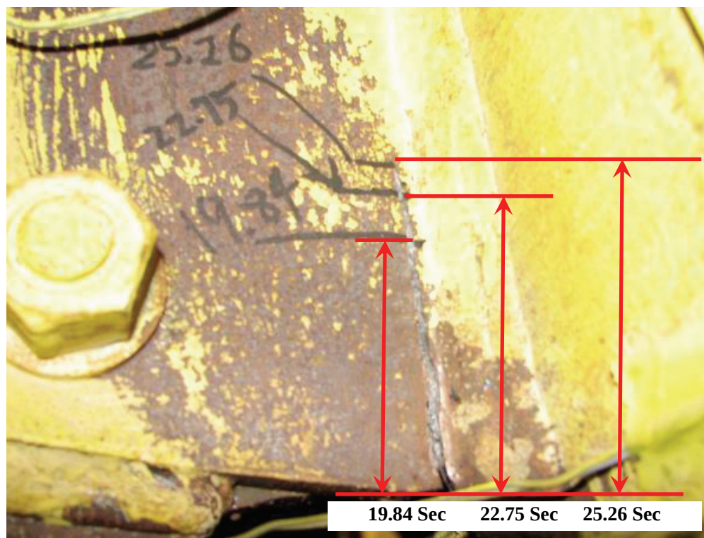
FIGURE 4-45 Development of the Fracture at the Bottom of the Shear Tab at the North End of the Intermediate HBE
