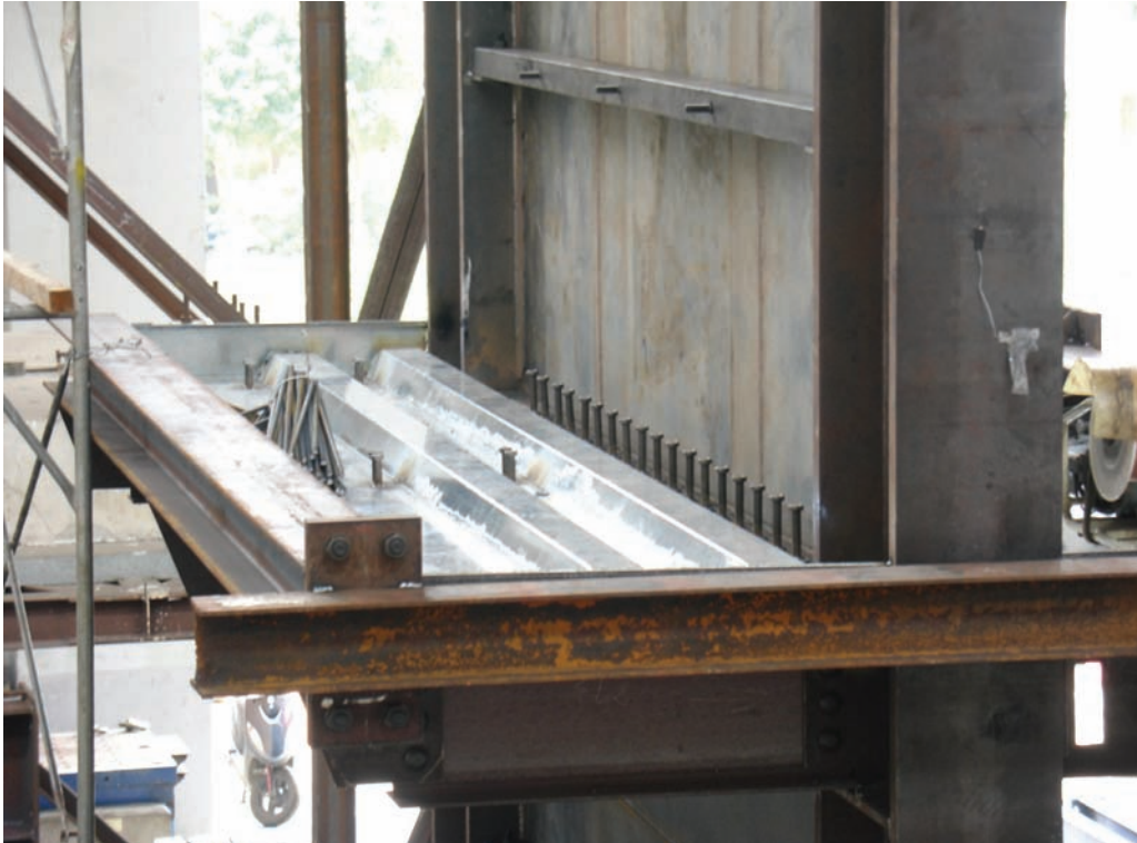
FIGURE 3-13 Corrugated Steel Deck (Photo Courtesy of C.H.Lin and K.C.Tsai, NCREC)
