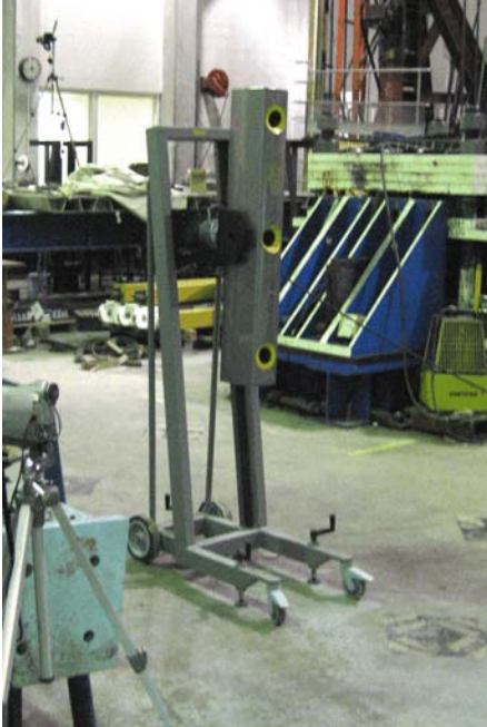
FIGURE 5-15 Krypton K600 Coordinate Measurement Machine (a) Front View and (b) Position in Front of Specimen during Testing
