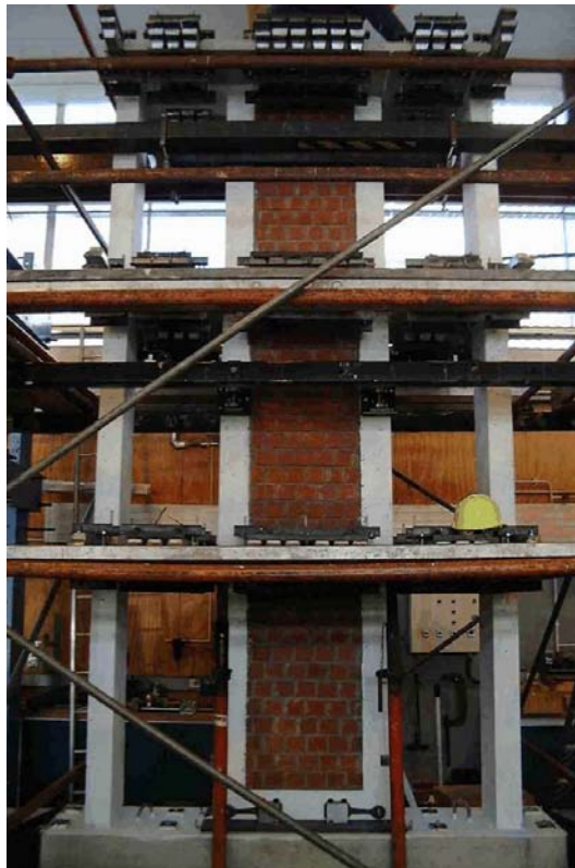
FIGURE 2-4 Rocking Wall Specimen with Flexural Steel Yielding Devices at Uplifting Location (Toranzo et. al., 2001)
