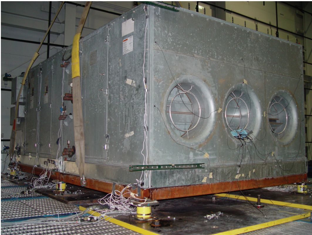
Figure 5-8 Test Setup, Phase II: Rigidly Mounted Test Specimen
