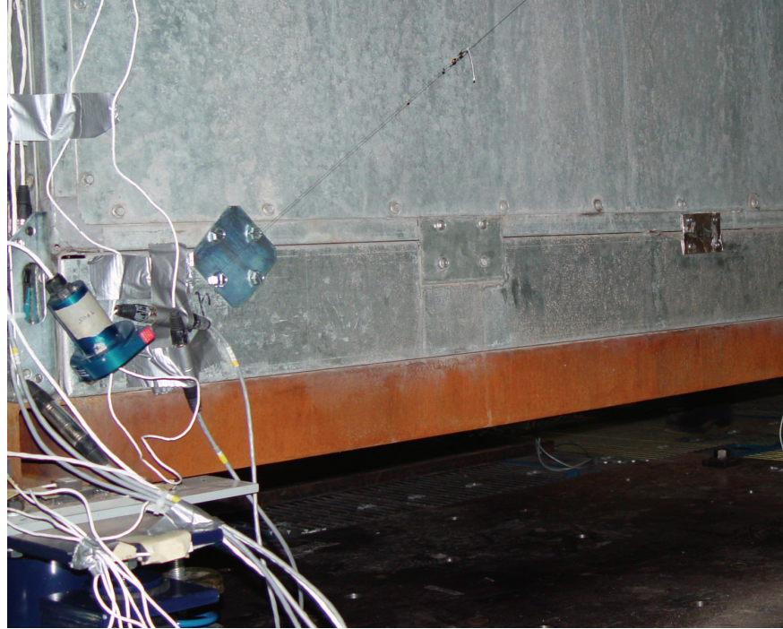
Figure 4-9 Displacement Transducers on West Face of Test Specimen, Channel#113, Phase I: Isolated Test Specimen
