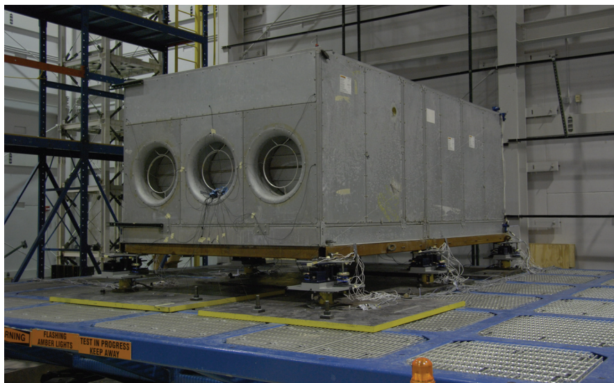
Figure 2-1 Test Specimen: Air-Handling Unit
