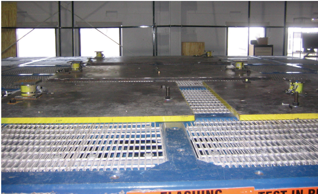
Figure 5-6 Six Load Cells Bolted to Interface Plates
