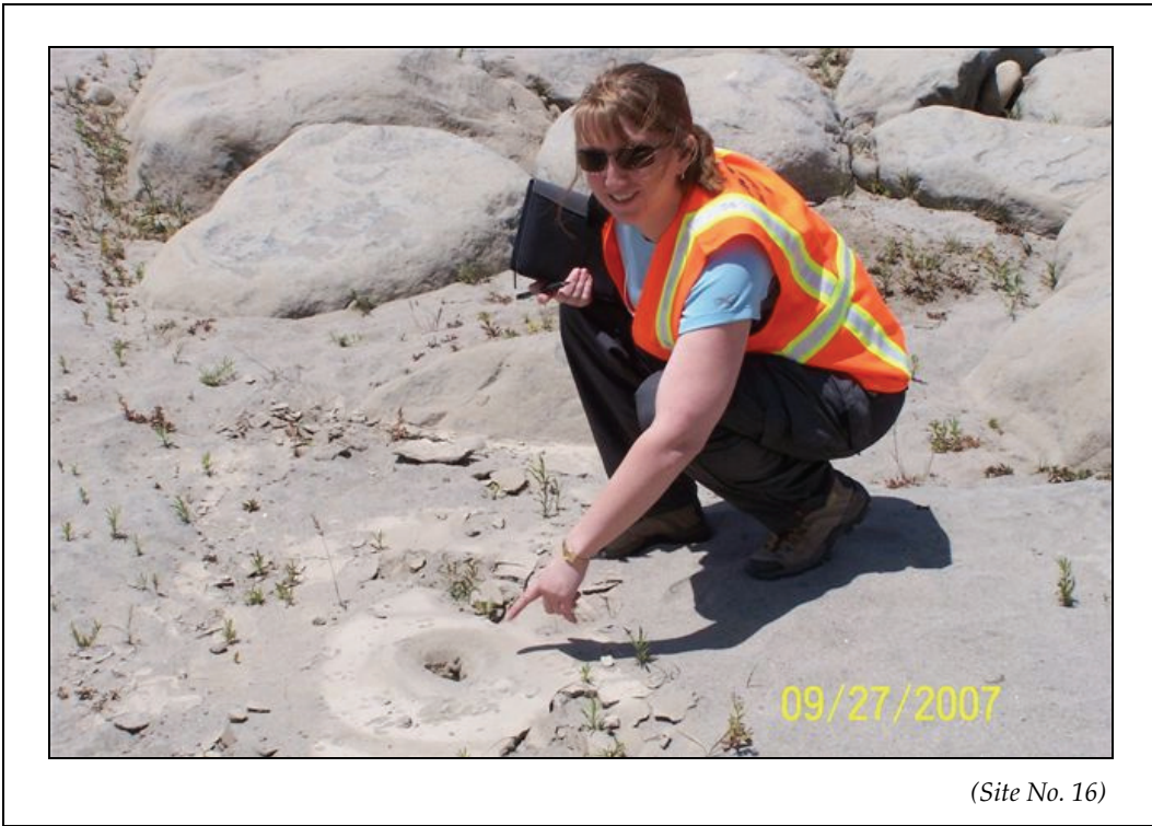
Figure 5-44. Monique Nykamp pointing to sand boil as evidence of liquefaction in river bed of Rio Ica at Puente Los Molinos.
