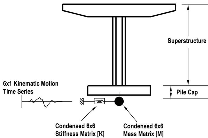
**Figure 2.1 Modeling of Pile Foundation for Seismic Design of Bridges**
