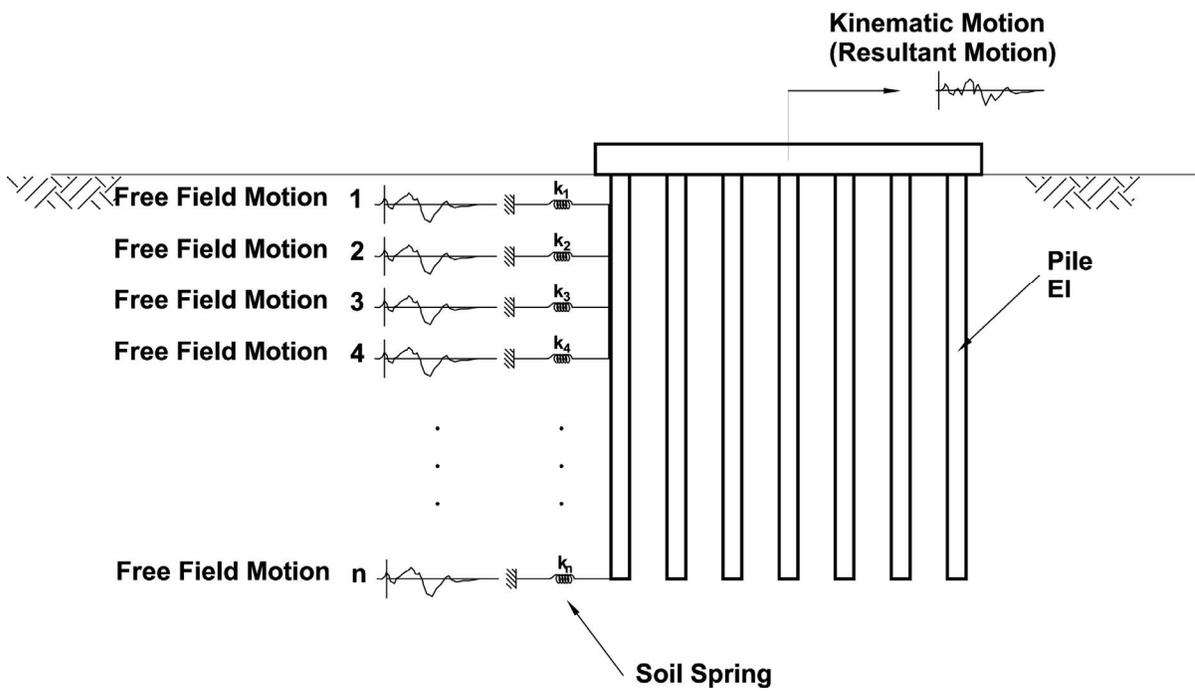
Figure 4.12 Schematic of Kinematic Motion
