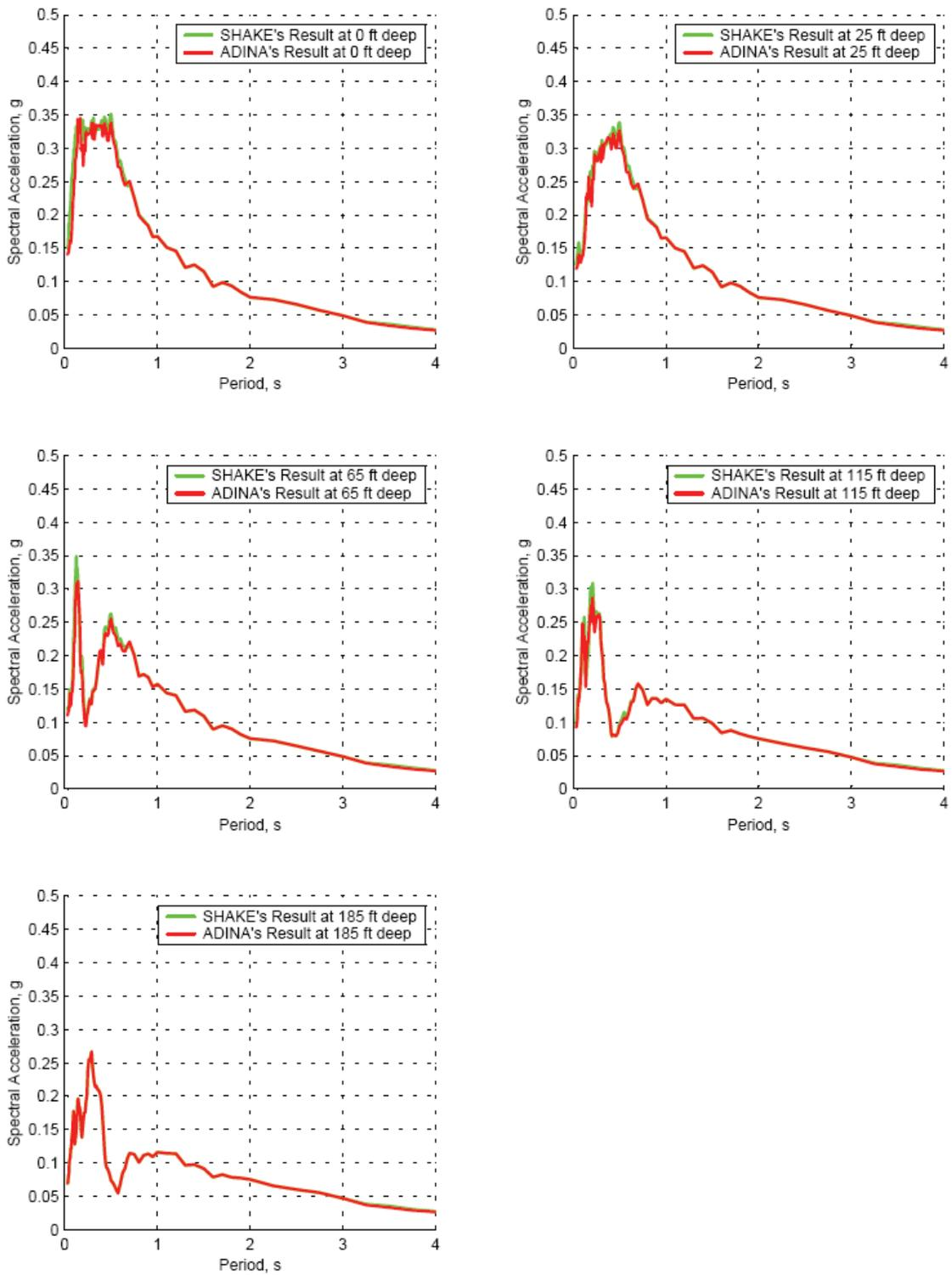
**Figure 3.10 Comparison of SHAKE Results and ADINA Results of the Model with Slaving Left and Right Boundaries**
