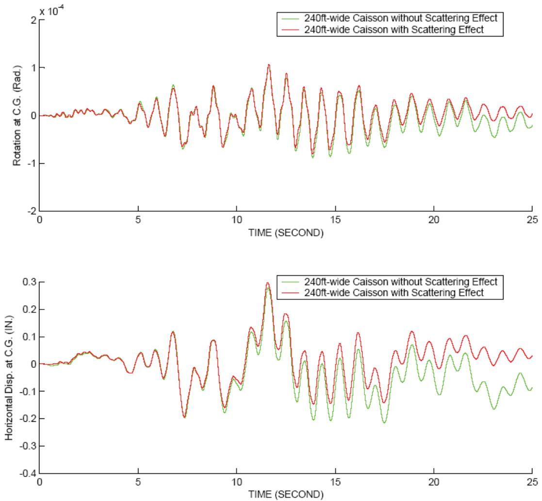
**Figure 5.13 Seismic Response of Caisson with the Base Width of 240 feet**
