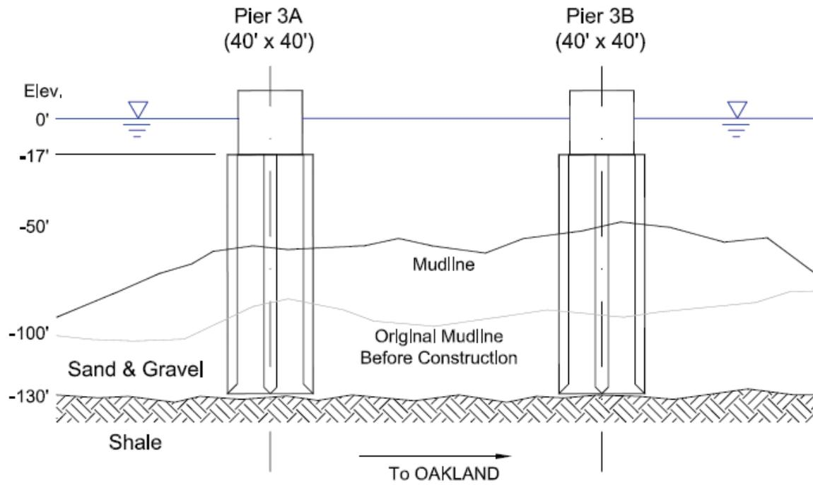
**Figure 5.3 Multiple Caissons at Pier 3 of Carquinez Bridge, CA**
