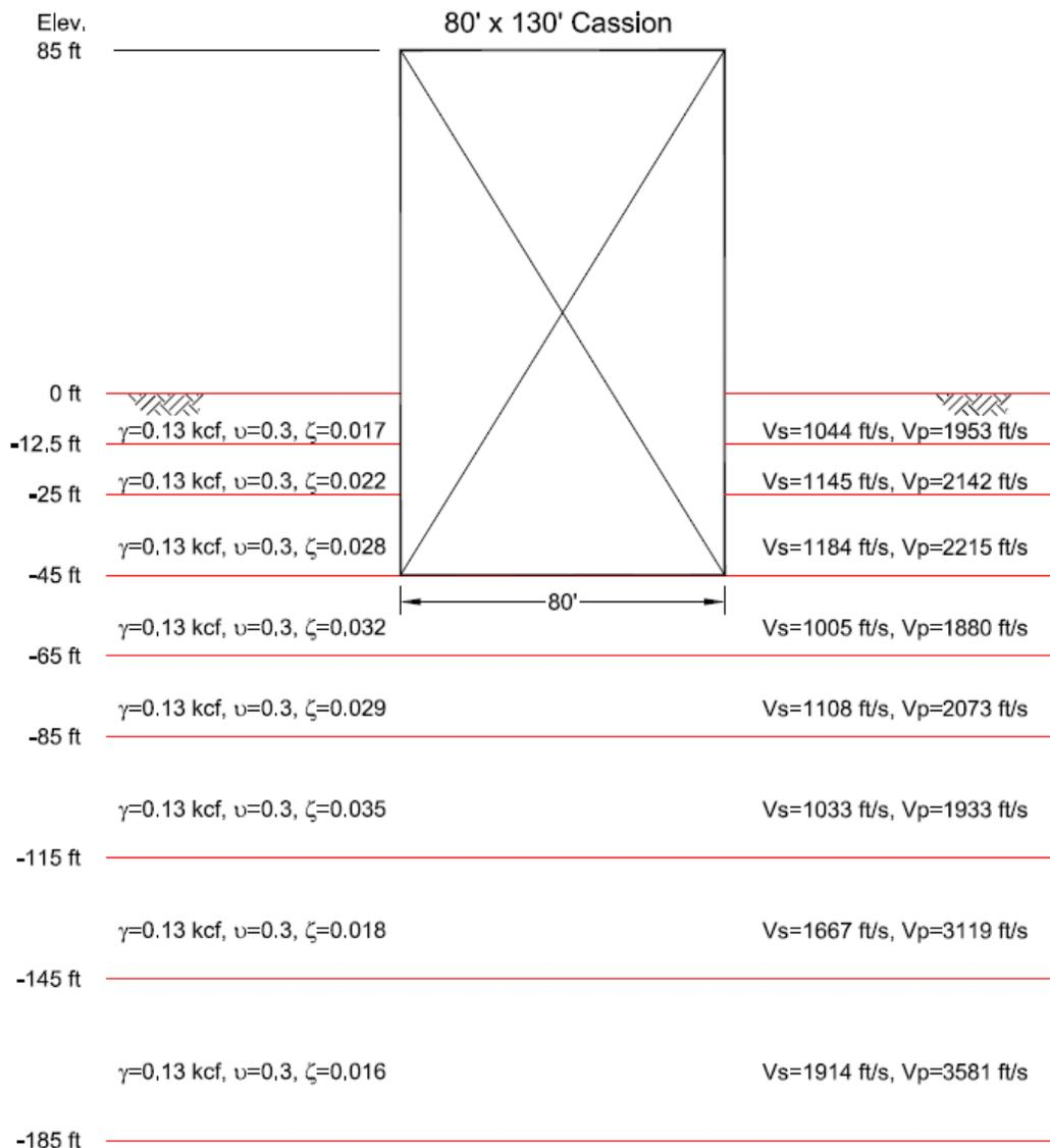
**Figure 5.9 Caisson Dimensions and Soil Data**
