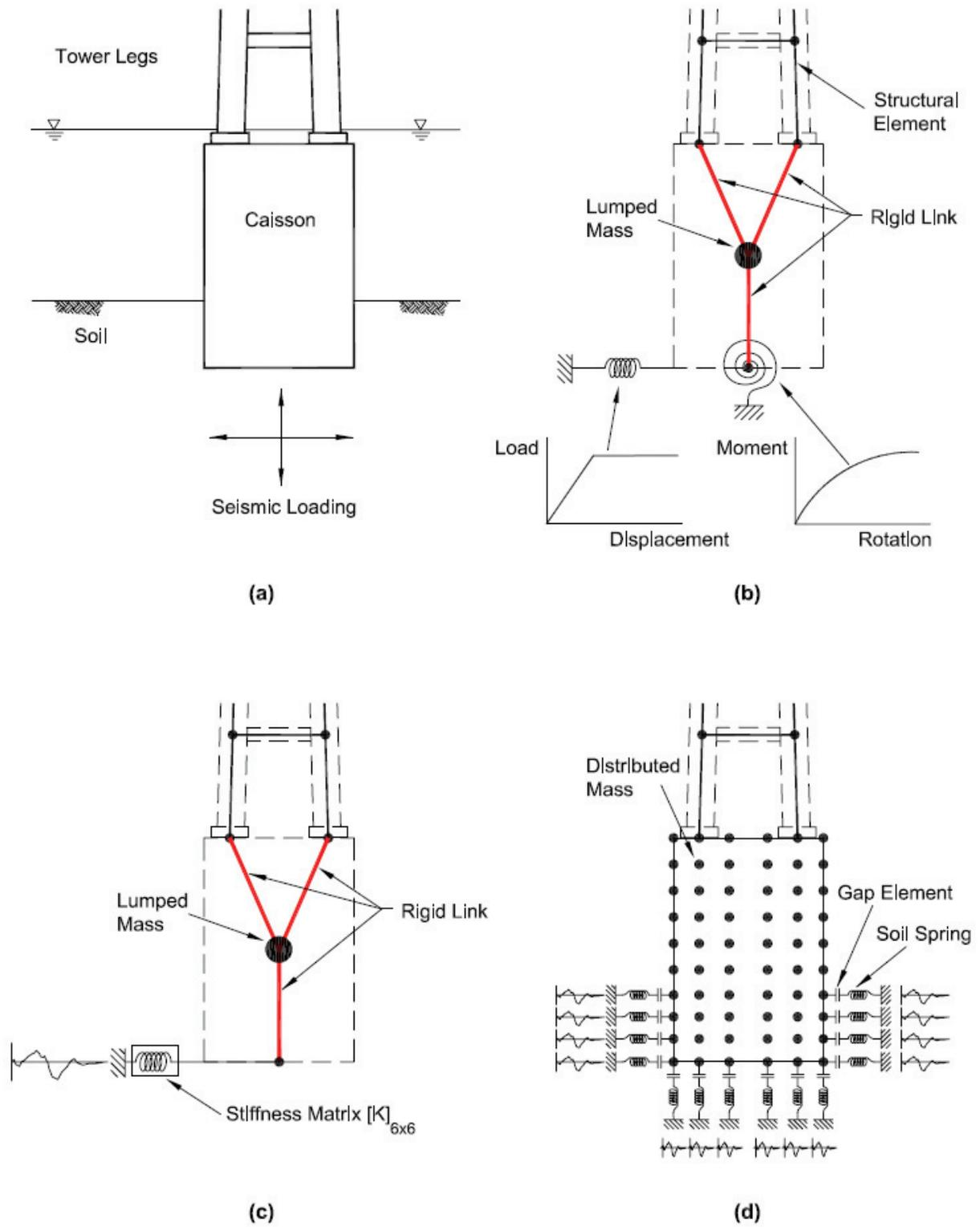
**Figure 2.2 Various Modeling Techniques for Gravity Caisson**
