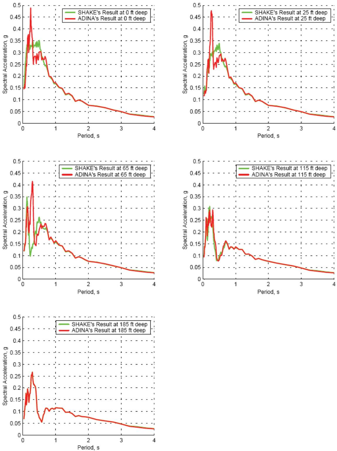
**Figure 3.9 Comparison of SHAKE Results and ADINA Results of the Model with Two Edge Columns**
