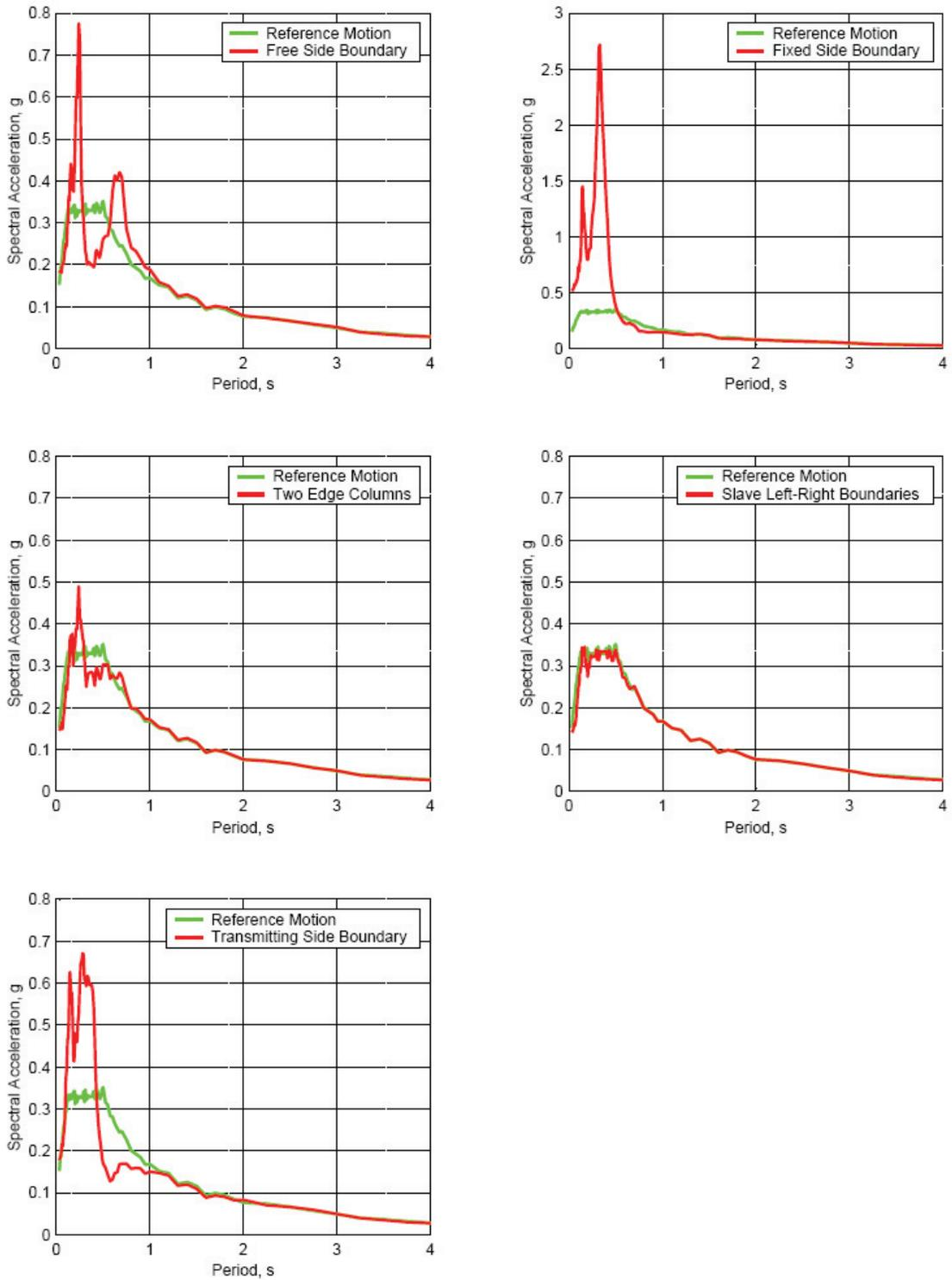
**Figure 3.8 Effects of Side Boundary Conditions**
