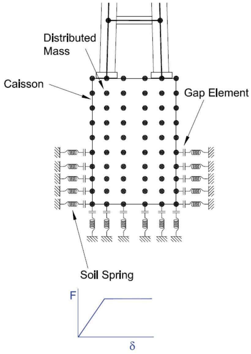
**Figure 5.8 Distributed Mass and Soil Springs**
