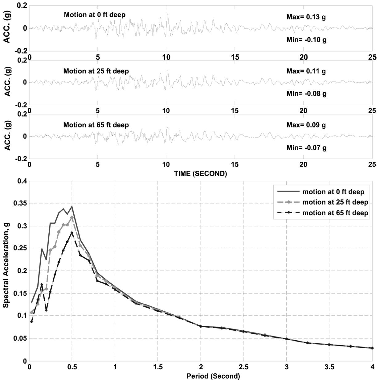
**Figure 4.7 SASSI Results of Computed Time Histories and Response Spectra at Three Selected Locations**
