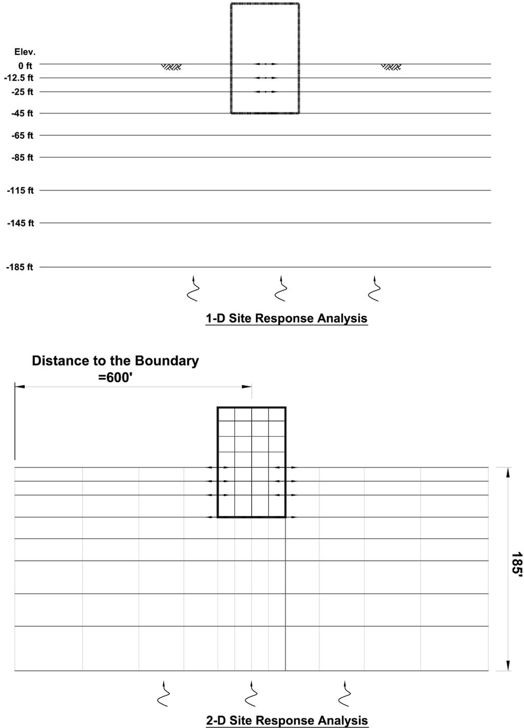
**Figure 5.10 1D versus 2D Site Response Analysis**
