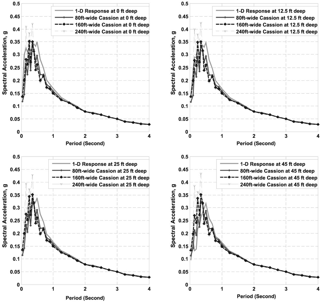
Figure 5.12 Near-Field Motions of Three Caisson Sizes
