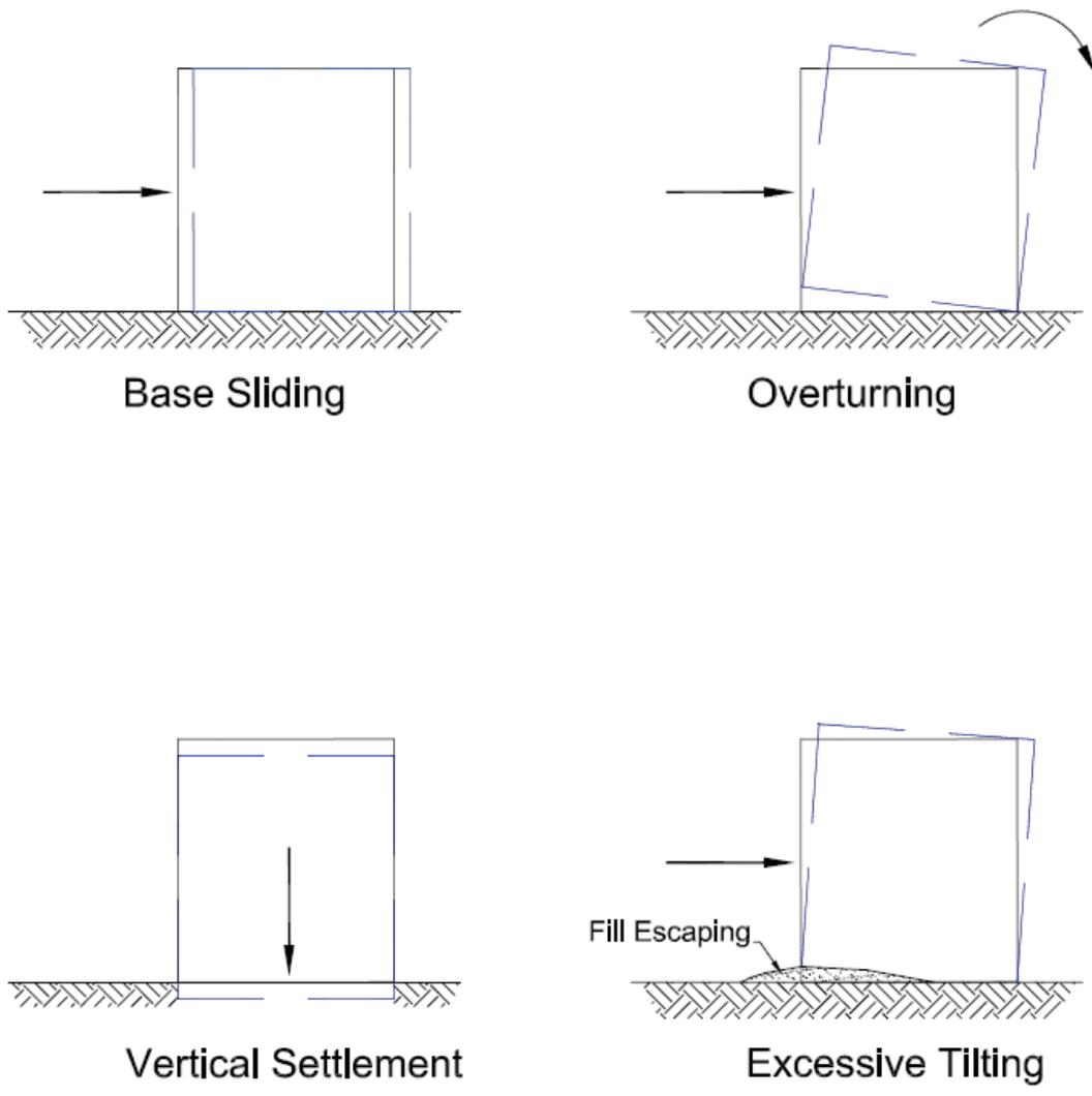
**Figure 5.1 Possible Failure Modes of Caissons**
