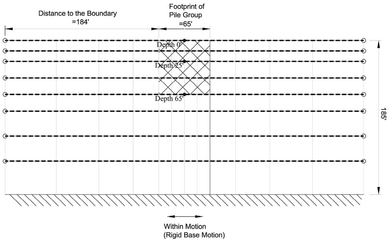
**Figure 4.8 ADINA Model of Pile Group with Slaving of the Two Side Boundaries**
