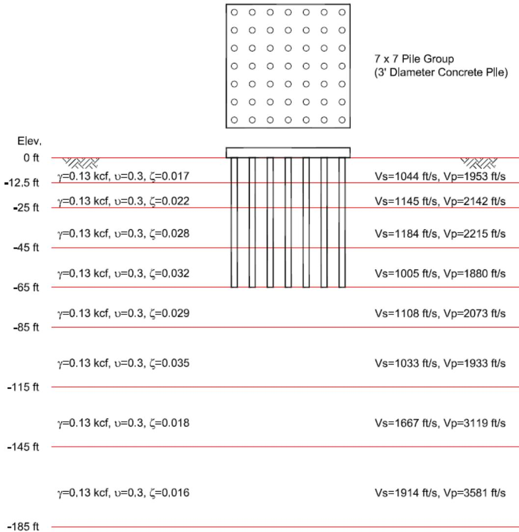
**Figure 4.5 Hypothetical Pile Foundation and Soil Strata**
