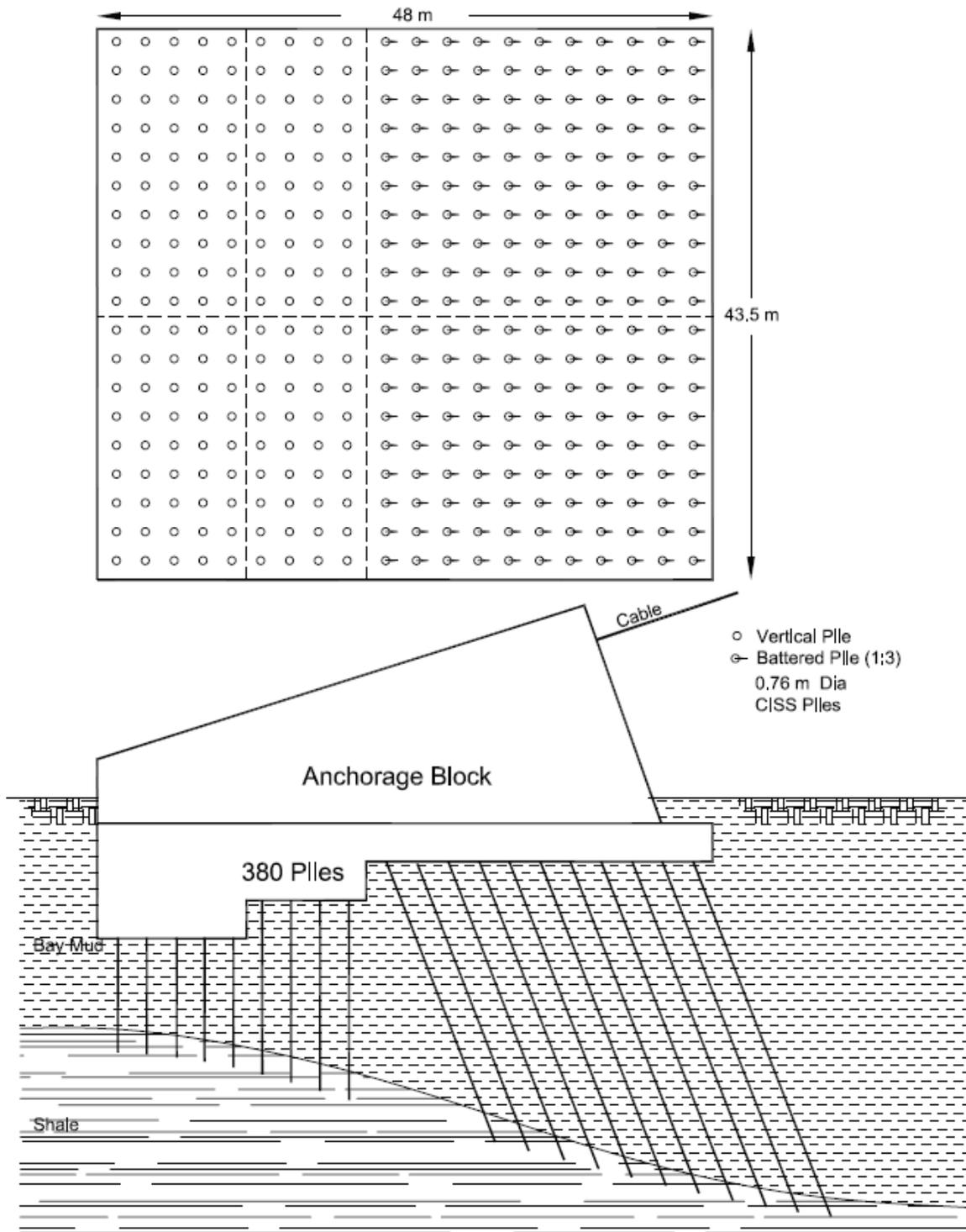
**Figure 4.1 South Anchorage Foundation of New Carquinez Bridge, CA**
