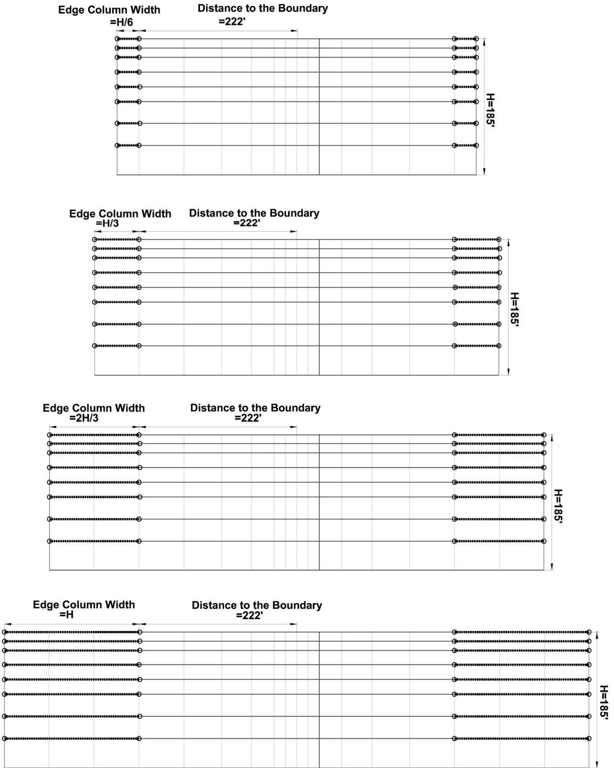
Figure 3.11 FEM Model with Different Edge Column Widths
