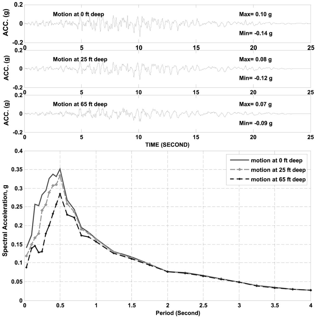
**Figure 4.9 ADINA Results of Computed Time Histories and Response Spectra at Three Selected Locations**
