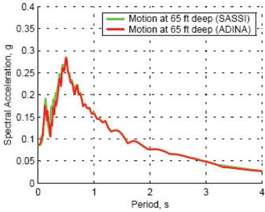
**Figure 4.10 Comparisons Between SASSI and ADINA Response Spectra**
