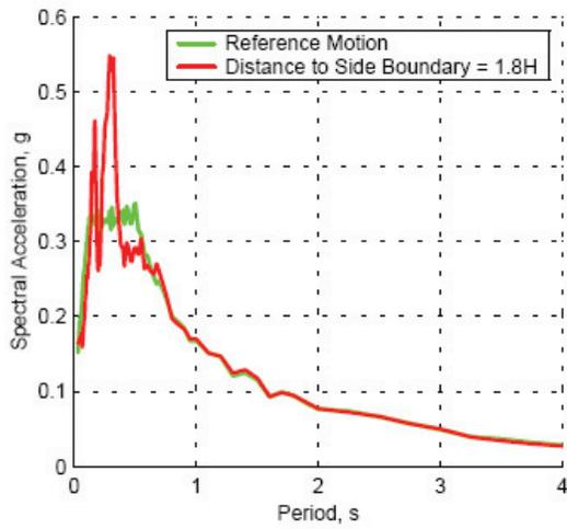
**Figure 3.13 Effect of Different Distances to Boundary**
