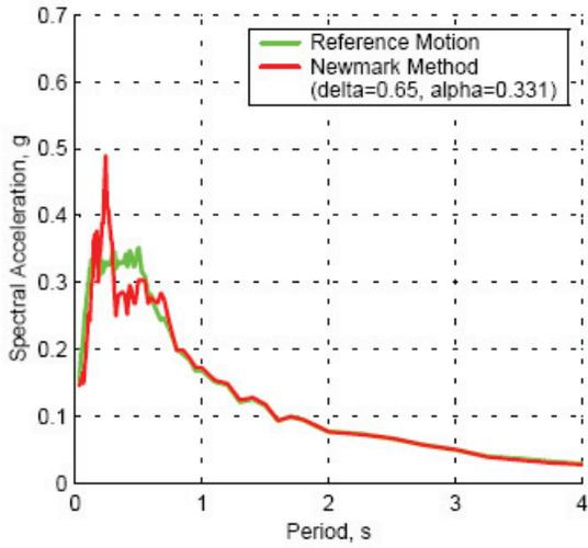
**Figure 3.14 Effect of Different Integration Scheme**
