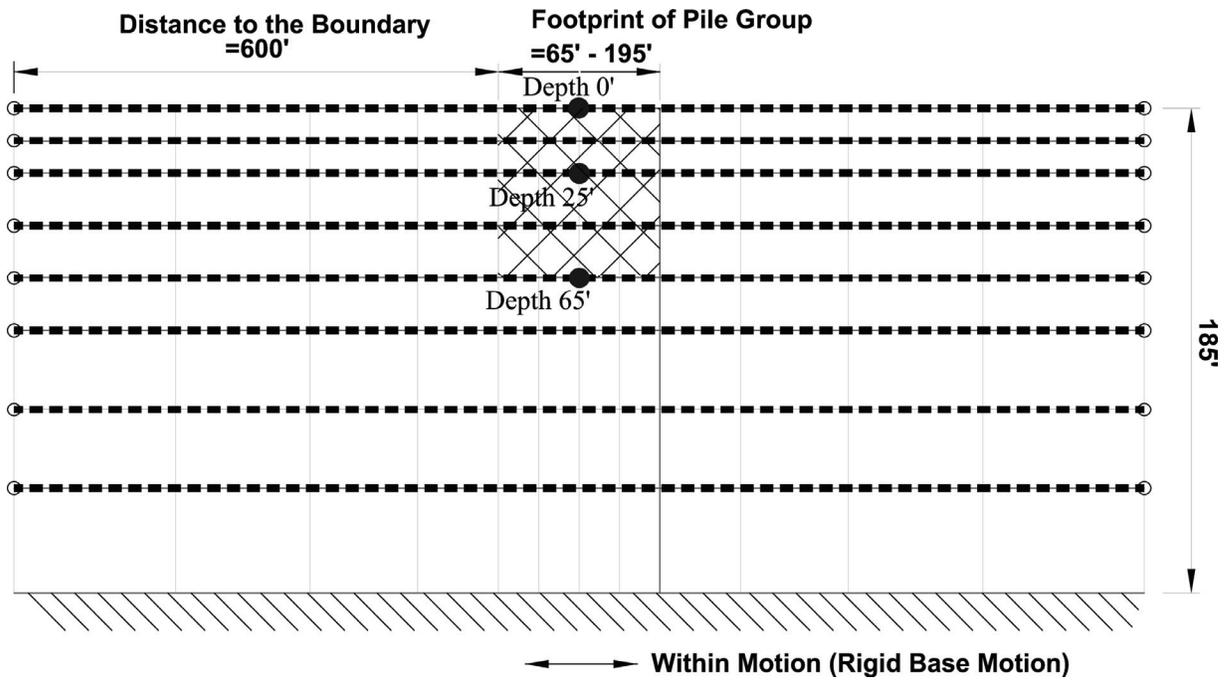
Figure 4.11 ADINA Model to Study Effects of Larger Pile Foundation Size
