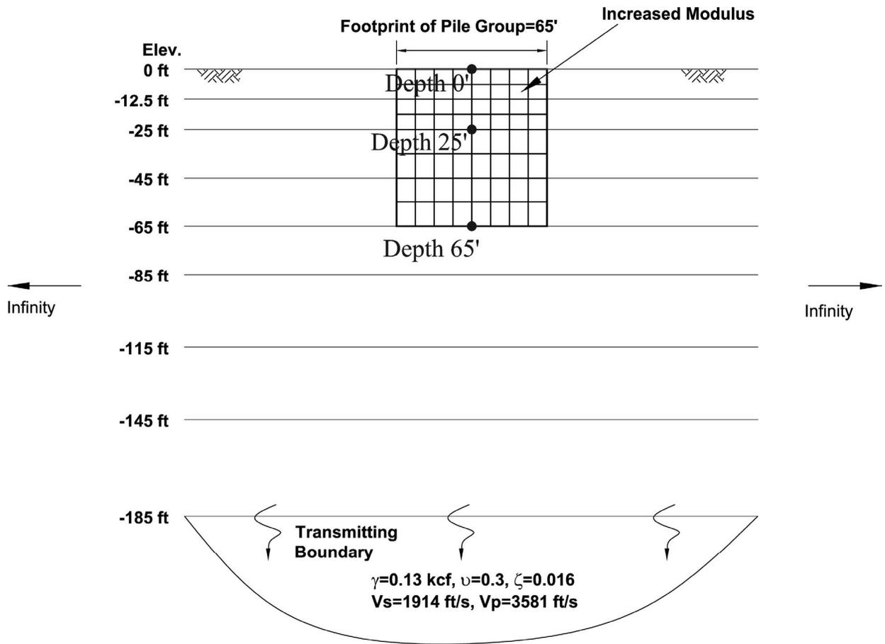
**Figure 4.6 Conceptual SASSI Model of Pile Group**
