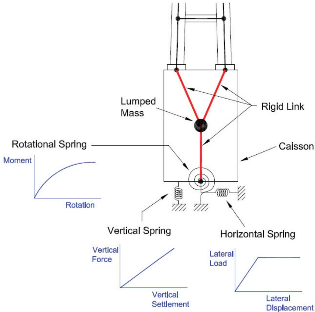
**Figure 5.7 Lumped Mass with Nonlinear Uncoupled Springs**
