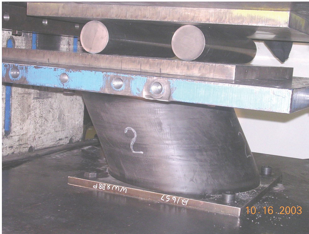
FIGURE 8-14 Lead-Rubber Bearing During High Speed Testing
