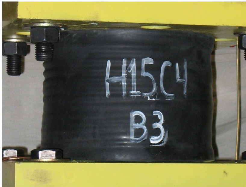
FIGURE 7-14 Rubber Bearing at Tensile Deformation of 60% of the Total Rubber Thickness
