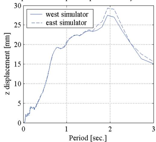
f. displacement response spectra in the z-direction
