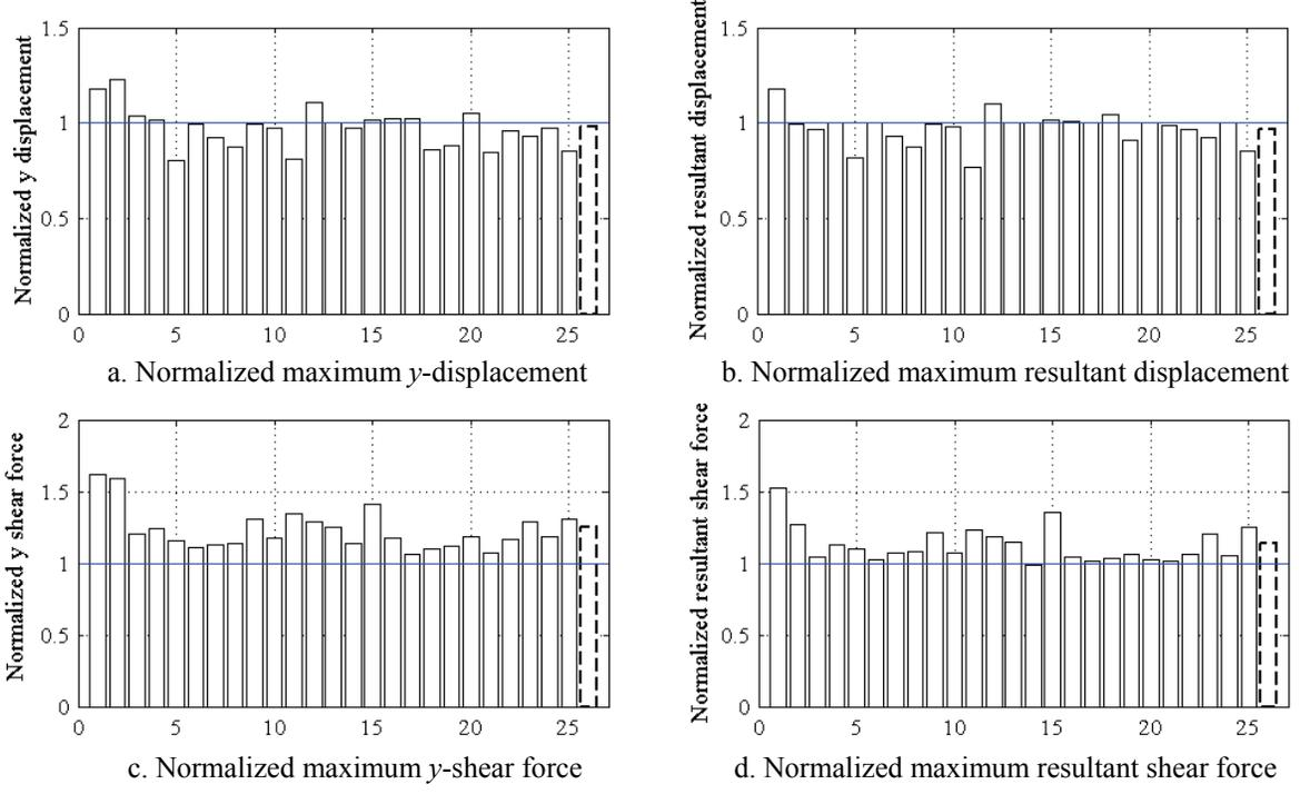
**Figure 8-17** Maximum response of the orthotropic configuration O4 normalized by the maximum response of the isotropic configuration I1 (O4/I1) and friction property FA for the far-field set of ground motions
