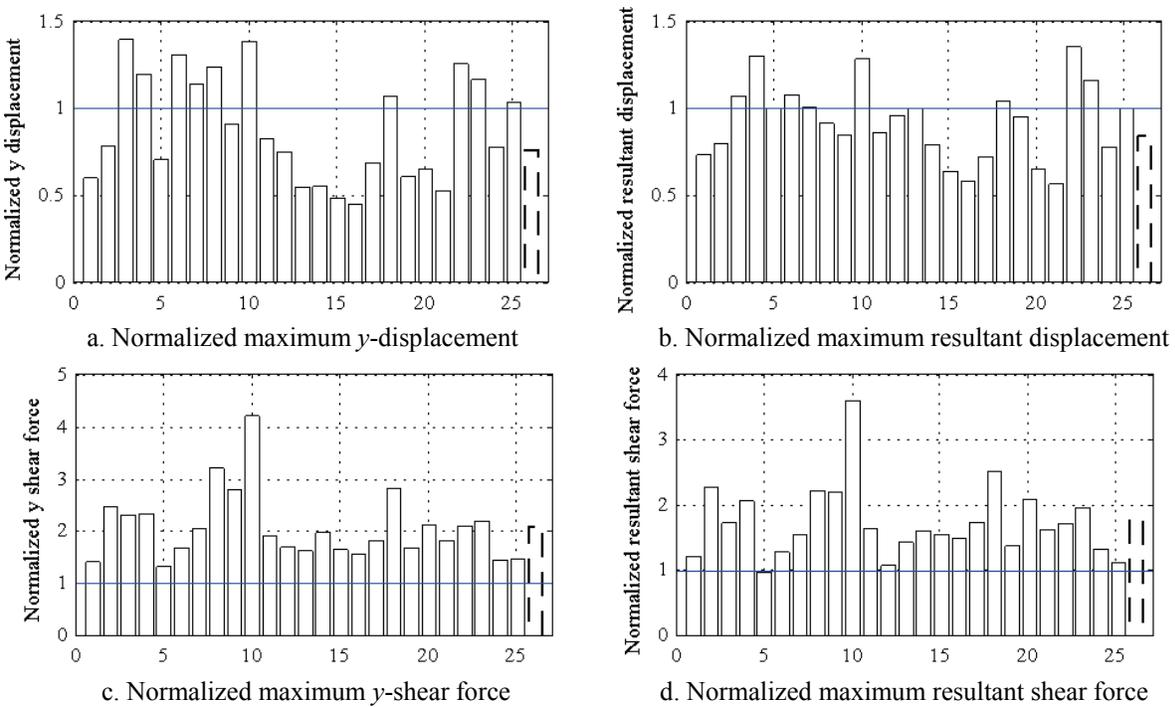
**Figure 8-8** Maximum response of the orthotropic configuration O2 normalized by the maximum response of the isotropic configuration I1 (O2/I1) for the near-field set of ground motions and friction property FA
