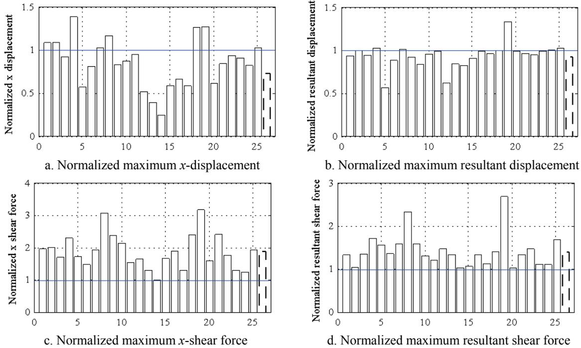
**Figure 8-7** Maximum response of the orthotropic configuration O1 normalized by the maximum response of the isotropic configuration I1 (O1/I1) for the near-field set of ground motions and friction property FA
