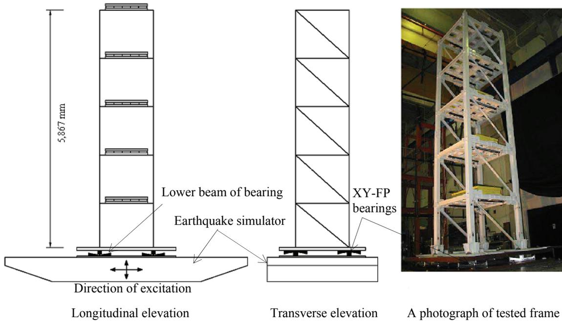
**Figure 2-15 1/4-length-scale isolated frame with XY-FP bearings (Roussis, 2004)**
