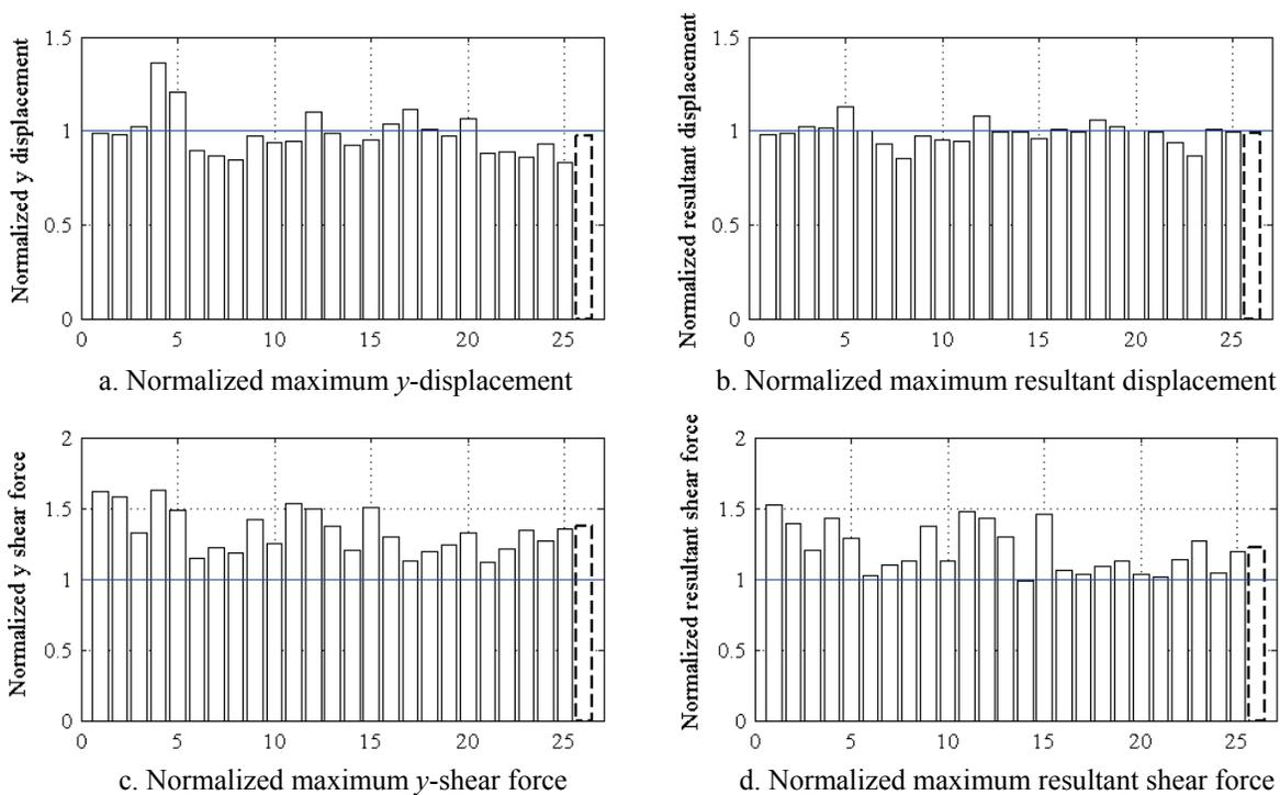
**Figure 8-19** Maximum response of the orthotropic configuration O6 normalized by the maximum response of the isotropic configuration I2 (O6/I2) and friction property FA for the far-field set of ground motions
