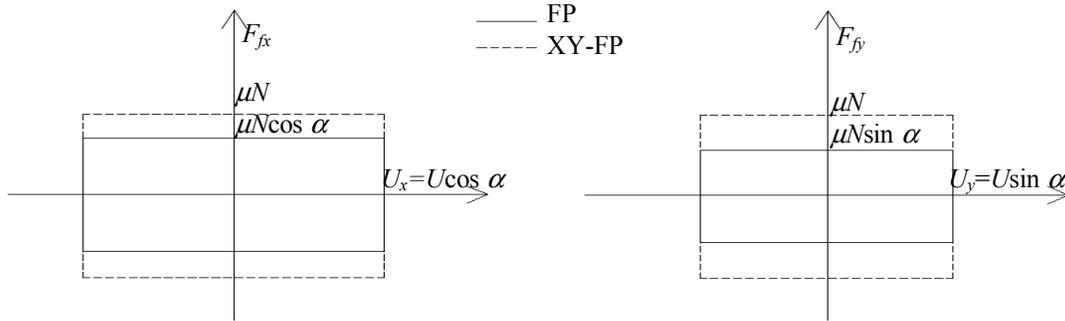
**Figure 3-16 Friction force-displacement loops in unidirectional motion**
