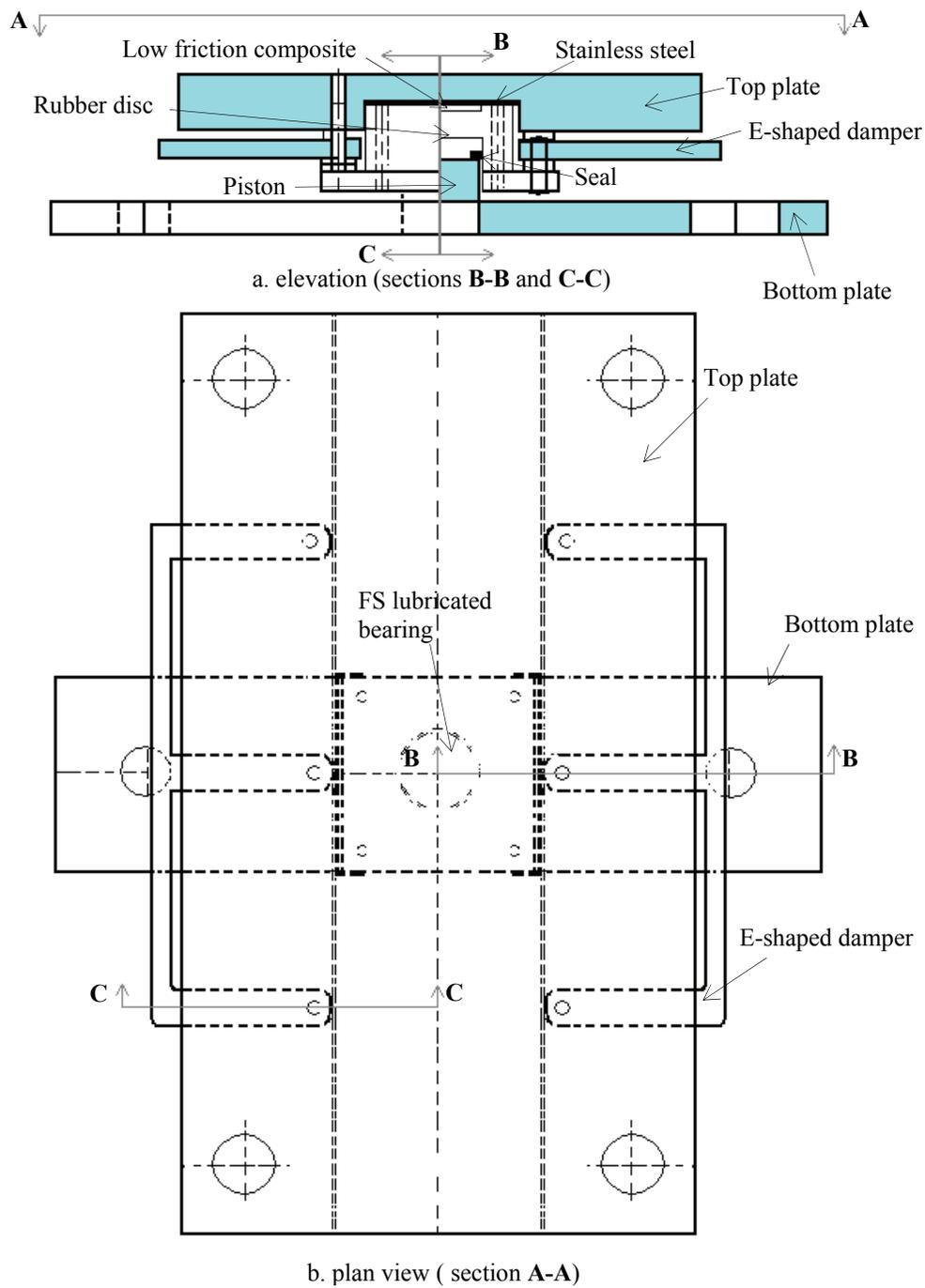
**Figure 2-4 Lubricated sliding bearing with E-shaped steel dampers (Tsopeles et al., 1994c)**
