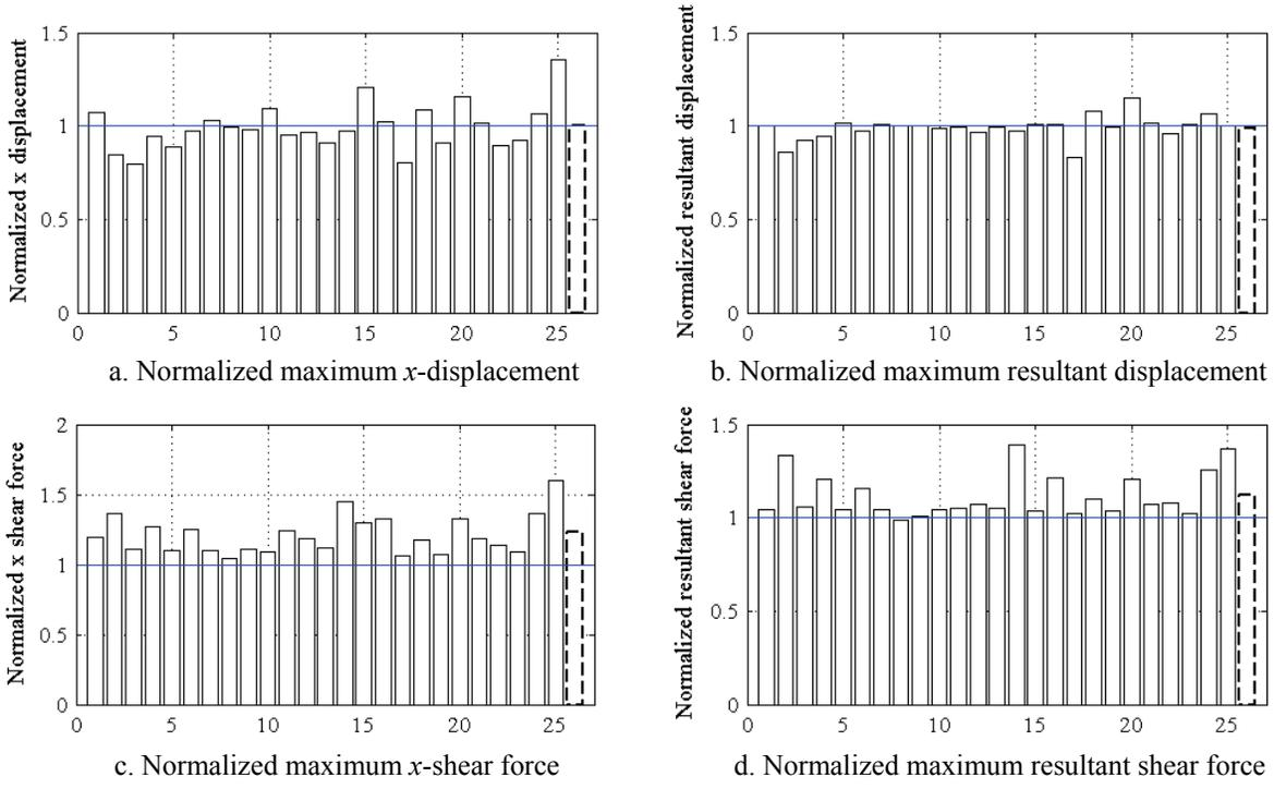
**Figure 8-16** Maximum response of the orthotropic configuration O3 normalized by the maximum response of the isotropic configuration I1 (O3/I1) and friction property FA for the far-field set of ground motions
