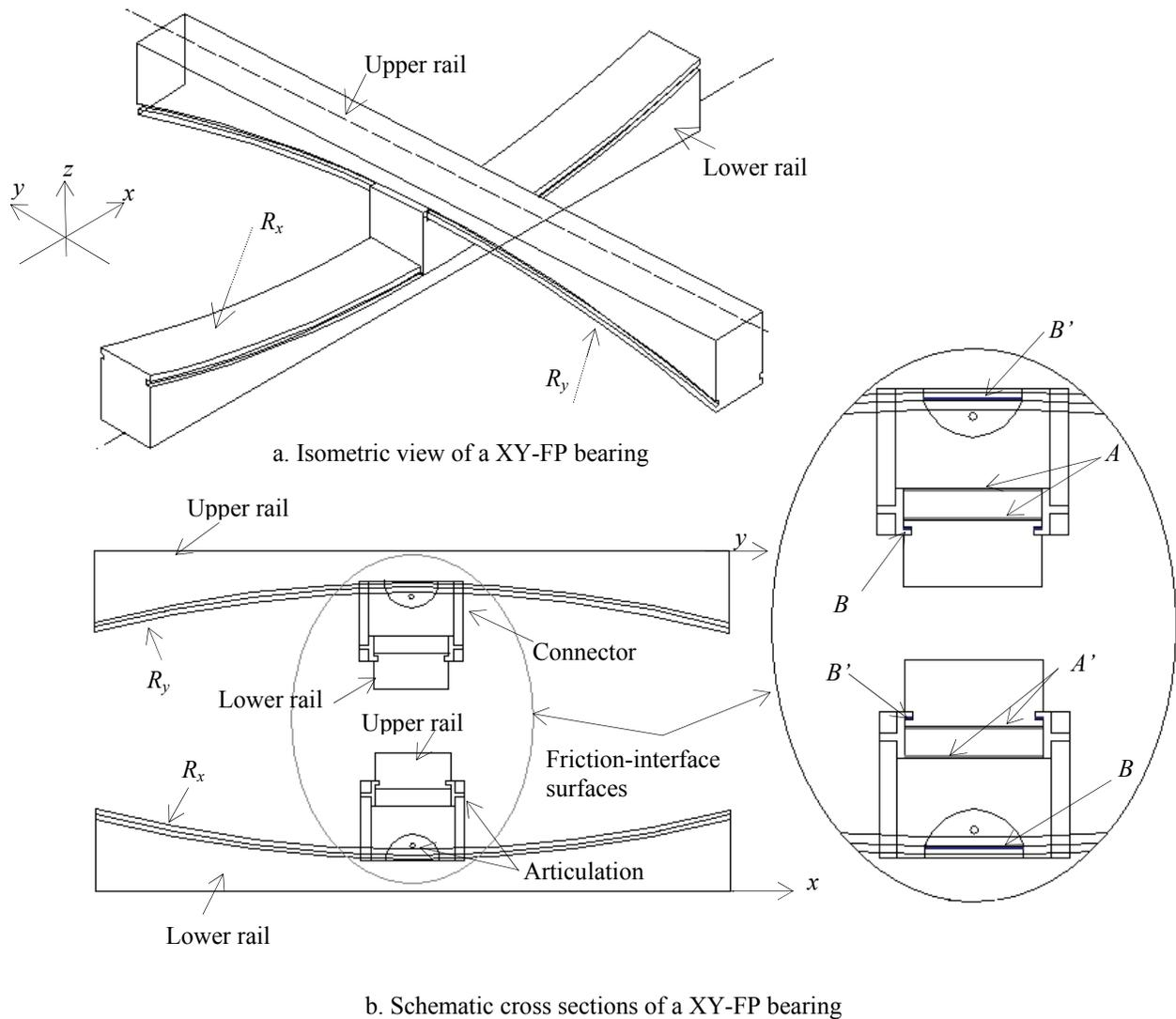
(A and A' are the friction interfaces of the bearing in compression. B and B' are the friction interfaces of the bearing in tension)
