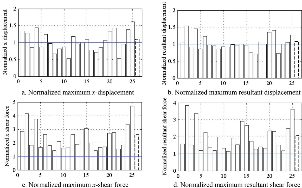
**Figure 8-24** Maximum response of the orthotropic configuration O1 normalized by the maximum response of the isotropic configuration I1 (O1/I1) and friction property FB for the far-field set of ground motions
