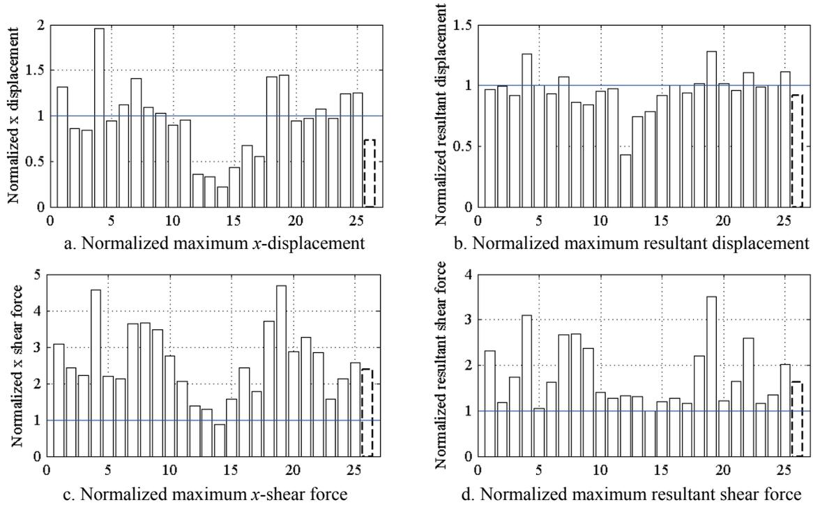
**Figure 8-21** Maximum response of the orthotropic configuration O1 normalized by the maximum response of the isotropic configuration I1 (O1/I1) and friction property FB for the near-field set of ground motions
