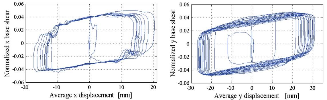
b. Global force-displacement loops for test F81xy (excitation frequency:  $x=0.4$  Hz and  $y=0.8$  Hz)
