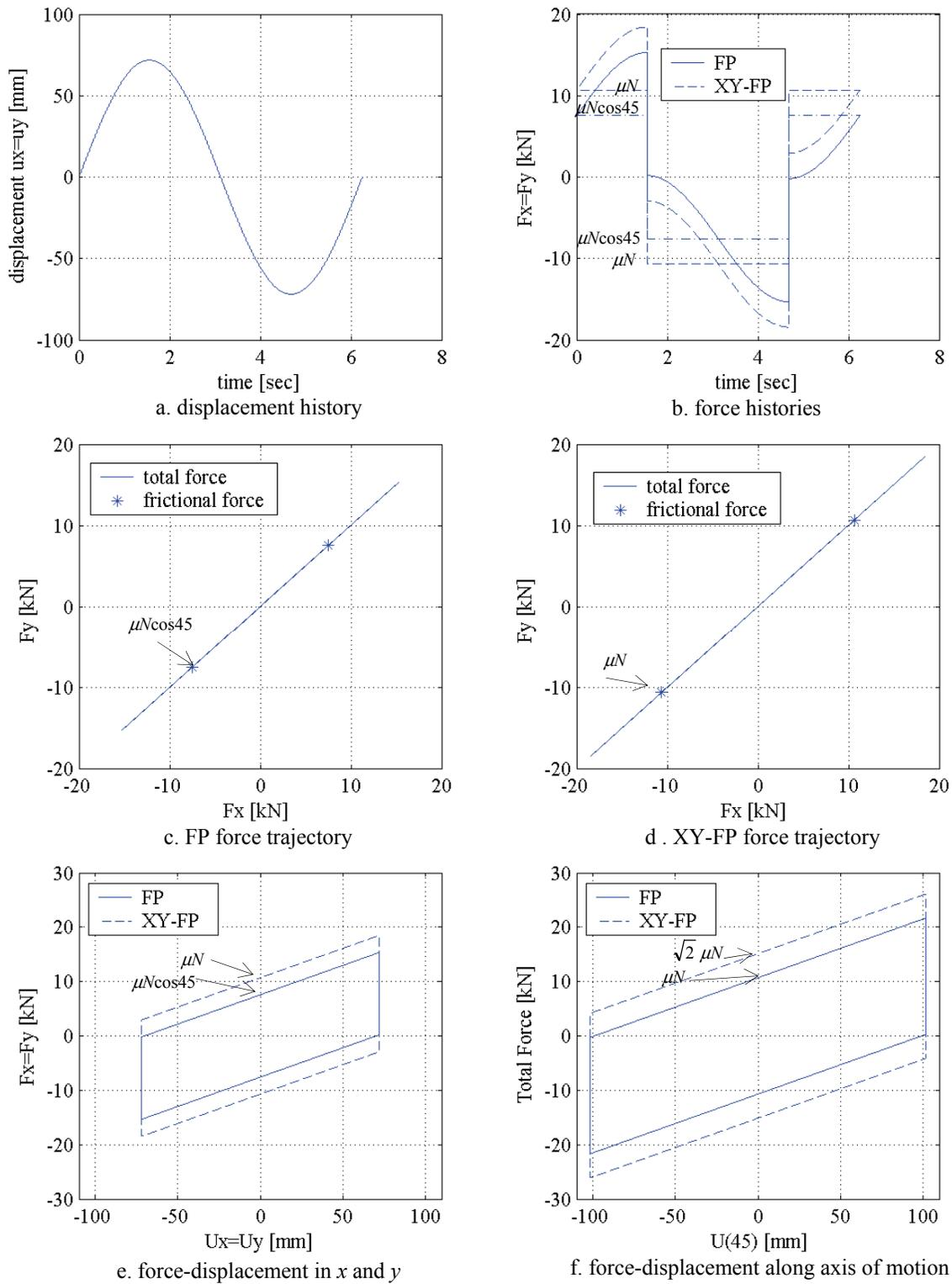
**Figure 3-17 Unidirectional motion oriented 45° to the x-axis**
