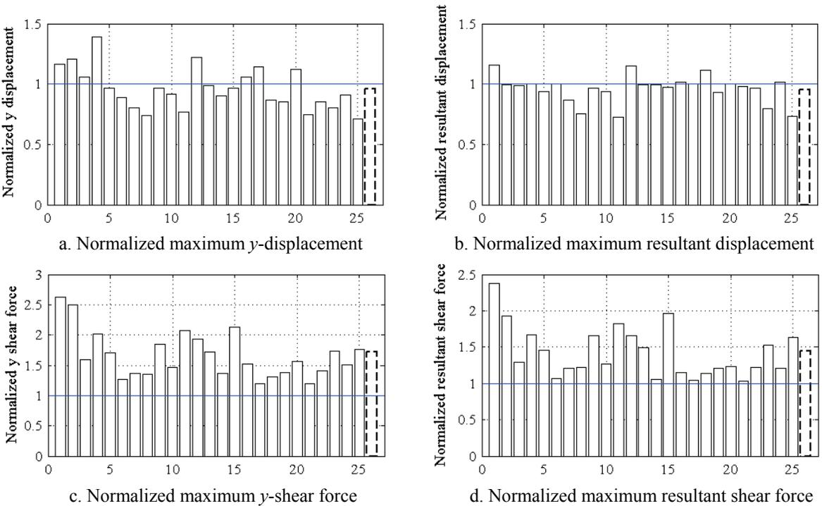
**Figure 8-15** Maximum response of the orthotropic configuration O2 normalized by the maximum response of the isotropic configuration I1 (O2/I1) and friction property FA for the far-field set of ground motions
