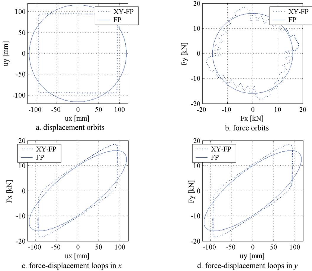
**Figure 3-29** Steady-state response to the circular acceleration orbit
