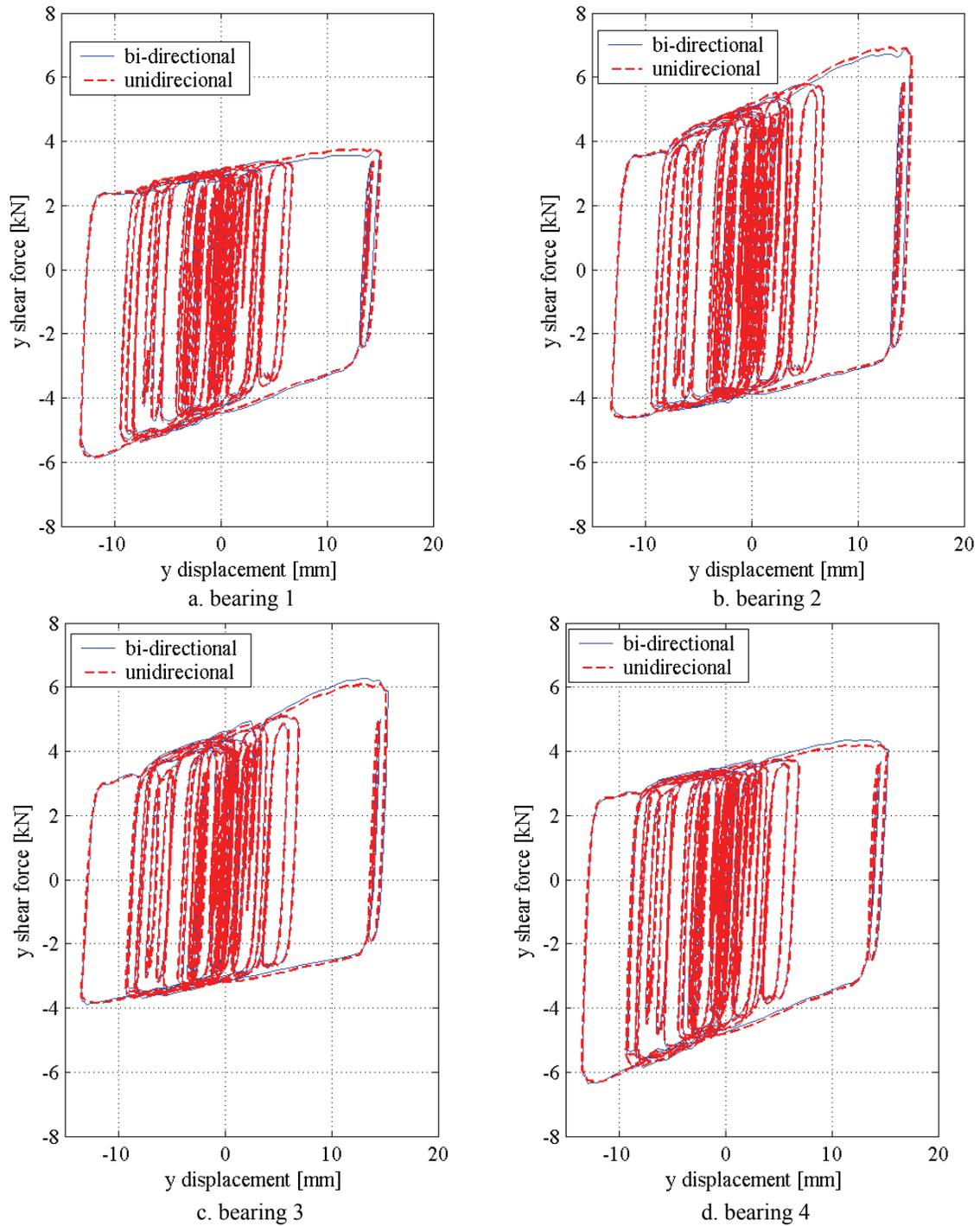
**Figure 7-14 Numerical response of the XY-FP bearings in the y-direction for 45% Tabas earthquake, inputs from tests T45%xy and T45%y**
