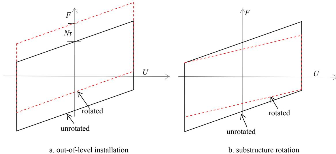
**Figure 5-6 Force-displacement loops of rotated FP bearings**
