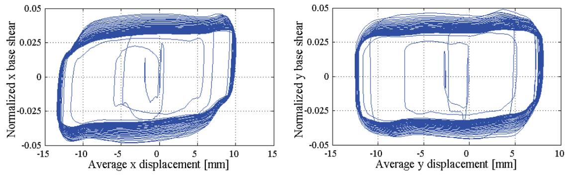
d. Global force-displacement loops for test C1xy (excitation frequency:  $x=1.6$  Hz and  $y=1.6$  Hz)
