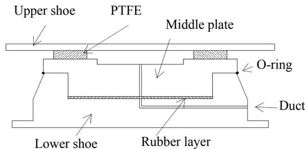
Figure 2-6 FS bearing (Ogawa et al., 1998)
