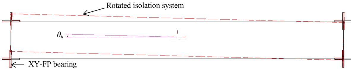
a. Plan view of an XY-FP isolated system translated and rotated
