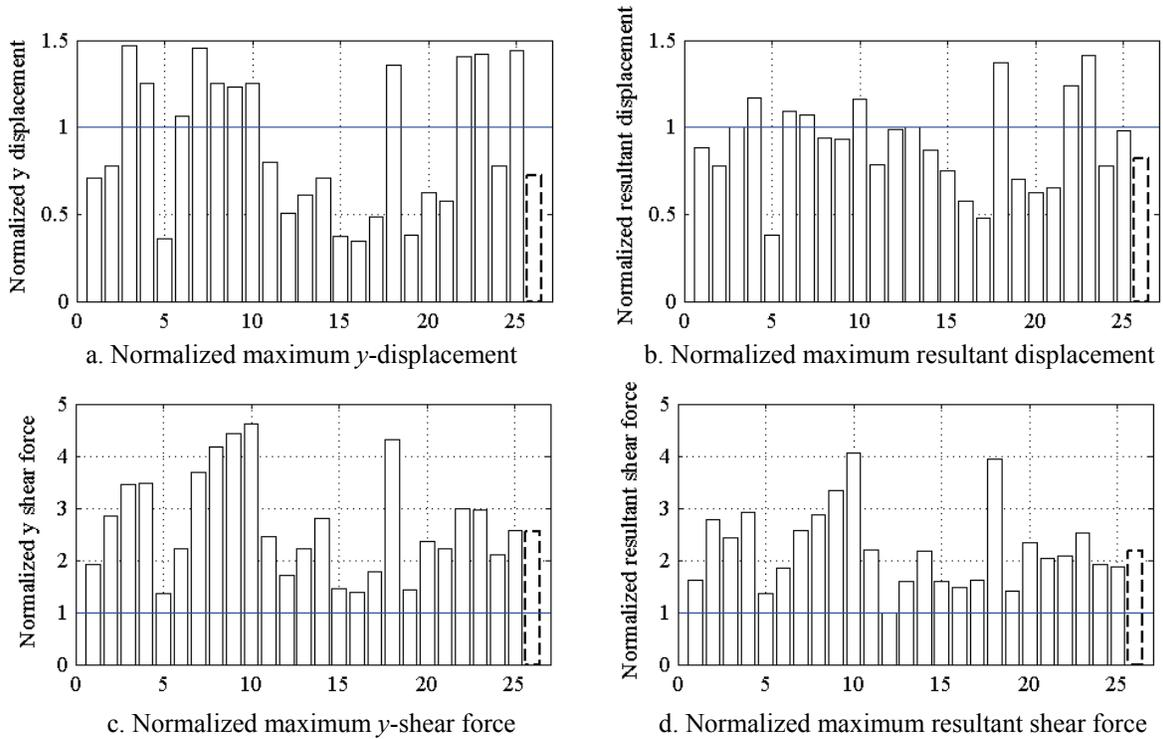
**Figure 8-22** Maximum response of the orthotropic configuration O2 normalized by the maximum response of the isotropic configuration I1 (O2/I1) and friction property FB for the near-field set of ground motions
