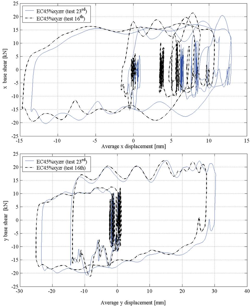
**Figure 6-40 Global responses of the XY-FP isolation system under the benchmark earthquake tests, tests EC45%xyzrr and EC45%xyzr**
