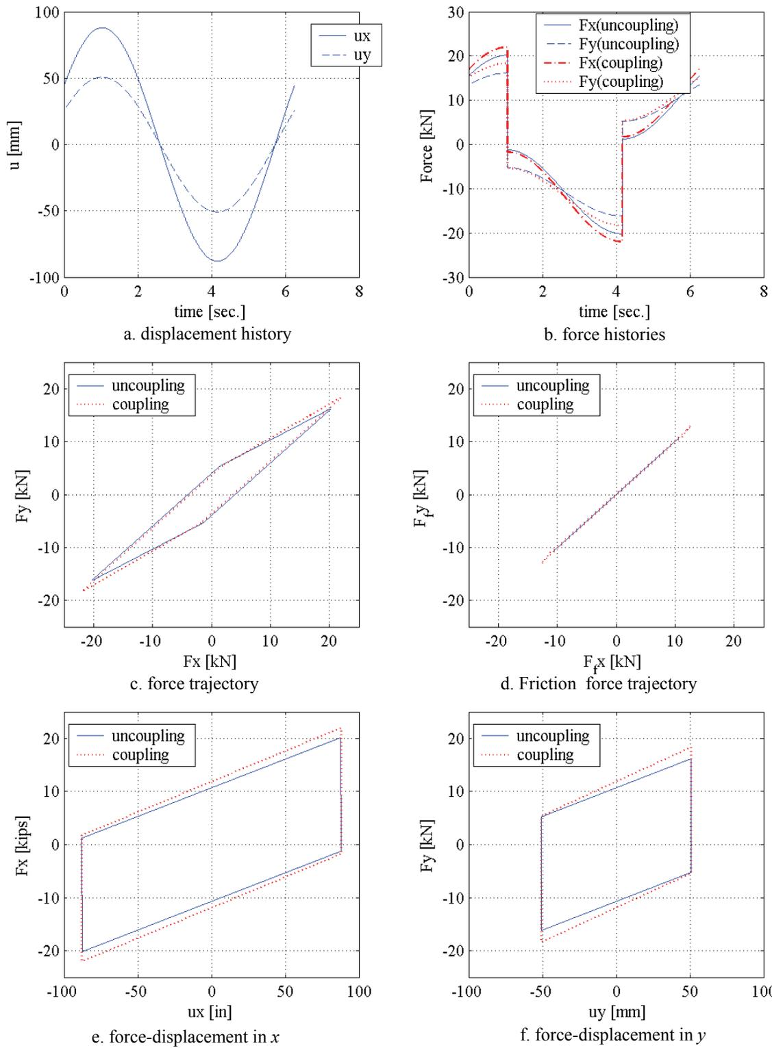
**Figure 3-25** Uncoupling and coupling of shear and friction forces in unidirectional motion oriented 30° to the x-axis
