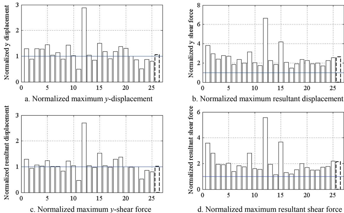
**Figure 8-25** Maximum response of the orthotropic configuration O2 normalized by the maximum response of the isotropic configuration I1 (O2/I1) and friction property FB for the far-field set of ground motions
