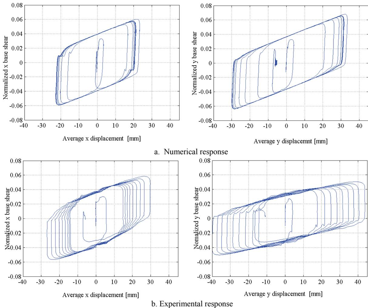
**Figure 7-1 Global force-displacement loop of the XY-FP isolation system for bi-directional excitation in test L451xy**
