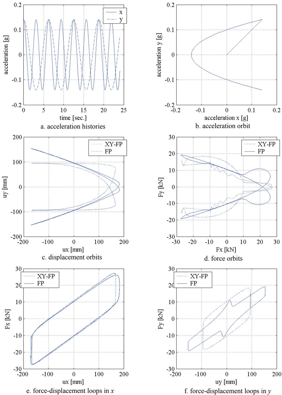
**Figure 3-31 Steady-state response to the C-shaped acceleration orbit**
