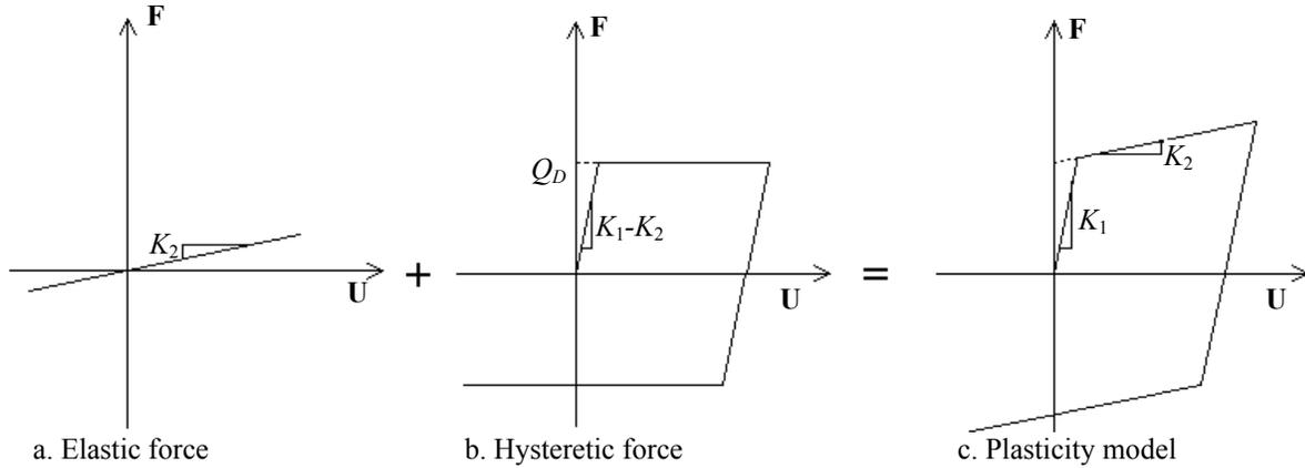
**Figure 3-7 Plasticity model components (Mosqueda et al., 2004)**
