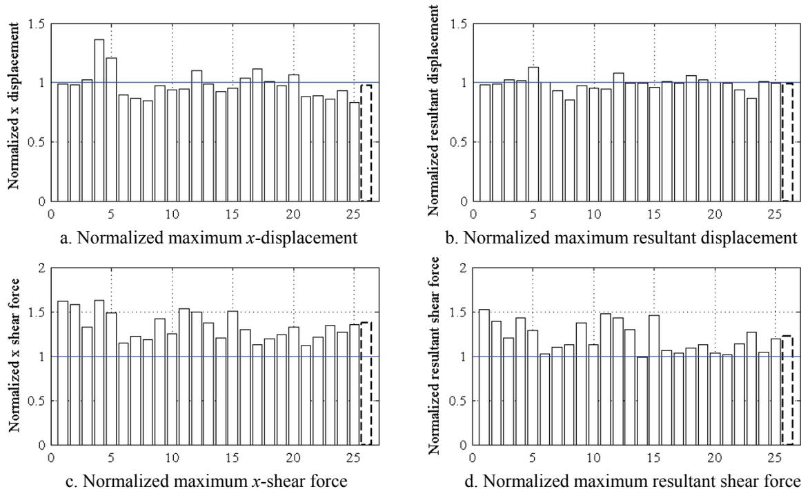
**Figure 8-18** Maximum response of the orthotropic configuration O5 normalized by the maximum response of the isotropic configuration I2 (O5/I2) and friction property FA for the far-field set of ground motions
