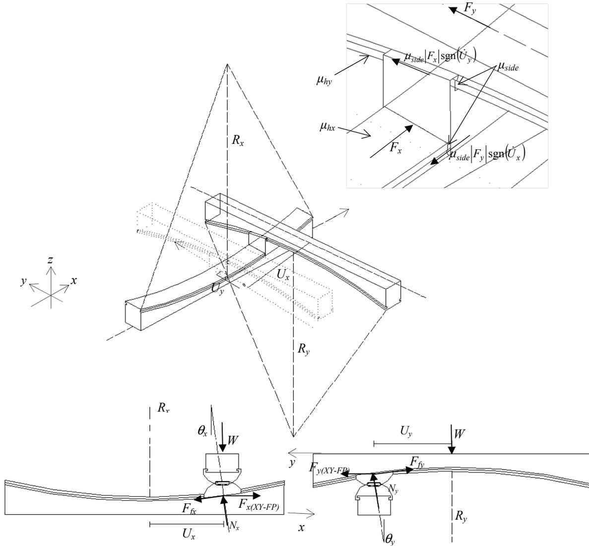
**Figure 3-8 Isometric view (original and displaced position) and free body diagrams of the rails of the XY-FP bearing in compression**
