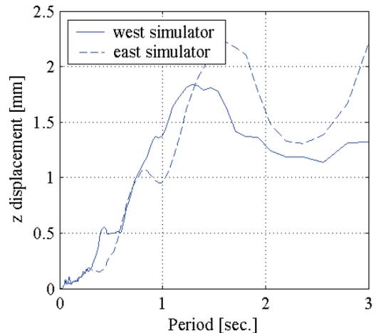
f. displacement response spectra in the  $z$ -direction
