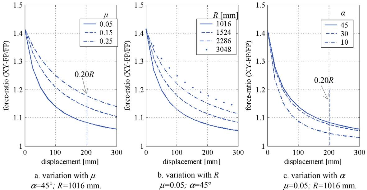
**Figure 3-15 Force ratio variation in unidirectional motion**
