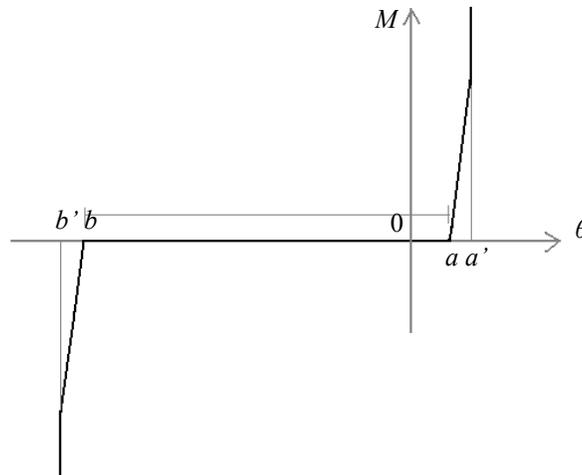
**Figure 5-12 Moment-rotation diagram of an XY-FP bearing after relocation of the center of rotation**
