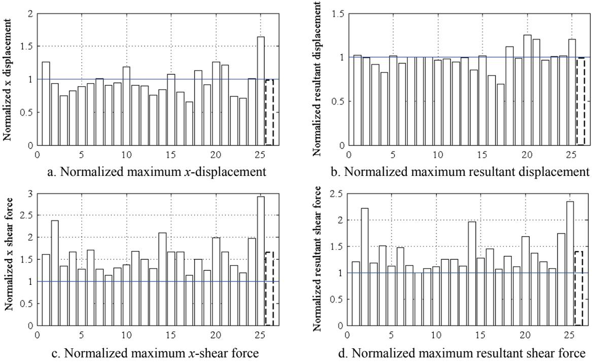
**Figure 8-14** Maximum response of the orthotropic configuration O1 normalized by the maximum response of the isotropic configuration I1 (O1/I1) and friction property FA for the far-field set of ground motions
