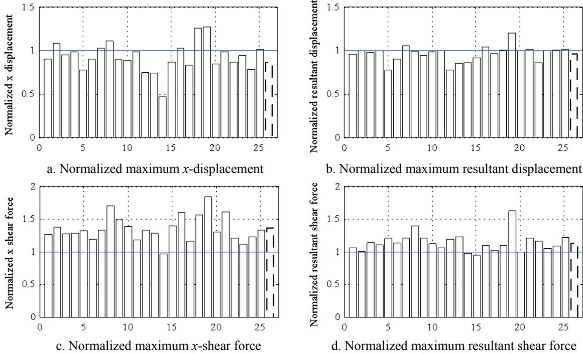
**Figure 8-9** Maximum response of the orthotropic configuration O3 normalized by the maximum response of the isotropic configuration I1 (O3/I1) for the near-field set of ground motions and friction property FA
