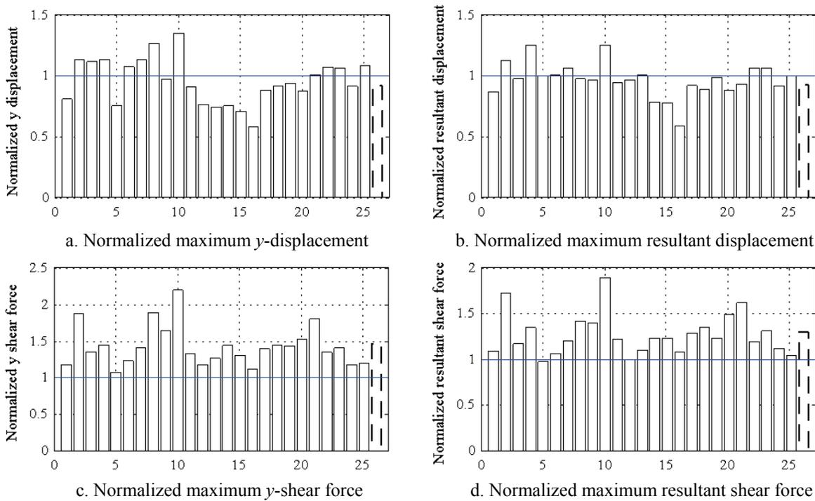
**Figure 8-10** Maximum response of the orthotropic configuration O4 normalized by the maximum response of the isotropic configuration I1 (O4/I1) for the near-field set of ground motions and friction property FA
