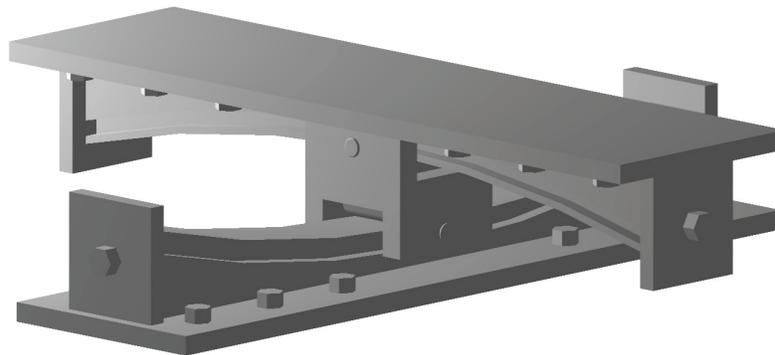
**Figure 3-3** 3D-drawing of the XY-FP bearing (Roussis, 2004)
