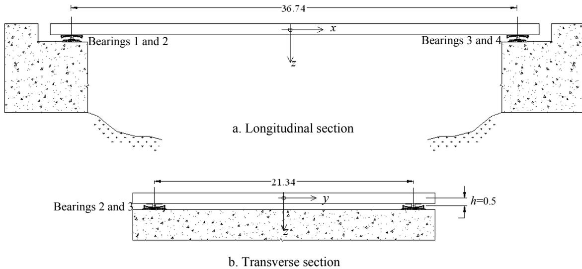
**Figure 8-4 Geometry of sample bridge (dimensions in m)**
