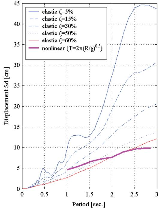
b. North-south component displacement spectra
