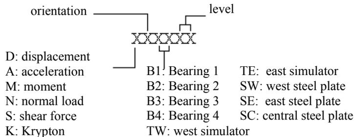
**Figure 4-8 Instrumentation notation**
