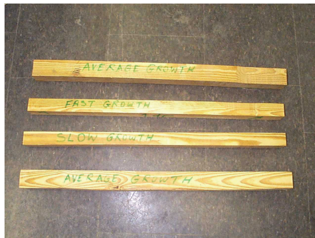
Figure 4-7. Tangential surfaces of bending specimens.
