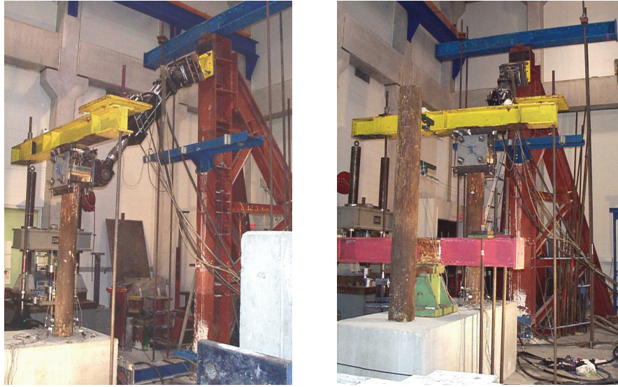
Figure 4-13. Test rig of the timber pile foundation specimens showing: (left) connection between actuator and specimen, and (right) anchor beam.
