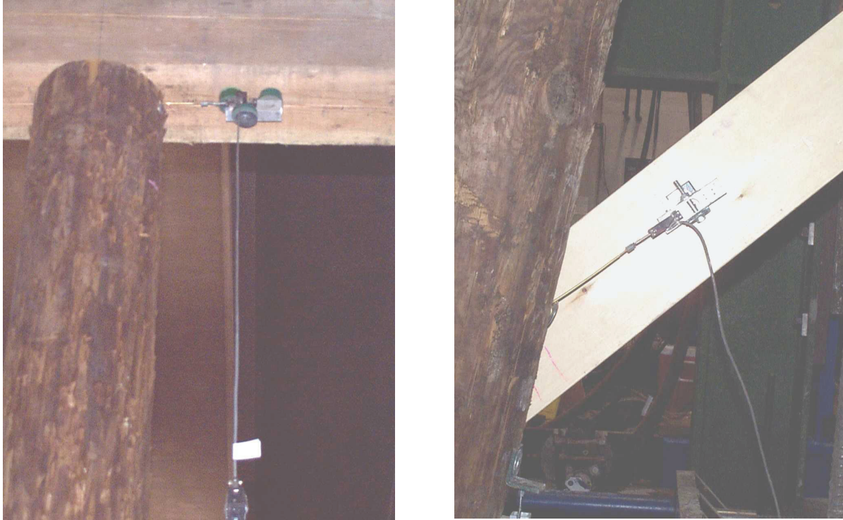
Figure 3-31. Locations of potentiometers to measure the relative displacement: between bracing and cap beam (left); and between bracing and piles (right).
