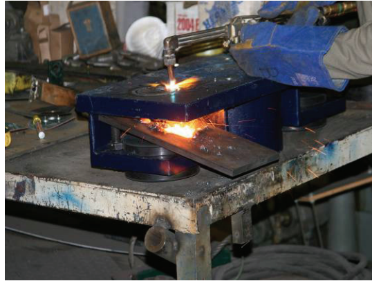
(b) Torching Holes in Base Plate
