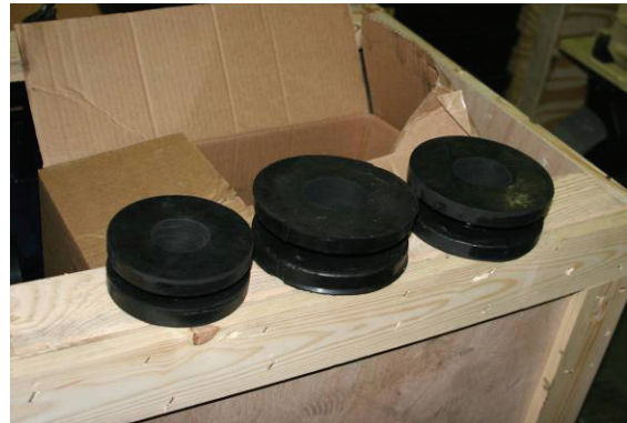
(d) Grommets Fitted in Holes of Bearings in Lower Part of Restraint Component
