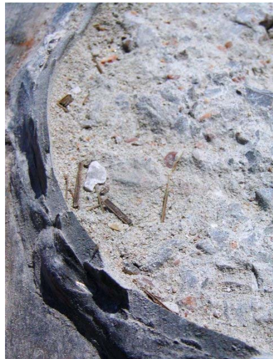
Figure 5-42 Fracture Surface of Column in Foundation (Column B2-C4, Test 7)
