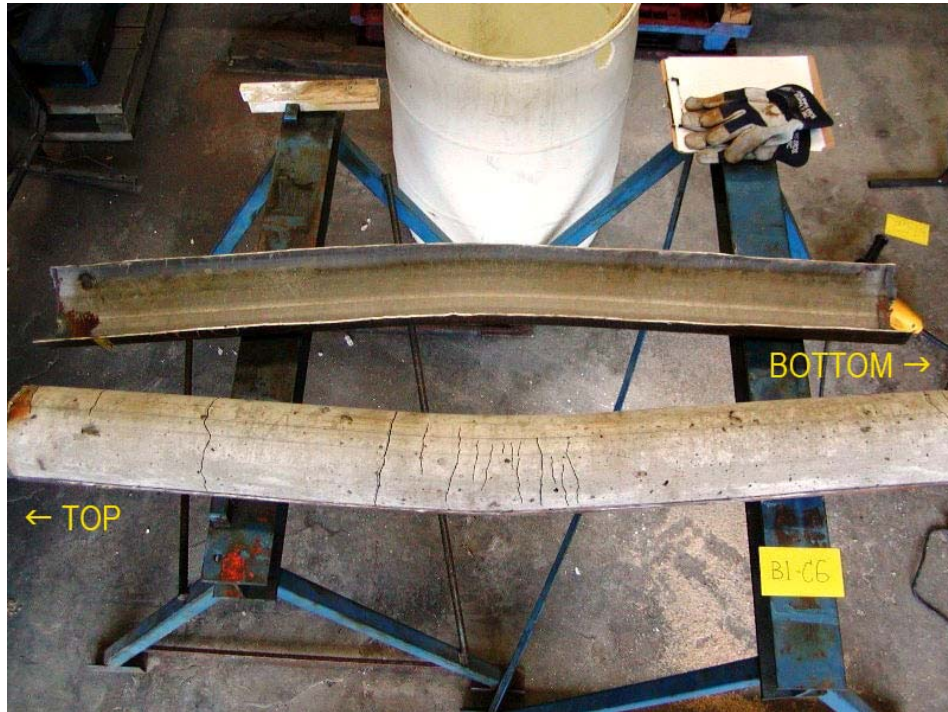
Figure 5-18 Core Concrete of Column B1-C6 after Test 4
