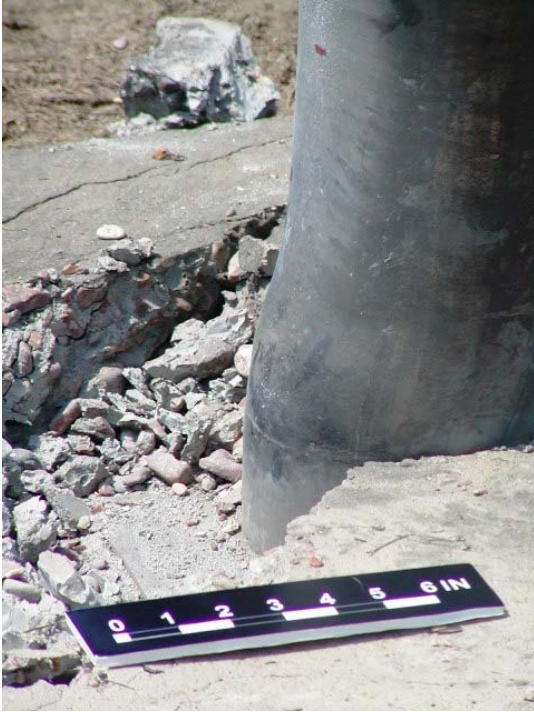
Figure 5-56 Damage at Foundation after Removal of Rubble (Column B2-C6, Test 9)
