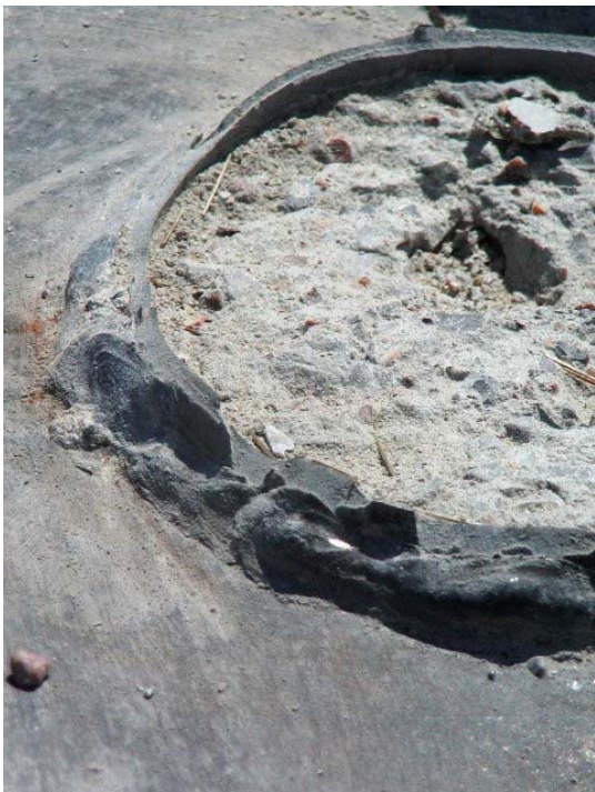
Figure 5-42 Fracture Surface of Column in Foundation (Column B2-C4, Test 7)
