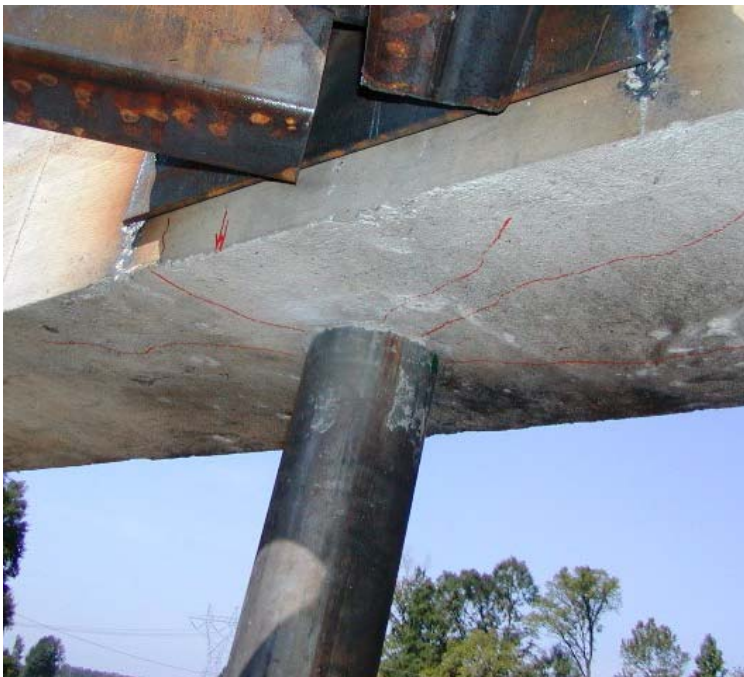
Figure 5-23 Cracking at Cap-beam of Column B1-C5 after Test 5
