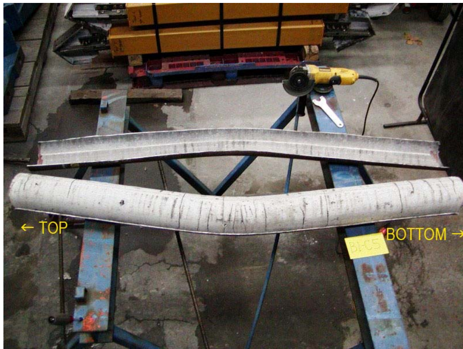
Figure 5-26 Core Concrete of Column B1-C5 after Test 5
