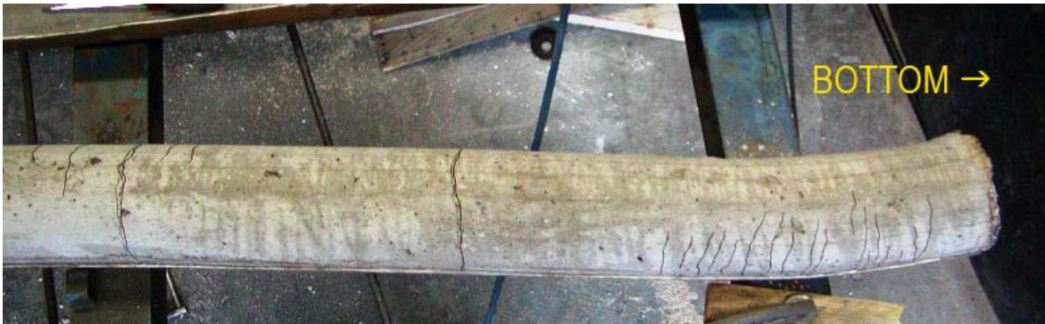
Figure 5-56 Damage at Foundation after Removal of Rubble (Column B2-C6, Test 9)
