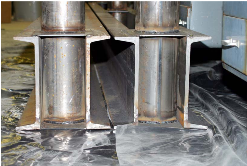
Figure 4-15 Column-to-cap Beam Connection
