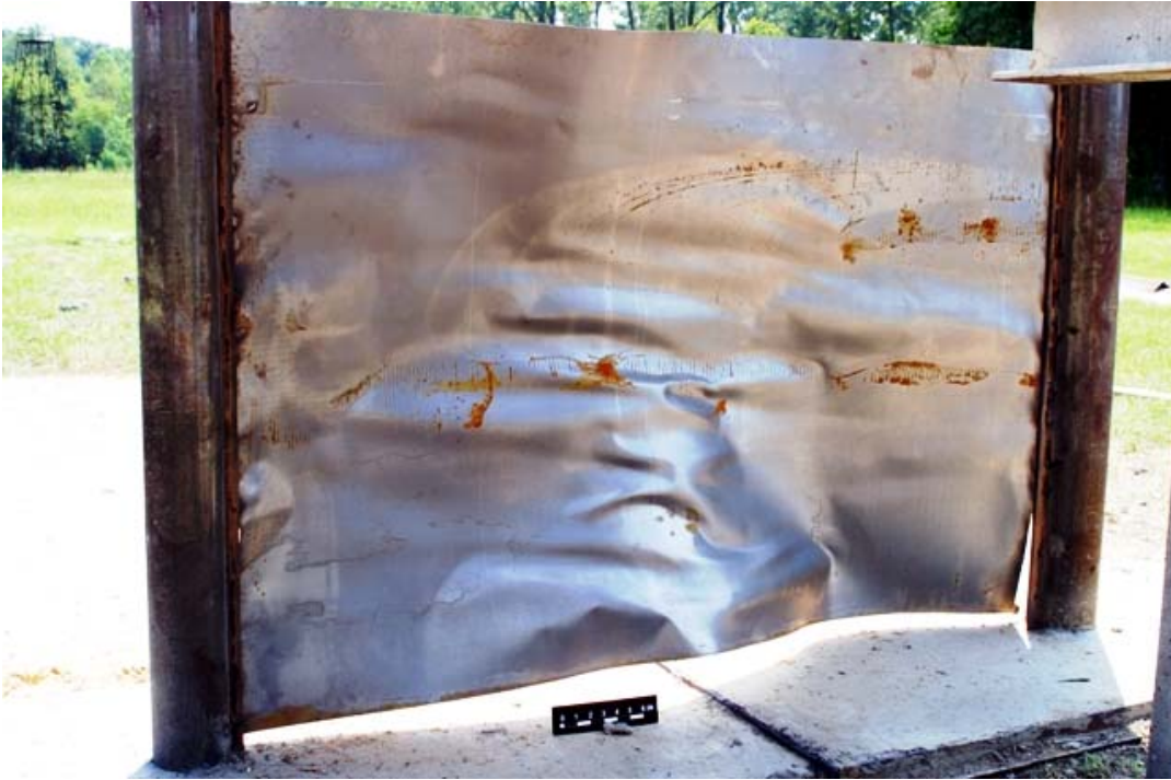
Figure 5-48 Deformation of Plate B2-SP56 after Test 8 (Back Face)
