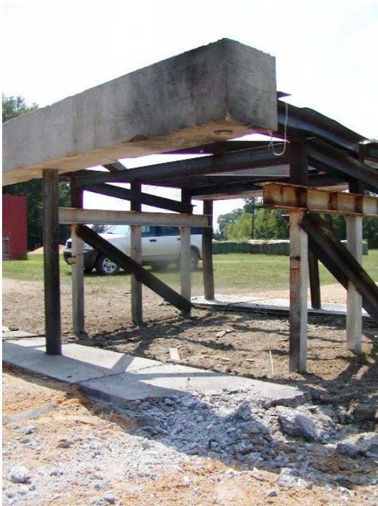
Figure 5-32 Disappearance of Column B2-C4 after Test 7
