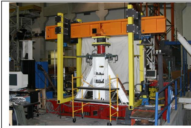
Figure 2. Small bearing testing machine
