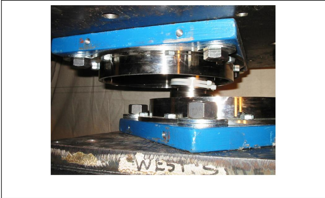
Figure 4. Photograph of the bearing at maximum displacement
