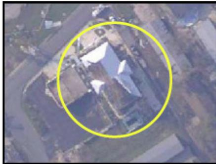
*Figure 4-14. Aerial photo reveals wind-pressure damage to the roof cladding, and low-density debris nearby. This portion of Bay St. Louis was not affected by storm surge.*
