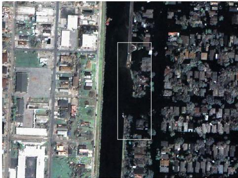
Levee breach at the 17<sup>th</sup> Street Canal near the Hammond Highway bridge. The non-flooded area on the west side of the canal is Jefferson Parish, and the flooded area on the east side is Orleans Parish. This image shows the dramatic difference between flood and no-flood areas.
