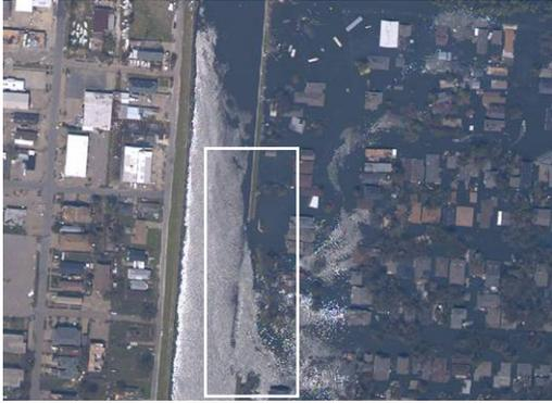
NOAA aerial image of levee breach at the 17<sup>th</sup> Street Canal near the Hammond Highway bridge.
