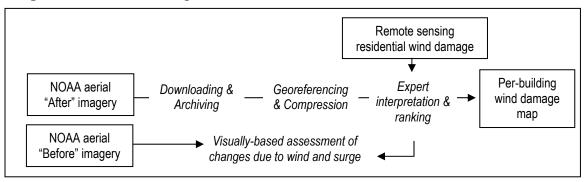
Figure 4-11. Methodology employed for per-building wind damage detection.
