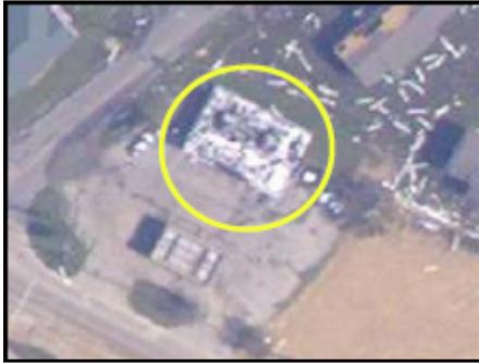
*Figure 4-16. Aerial photo reveals wind-pressure damage to the roof cladding, and low-density debris nearby. This portion of Waveland was not affected by storm surge.*
