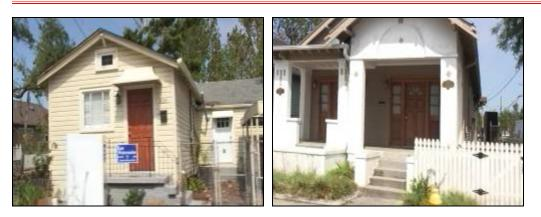
*Figure 5-14. Examples of buildings classified in the WF-1 ("Minor Damage") category in an area of no flooding.*
