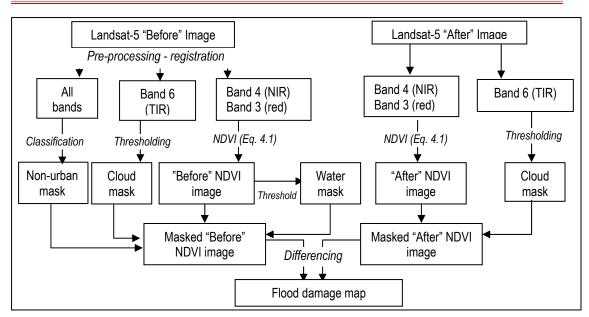
Figure 4-24. Methodology employed for region-wide flood damage detection.
