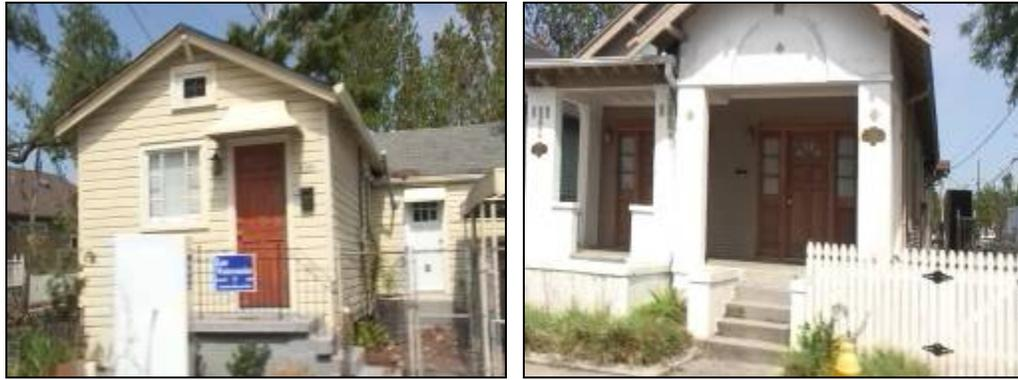
*Figure 5-14. Examples of buildings classified in the WF-1 (“Minor Damage”) category in an area of no flooding.*
