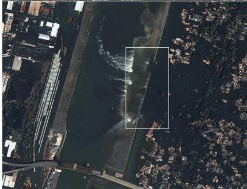
Levee breach located on the east side of the Industrial Canal between Florida Avenue and North Claiborne Avenue, causing flooding in the Lower Ninth Ward. The destruction of buildings in this area of high-velocity flooding is evident from the scattering of the building roofs.
