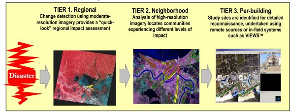
*Figure 3-2. Tiered reconnaissance system, using remote sensing to identify impacted areas for multi-hazard reconnaissance planning and damage assessment.*
