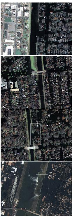
Levee breach at the 17<sup>th</sup> Street Canal near the Hammond Highway bridge. The non-flooded area on the west side of the canal is Jefferson Parish, and the flooded area on the east side is Orleans Parish. This image shows the dramatic difference between flood and no-flood areas.
