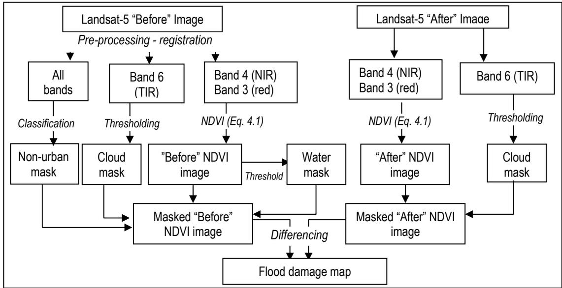
Figure 4-24. Methodology employed for region-wide flood damage detection.
