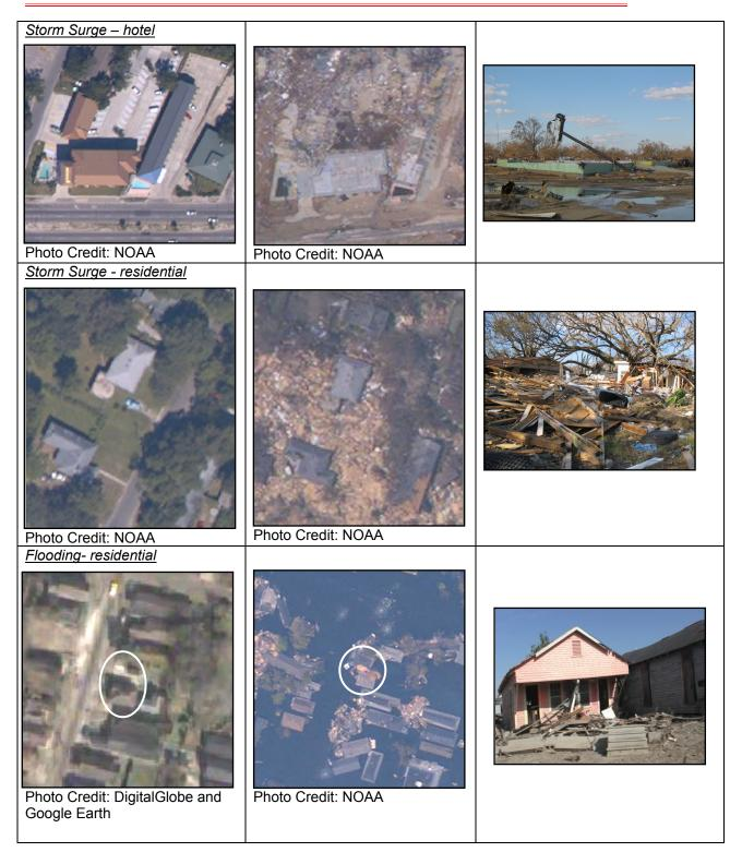
*Figure 6-7 (continued). Examples of pre-storm and post-storm remote sensing imagery with corresponding ground-truthing images.*
