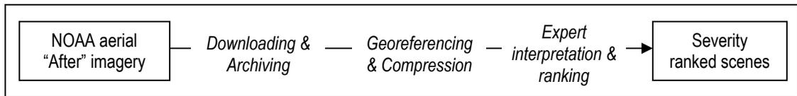
Figure 4-9. Methodology employed for neighborhood-scale wind damage detection.
