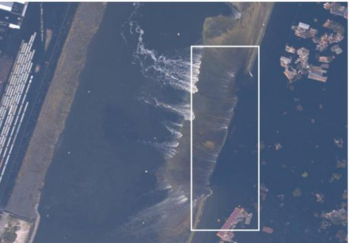
NOAA aerial image of levee breach located on the east side of the Industrial canal between Florida Avenue and North Claiborne Avenue, causing flooding in the Lower Ninth Ward.
