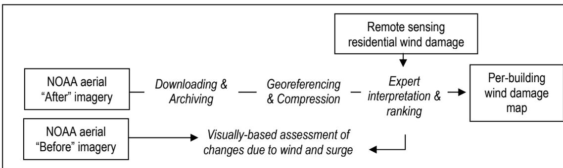
Figure 4-11. Methodology employed for per-building wind damage detection.
