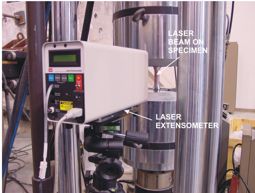
Figure 2-2: Photograph of Laser Extensometer Measuring Coupon Deformation
