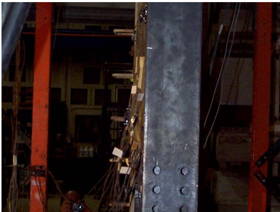
(b) After Buckling of the Inner PMC Sandwich Panel
