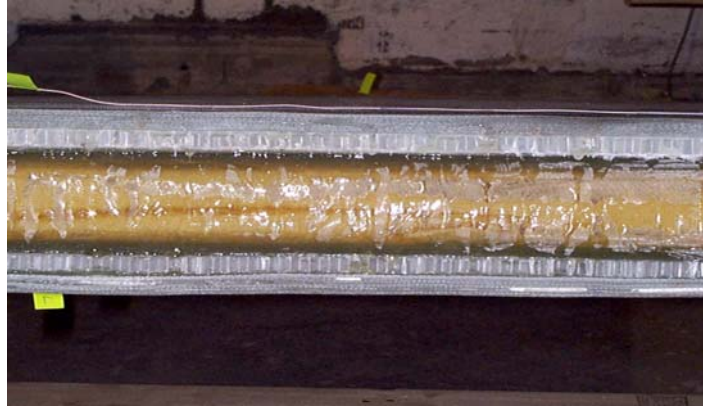
(a) Cross Section of the PMC Sandwich Panel
