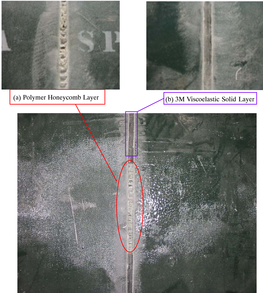
(c) Combining Polymer Honeycomb and 3M Viscoelastic Materials
