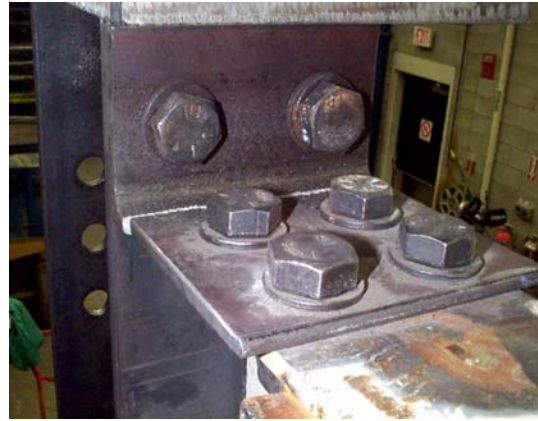
(a) Angle connection failure at top and bottom joints
