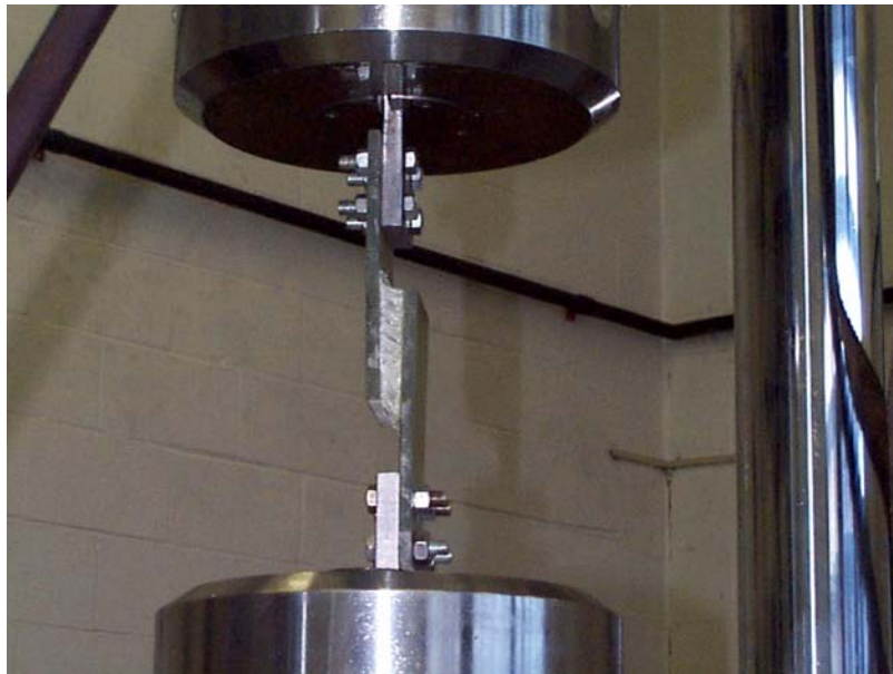
Figure 2-30 The Large Deform Shape of Polymer Honeycomb Material ( \epsilon = 0.79 in/in )
