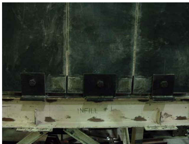
(c) Setup Outer Damping Panel to the Tested Frame by weld
