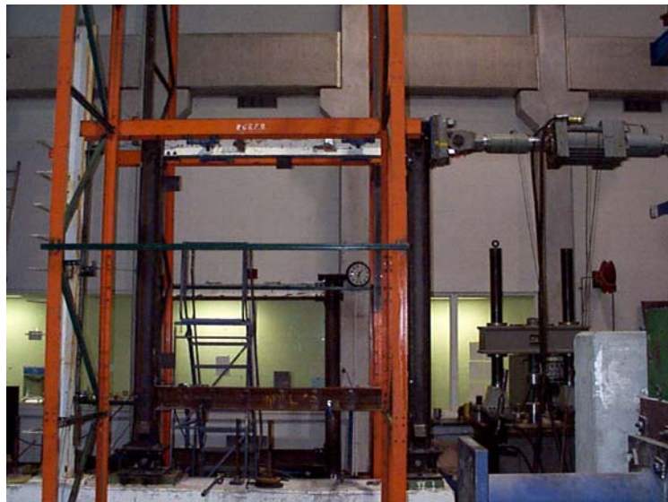
Figure 3-4 Steel Frame Setup
