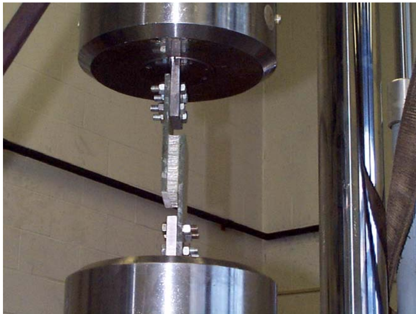
Figure 2-28 Setup of Polymer Honeycomb Test Coupon
