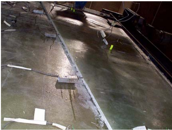
(c) Deformation of Viscoelastic Layers
