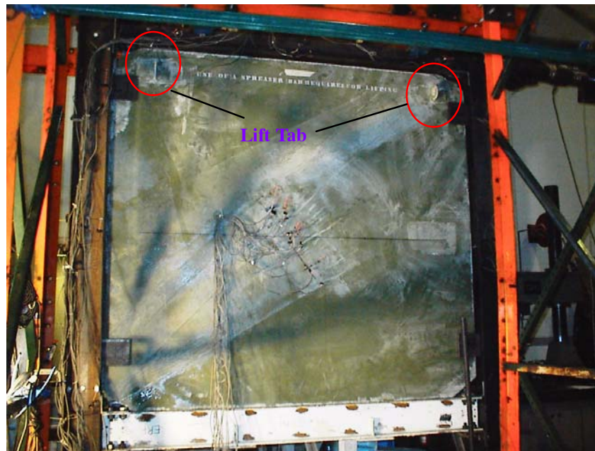
Figure 6-13 Fabrication of the PMC Sandwich Infill Panel
