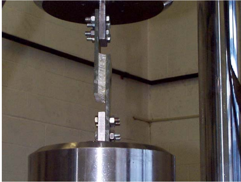
Figure 2-29 The Small Deform Shape of Polymer Honeycomb Material ( \epsilon = 0.28 in/in )
