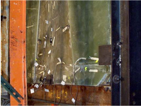
(a) Elastic Buckling of Inner Panel
