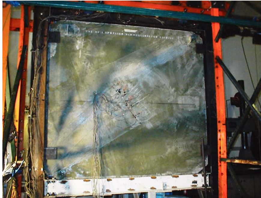
Figure 6-32 PMC Sandwich Infill Setup
