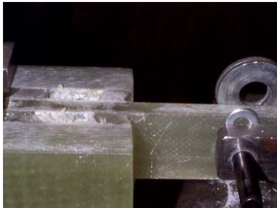
(c) Bonding Failure of the Honeycomb
