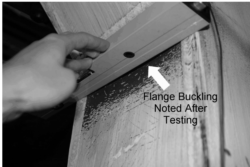
FIGURE 5-27 Magnitude of Flange Buckling After Testing of Specimen X1L2.1 Relative to a Straight Edge
