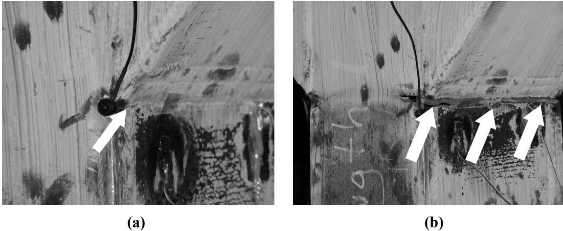
FIGURE 5-3 Flange Fracture of Specimen X1L1.2 During: (a) Sequence 14; and (b) Sequence 15
