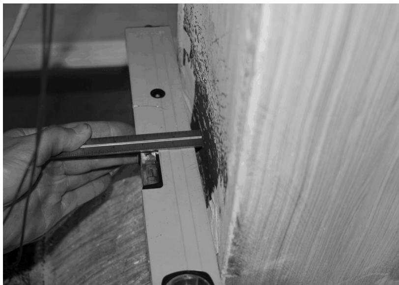
FIGURE 5-41 Buckling Magnitude of Bottom East Flange of Specimen X1L3.9 Relative to a Straight Edge After Testing
