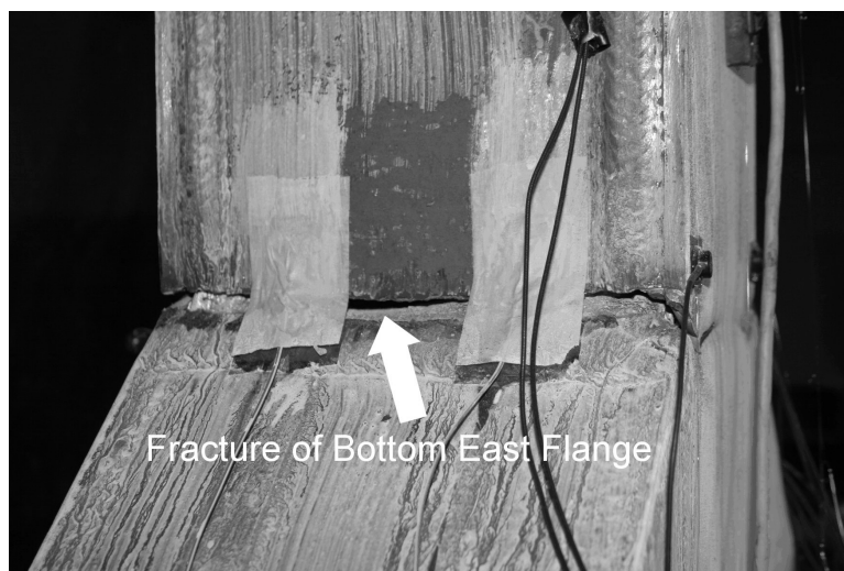
FIGURE 5-37 Fracture of the Bottom East Flange of Specimen X3L2.1 After Testing
