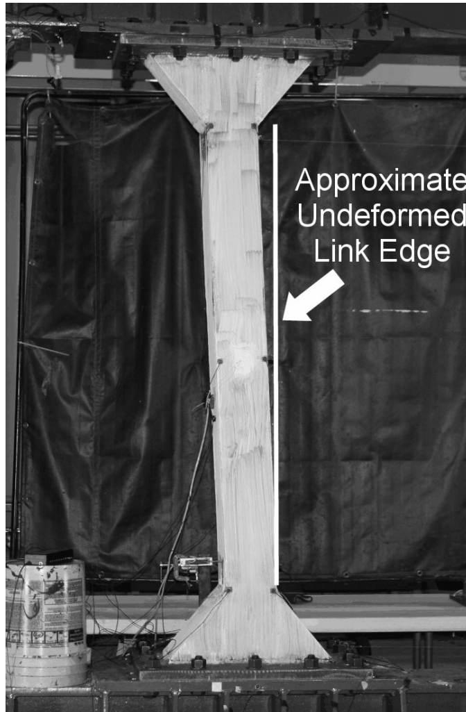
FIGURE 5-50 Specimen X3L3.0 at -0.059 rads During Cycle 2 of Sequence 8
