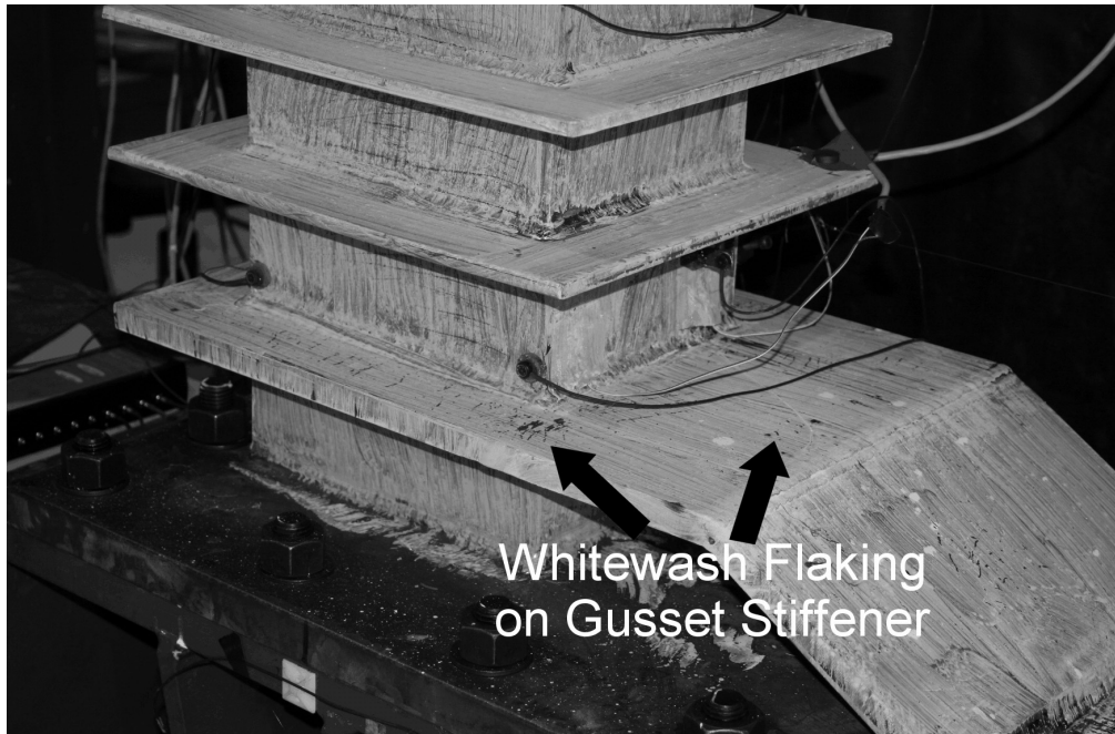
FIGURE 5-61 Whitewash Flaking on End Connection of AX2L1.6 After Sequence 5
