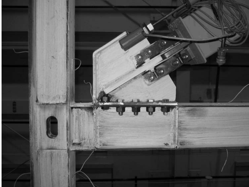
Figure 3.11. Gusset-Plate for Nippon Steel BRBs
