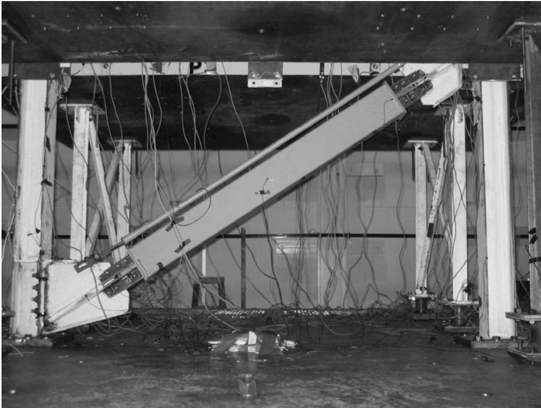
Figure 3.8. Nippon Steel BRB in Place
