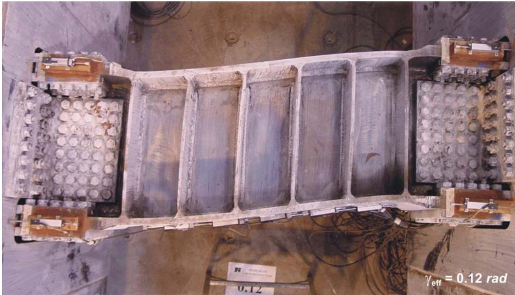
**Figure 3-6: Deformed Link H485**
