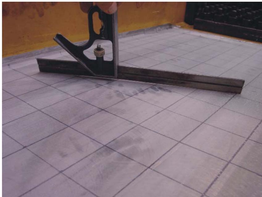
**Figure 4-37: Web Distortion in Link X100 at End of Second Set**
