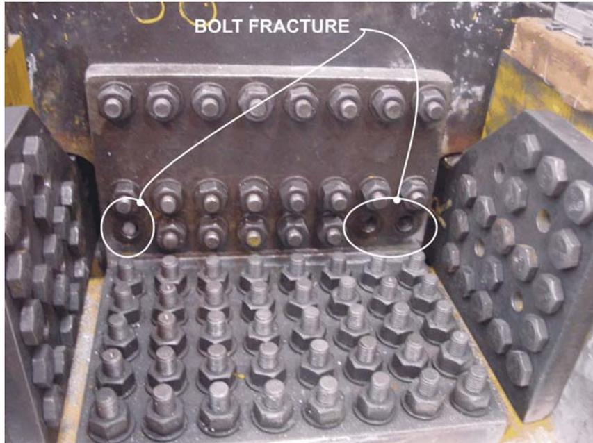
**Figure 4-9: Bolt Fracture in Connection Zone of Link L100**
