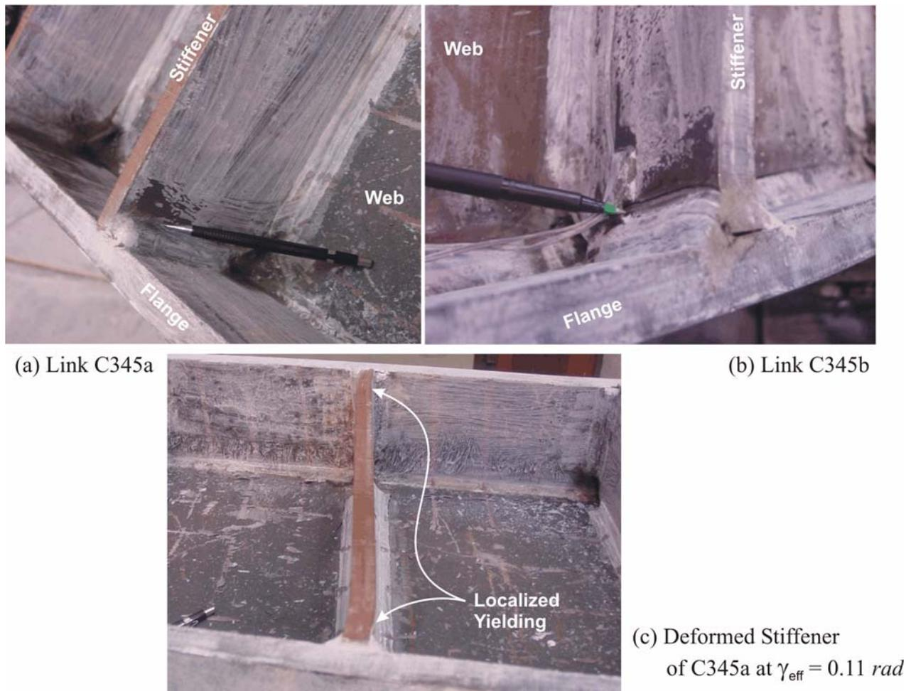
**Figure 2-12: Stiffener Cracking at Flange Fillet Welds**
