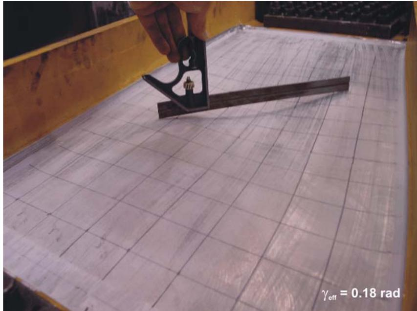
**Figure 4-19: Web Out of Plane Web Deformation in Link X100**
