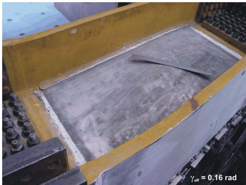
**Figure 4-14: Web Out of Plane Web Deformation of Link L225**
