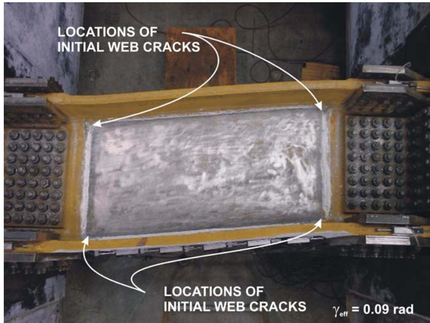
**Figure 4-13: Location of Initial Cracks in Link L225**
