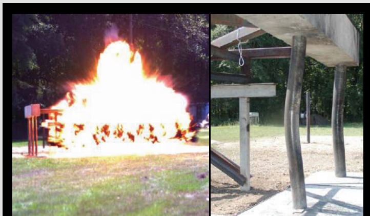
Figure 10. Blast testing of concrete-filled steel tube bridge pier concept, and resulting acceptable residual deformations.
