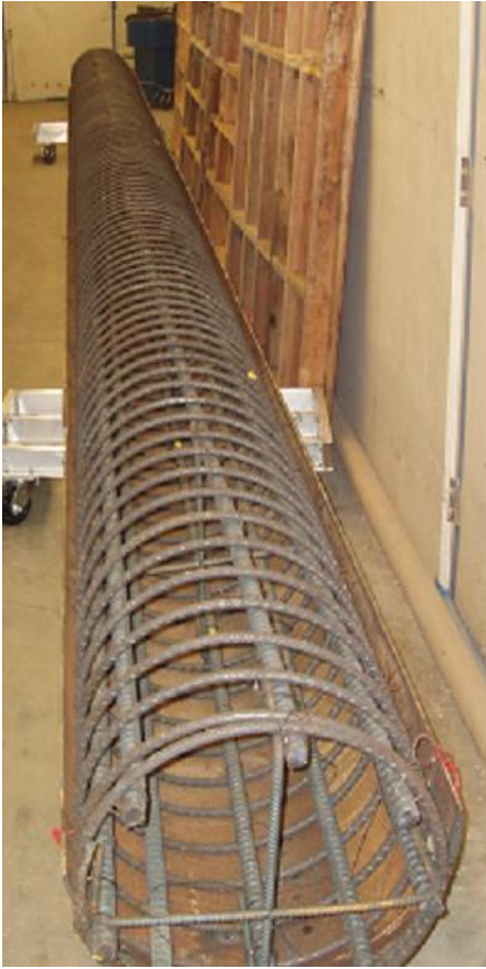
Figure 10. Empty rebar column
