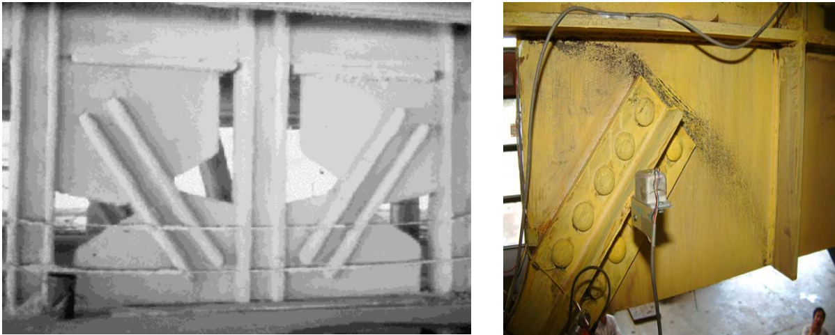
Figure 2: Oversized Gusset Plate Connections Used in SCBF
