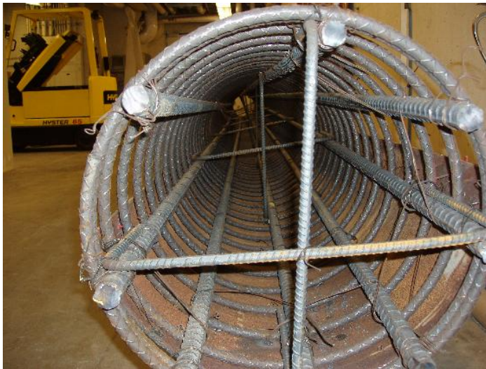
Figure 9. Empty rebar cage
