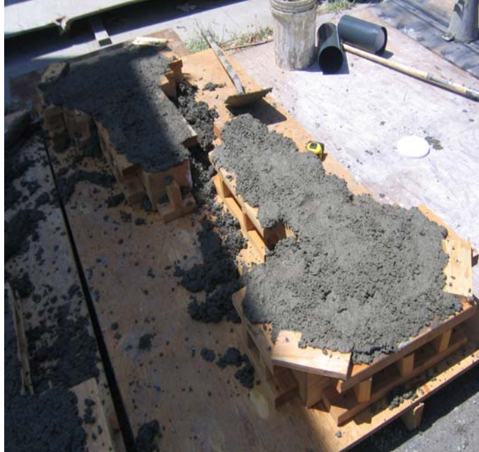
Figure 6.4: Casting of test specimens.
