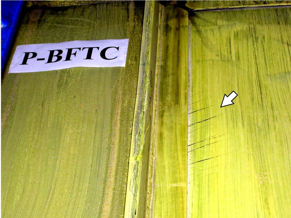
FIGURE 5-19 Panel yielding adjacent to far column fish plate (P: Cycle 19,  $\gamma = 1.5\% \approx 5\delta_y$ )
