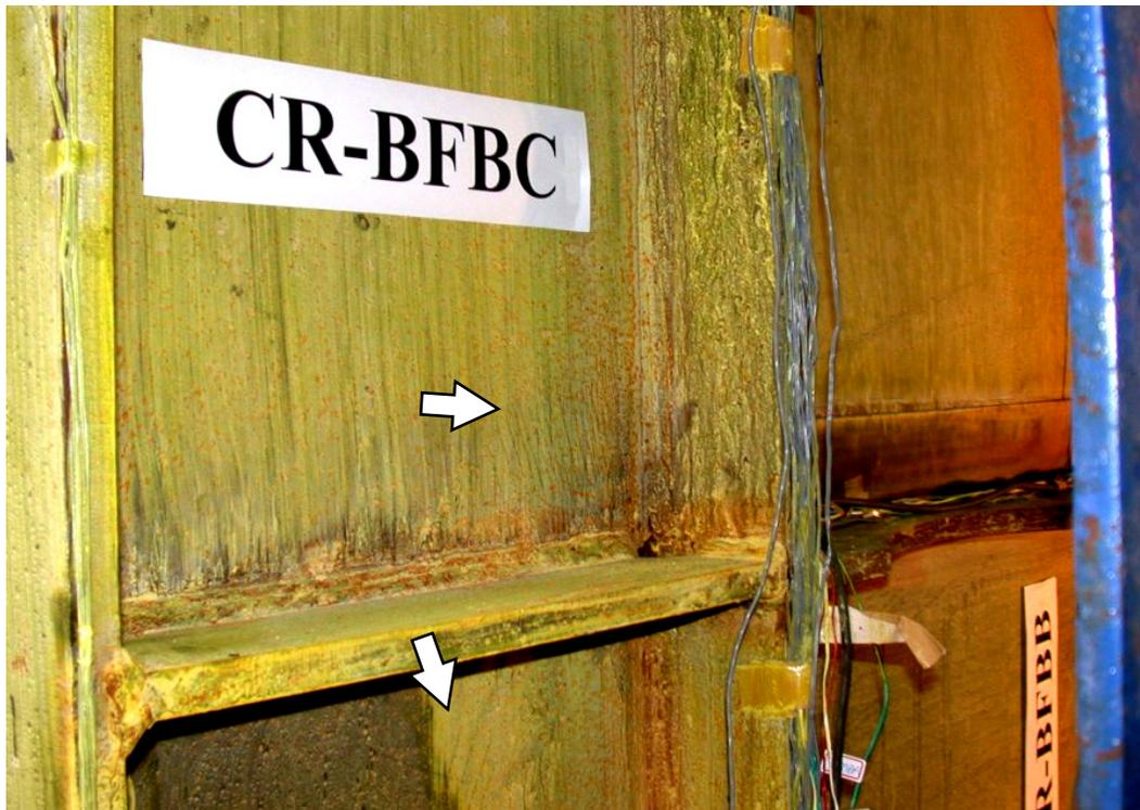
FIGURE 5-45 Web and panel zone yielding – bottom of far column
