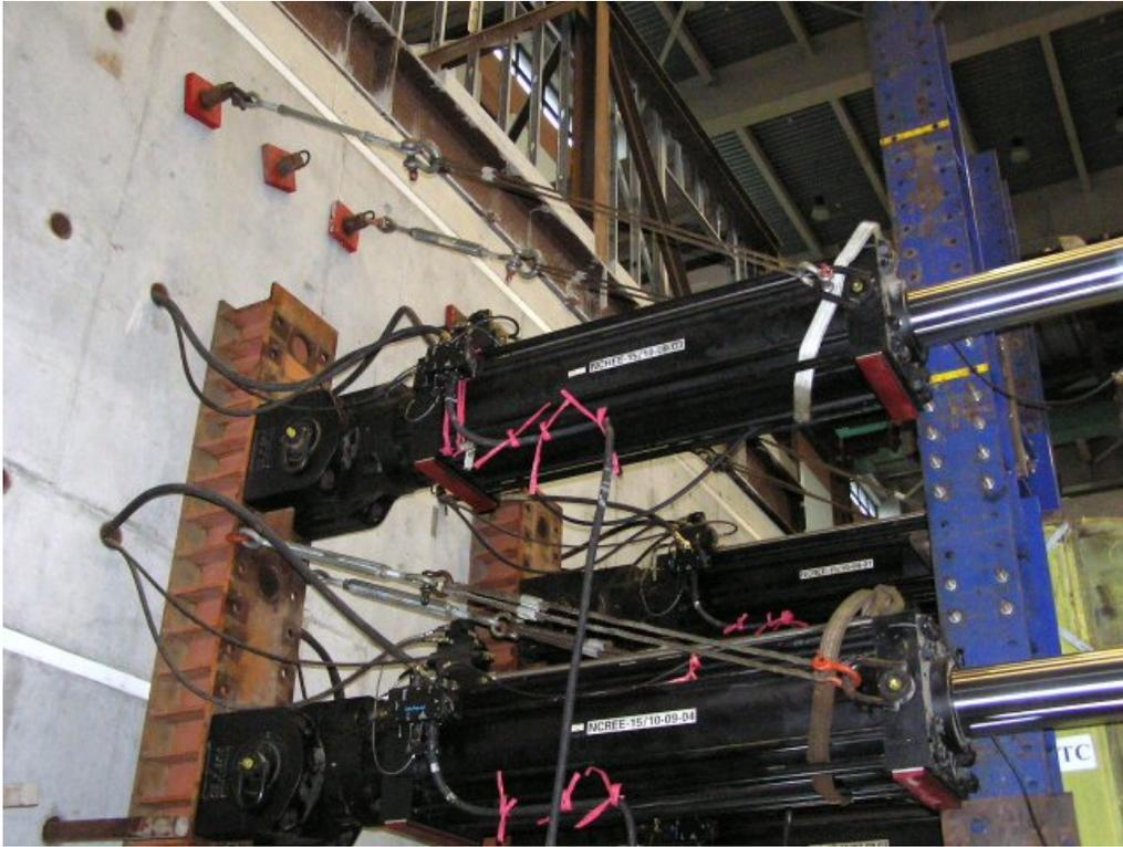
**FIGURE 5-18 Added cables supporting actuators**
