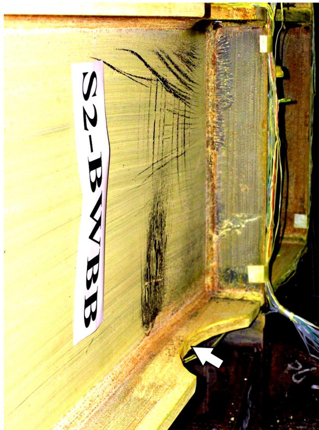
FIGURE 5-82 Wall bottom beam RBS web local buckling (S2: Cycle 17,  $\gamma = 1.2\% \approx 4\delta_y$ )
