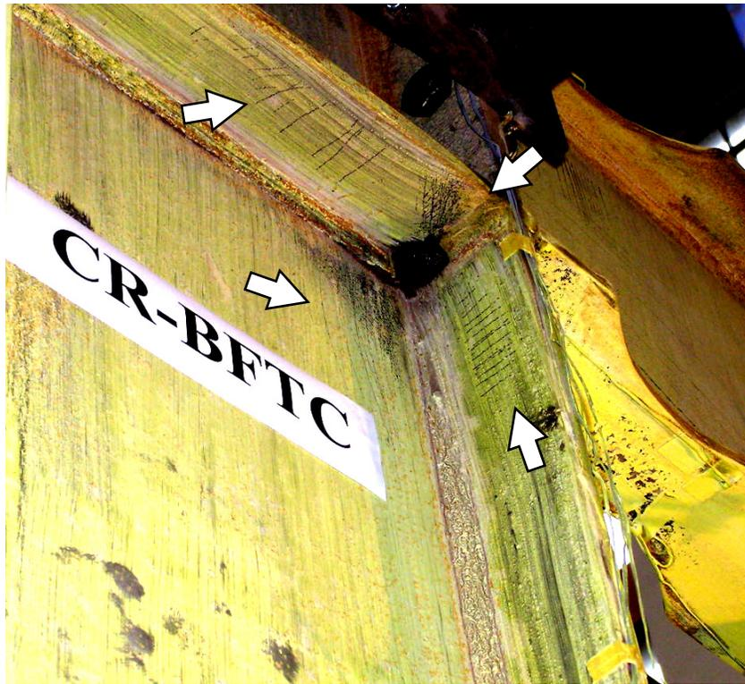
**FIGURE 5-54 Far column web and flange & top beam continuity plate yielding
