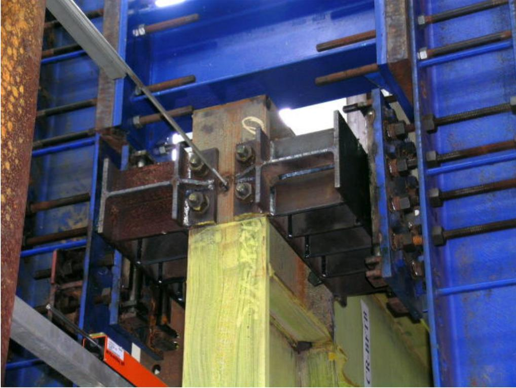
**FIGURE 5-37 New far column lateral support (CR: Pre-test)**
