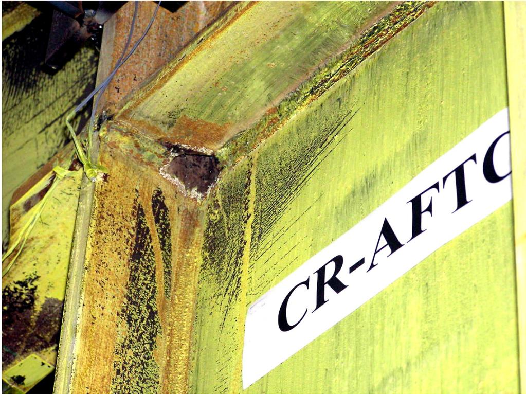
(c) Detail of web and inside of wall flange yielding from (a)
