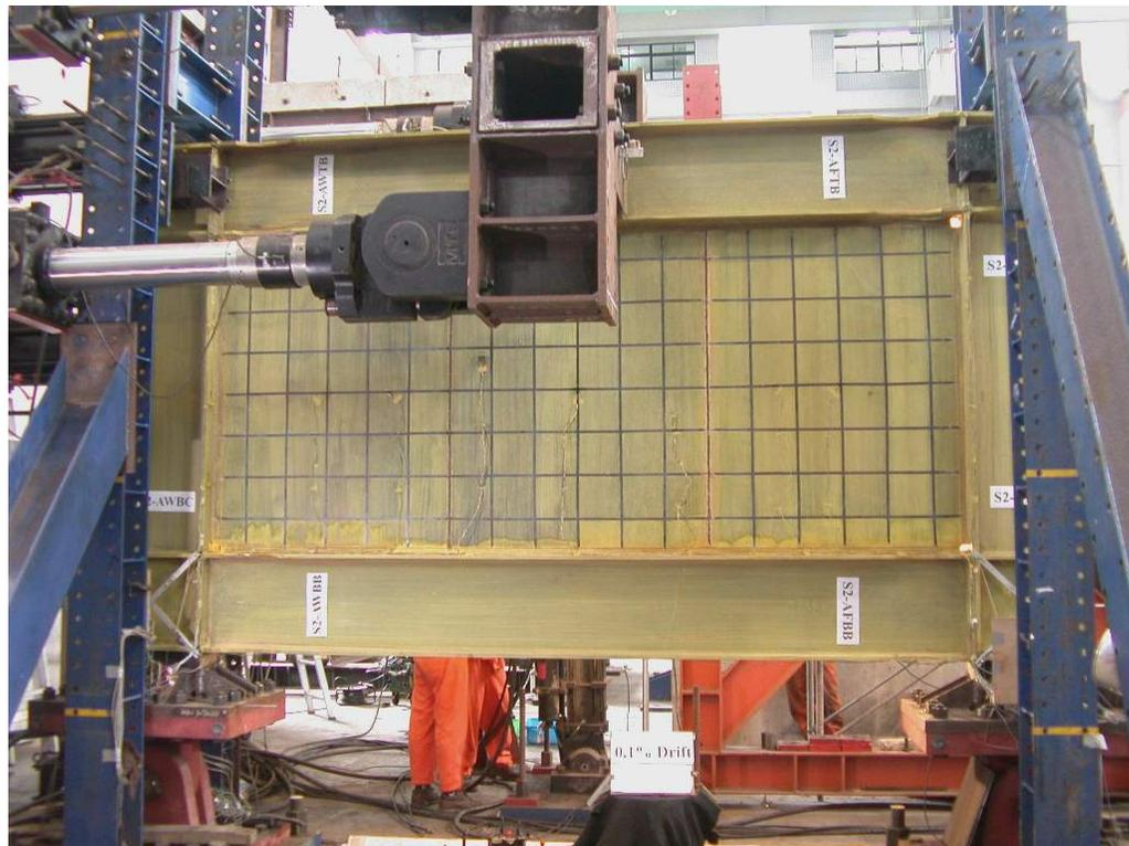
**FIGURE 4-19 Specimen S2 prior to Testing**
