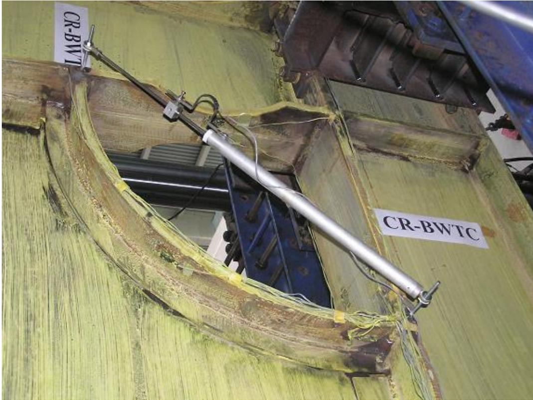
**FIGURE 4-23 “Pi” gage for Arch Deformation Measurement in Specimen CR**
