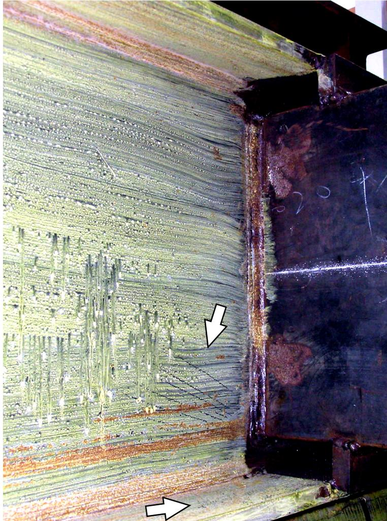
(e) A-side web and flanges adjacent to wall side of loading detail
