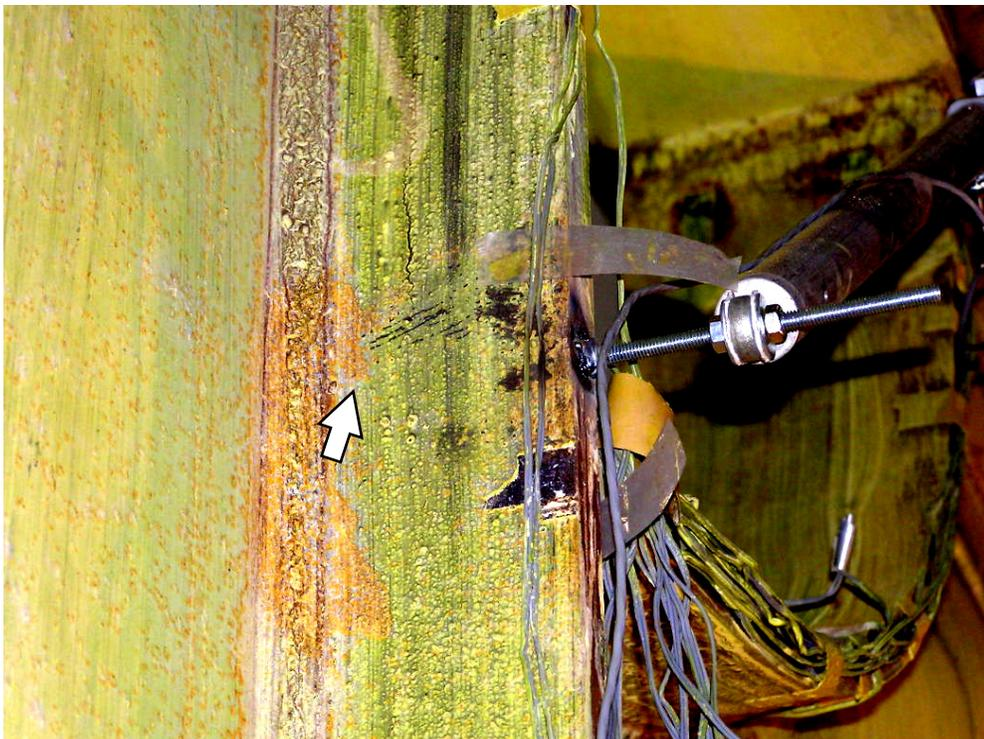
**FIGURE 5-55 Far column wall flange yielding at bottom of far arch
