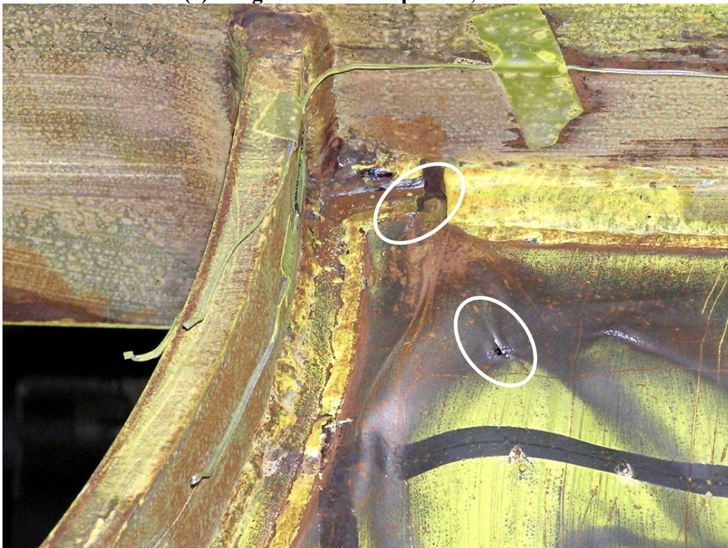
(f) Panel tears at wall arch at top beam connection and panel interior
