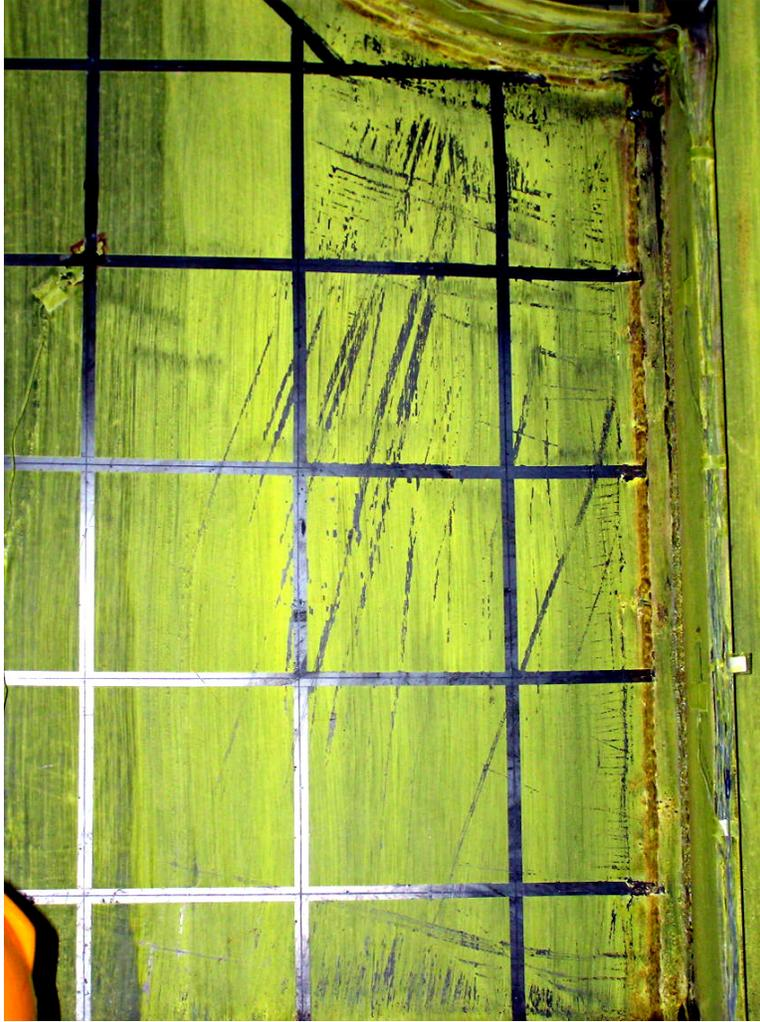
**FIGURE 5-42 panel yielding at far column (CR: Cycle 12,  $\gamma = 0.6\% \approx 2\delta_y$ )**
