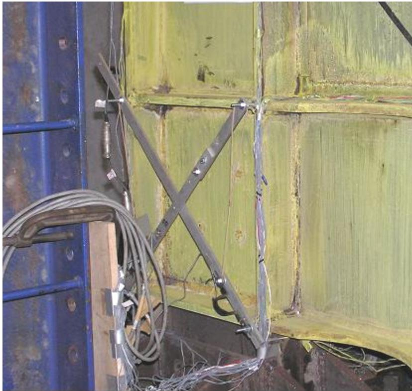
**FIGURE 4-22 “Pi” gage for Panel Zone Deformation Measurement**
