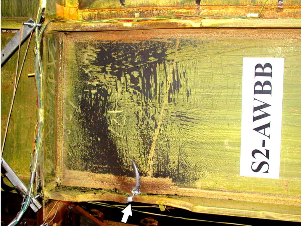
(a) Web and bottom flange rupture
