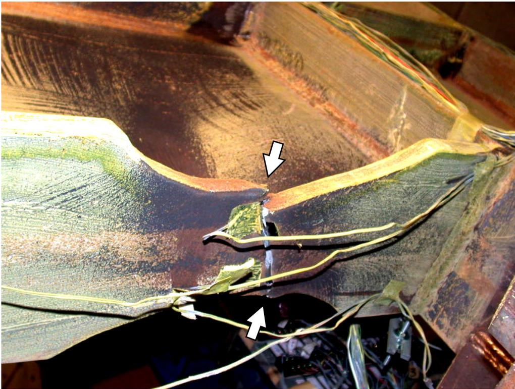
(b) Bottom flange rupture from bottom
