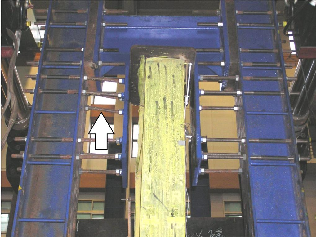
**FIGURE 5-25** Wall column rotation and damage to bolts supporting column lateral restraint (P: Cycle 22,  $\gamma = 2.5\% \approx 8.333\delta_r$ )
