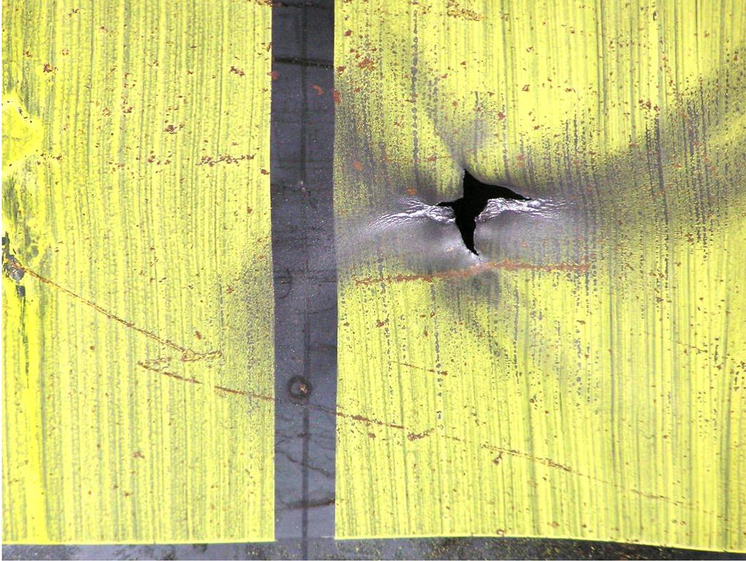
(i) Panel fatigue tear detail from (h)
