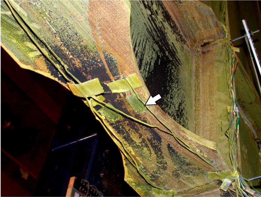
**FIGURE 5-91 Bottom beam far RBS connection yielding and bottom flange cracking (S2: Cycle 23,  $\gamma = 2.5\% \approx 8.333\delta_i$ )**
