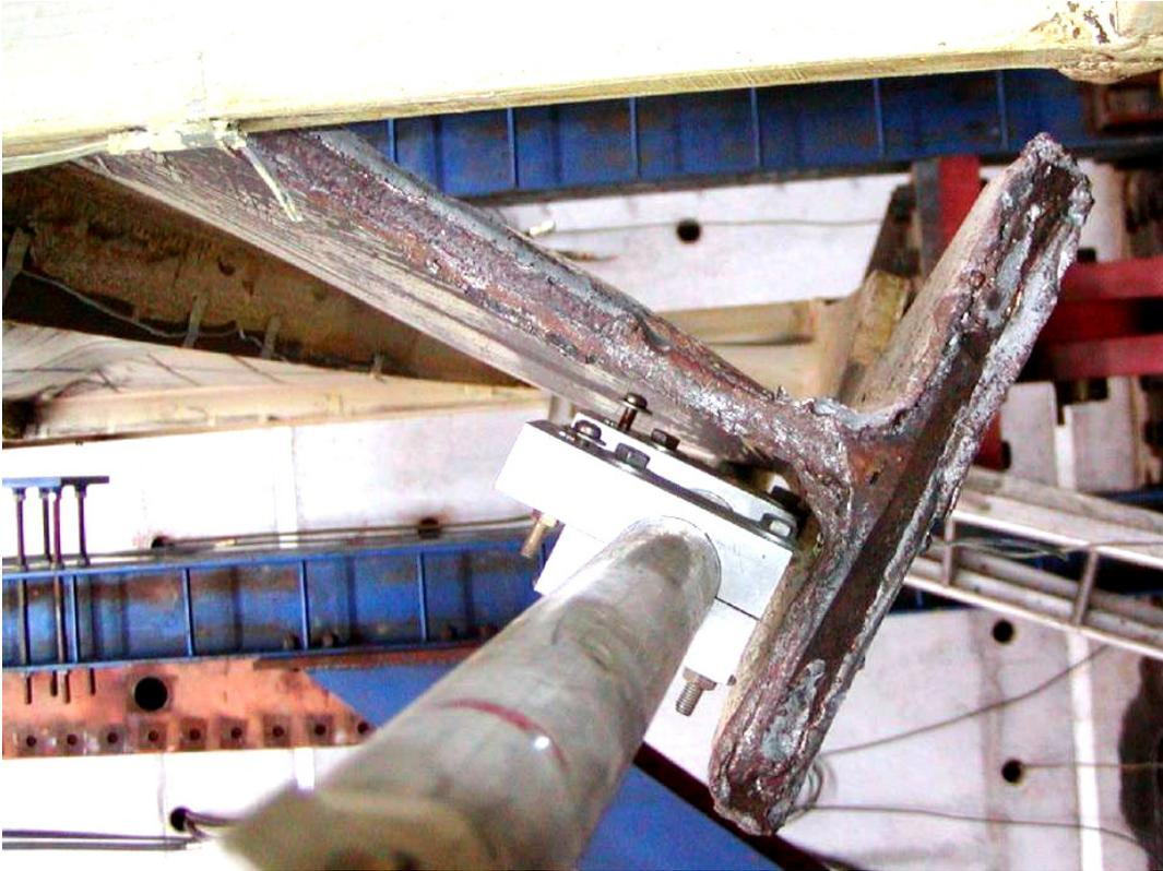
(b) Detail of failed weld surface on beam
