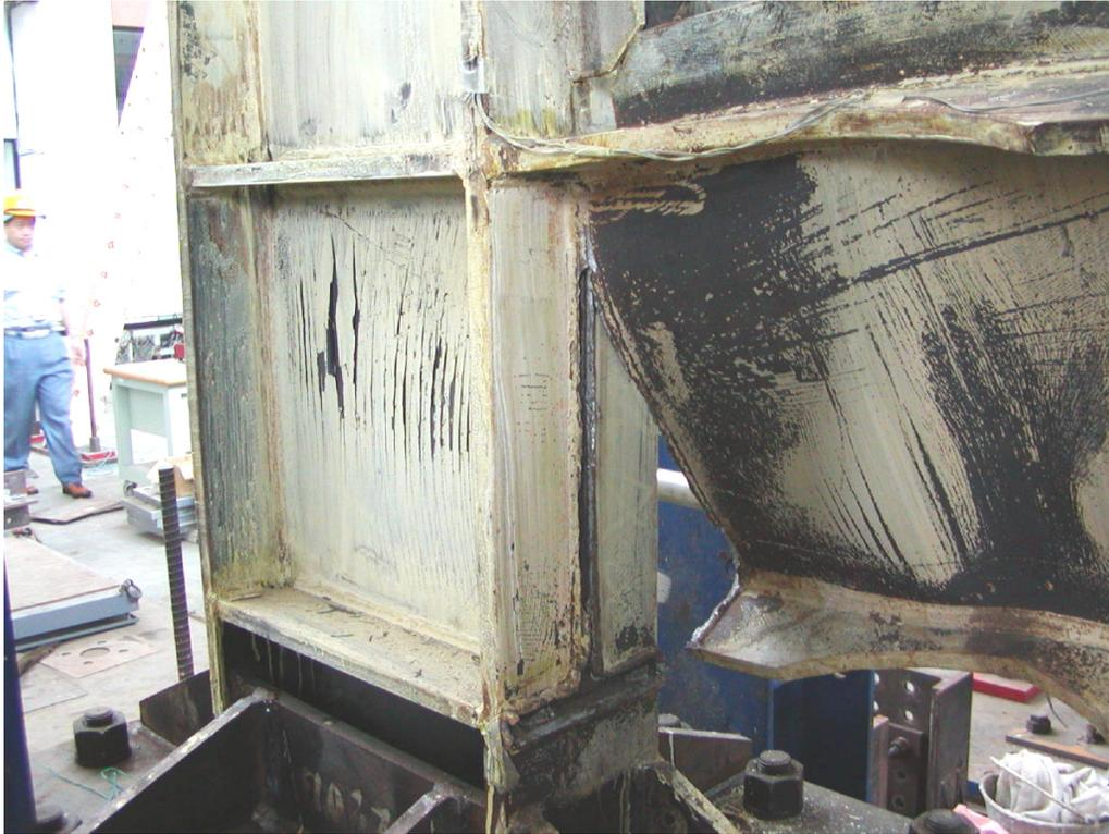
(a) Failed far beam to column connection from B-side
