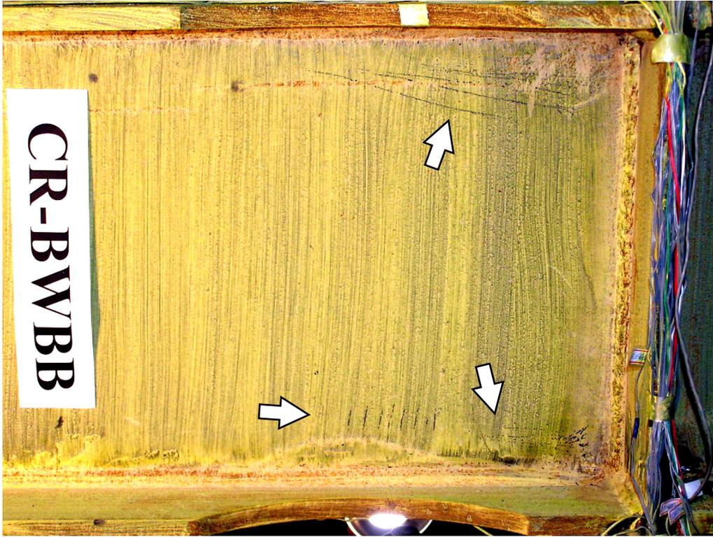
FIGURE 5-44 Bottom beam wall RBS web yielding (CR: Cycle 12,  $\gamma = 0.6\% \approx 2\delta_y$ )
