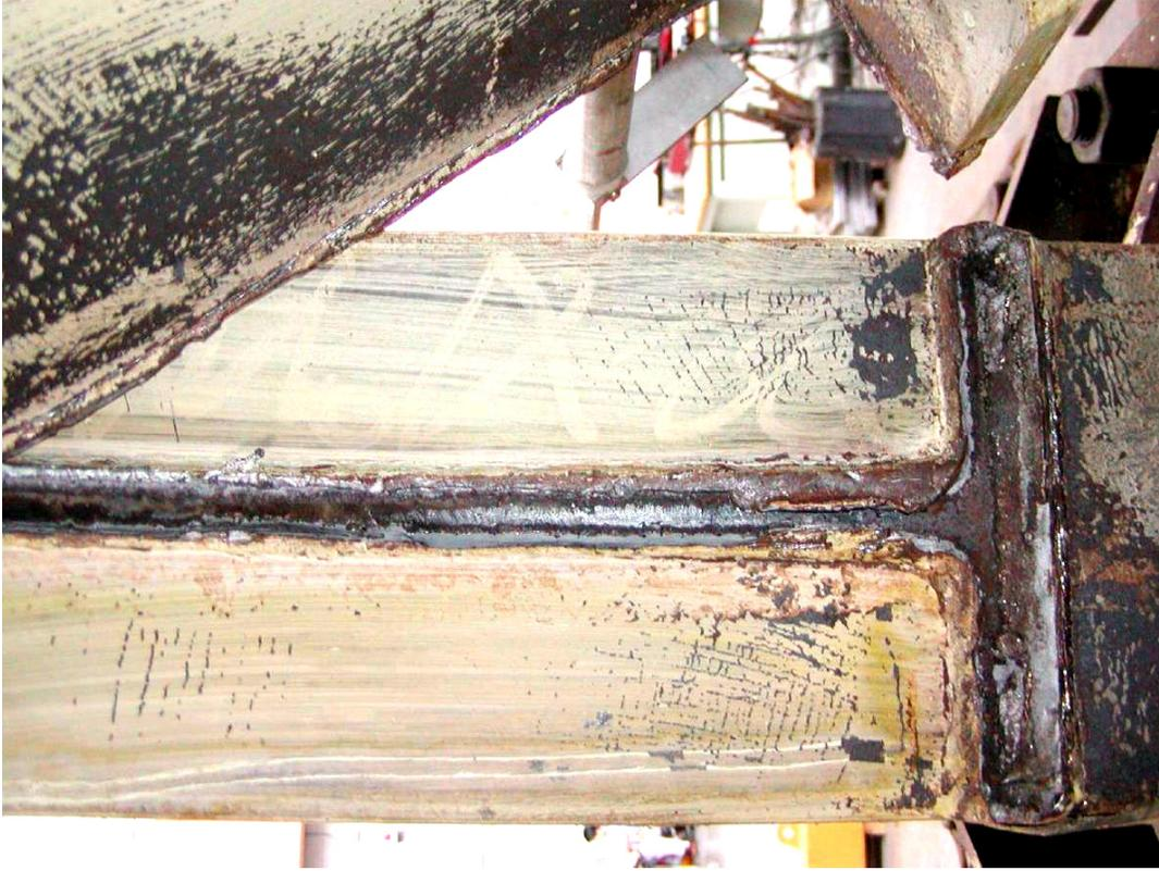
(c) Detail of failed weld surface on column
