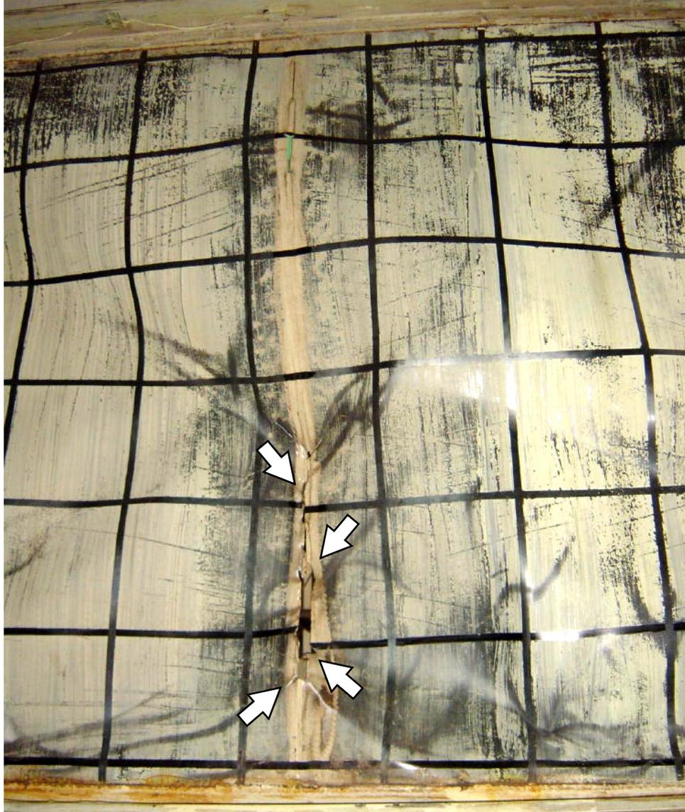
(a) Wall seam weld fractures
