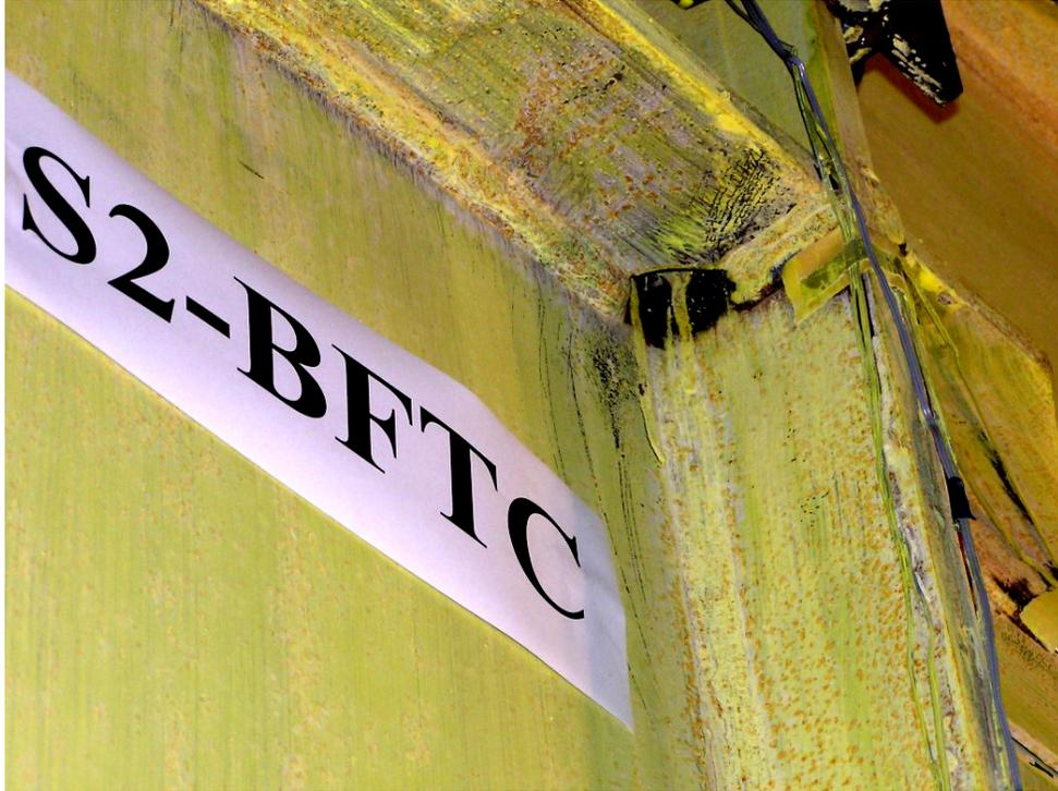
**FIGURE 5-80** Web, flange, and continuity yielding at top of far column
