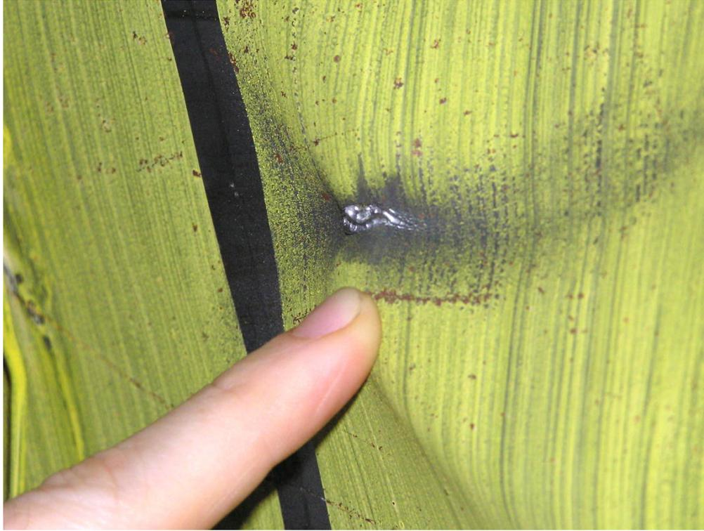
**FIGURE 5-59 Panel fatiguing near bottom of wall column
