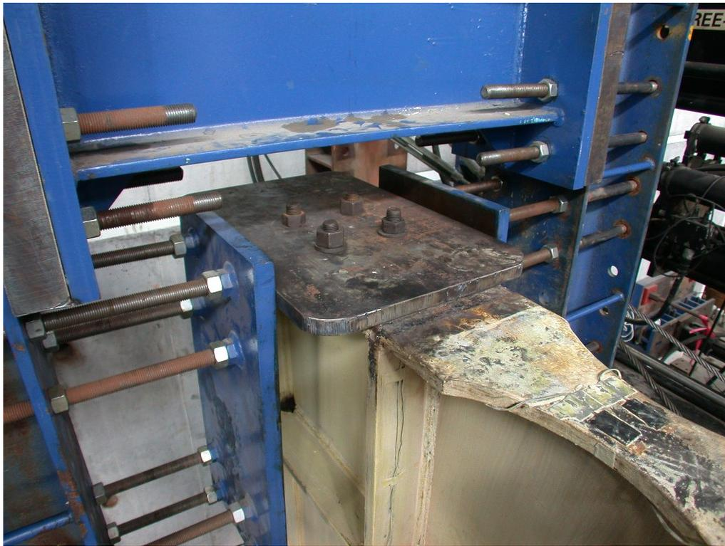
**FIGURE 4-20 Lateral Support at Top of Column
