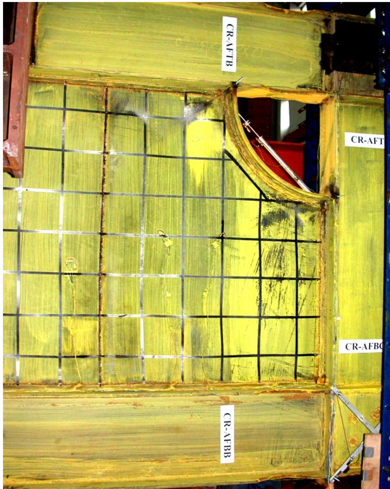
FIGURE 5-47 Infill panel and RBS yielding (CR: Cycle 16-17,  $\gamma = 1.2\% \approx 4\delta_y$ )
