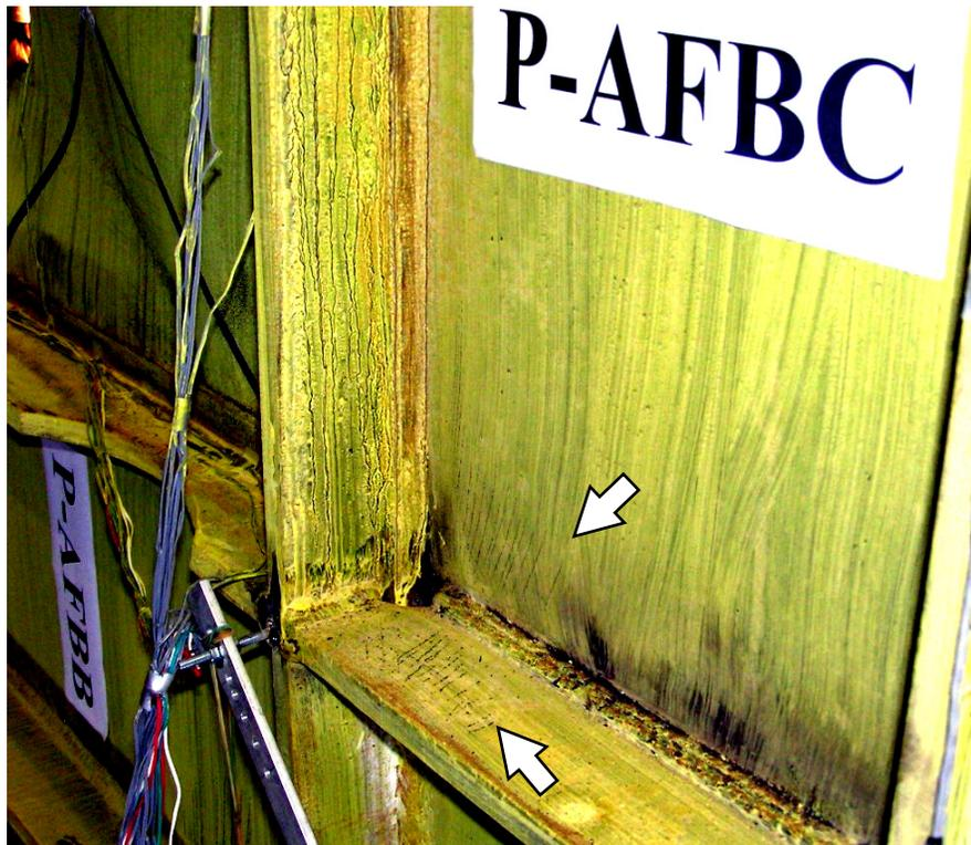
FIGURE 5-16 Yielding in far column web and bottom beam, top flange continuity plate (P: Cycle 16,  $\gamma = 1.2\% \approx 4\delta_y$ )
