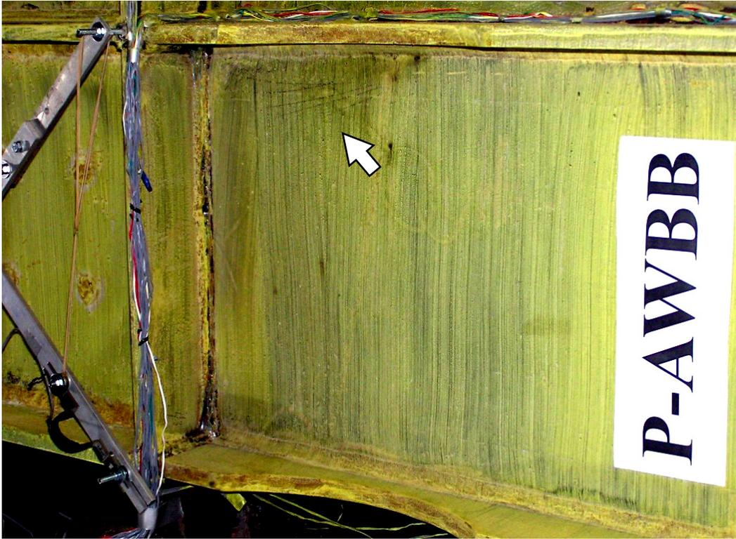
**FIGURE 5-11 Wall side bottom beam RBS web yielding
