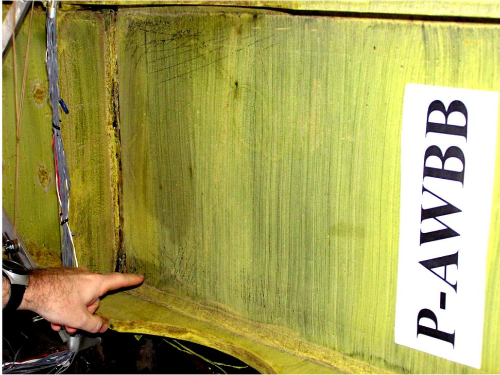
FIGURE 5-12 Wall side bottom beam RBS web yielding (P: Cycle 13,  $\gamma = 0.9\% \approx 3\delta$ )
