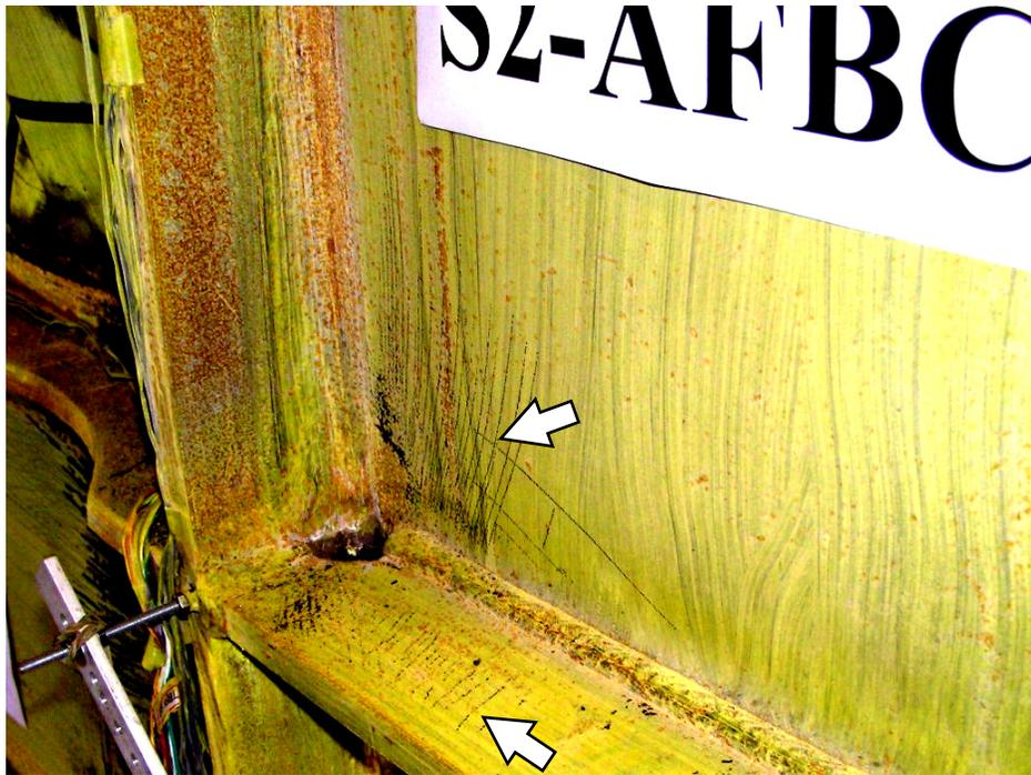
(a) A-side web and bottom beam top flange continuity plate
