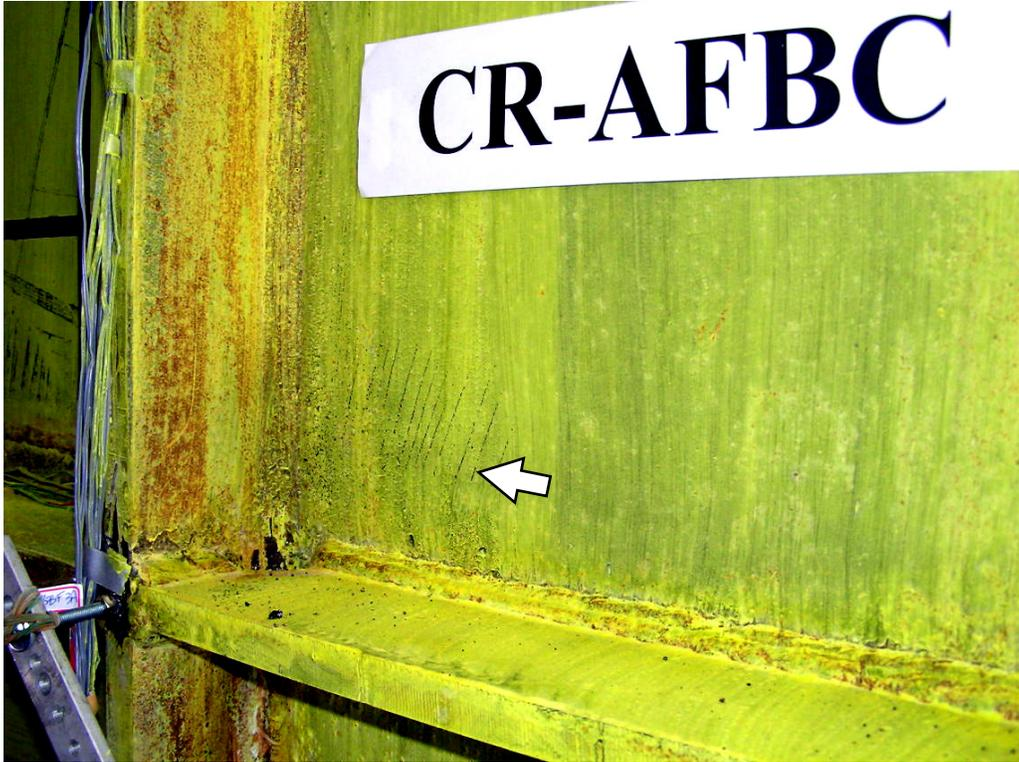
**FIGURE 5-41 Far column web yielding at bottom beam (CR: Cycle 10,  $\gamma = 0.6\% \approx 2\delta$ )**
