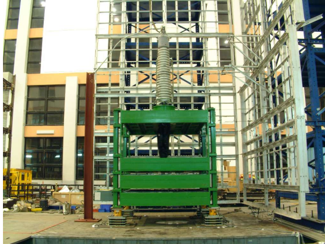
Figure A-1 Cable-Connected Base-Isolated Transformer Model
