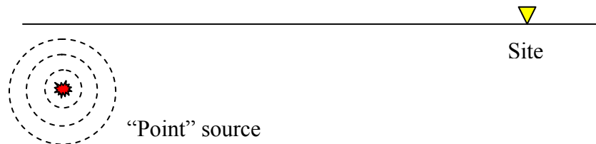
Figure 4-1 Fault-Site Model for Earthquakes in ENA
