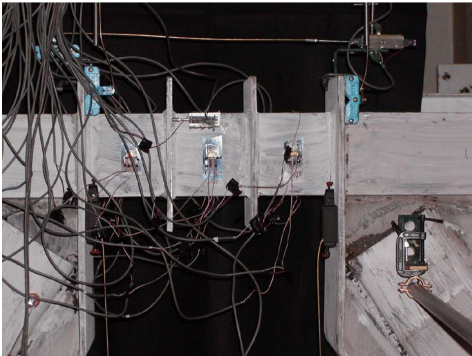
FIGURE 4-18 Instrumented Link Closeup
