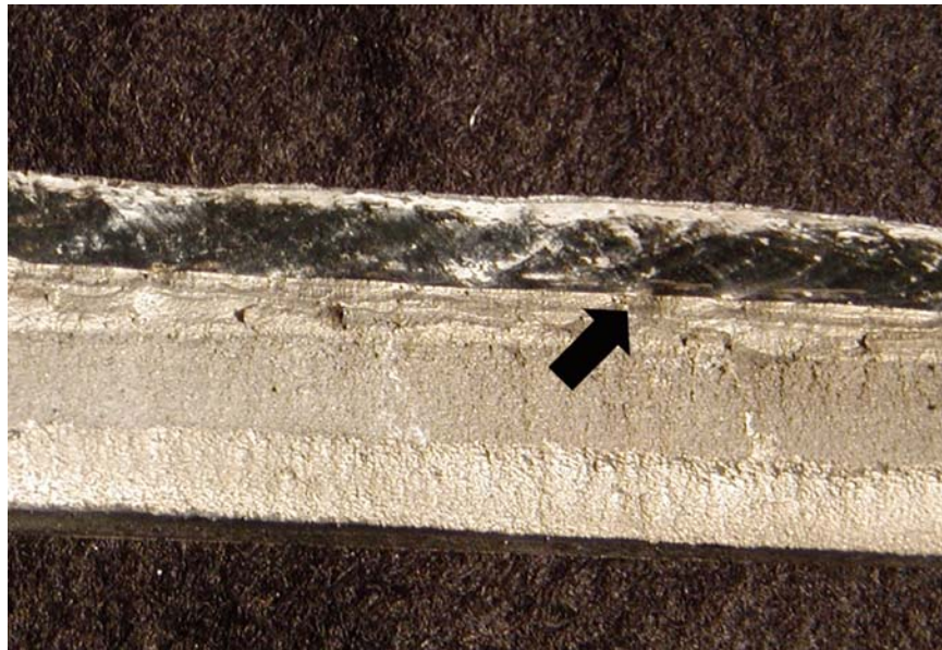
FIGURE 5-23 Second Pitted Region and Another Likely Location of Crack Initiation
