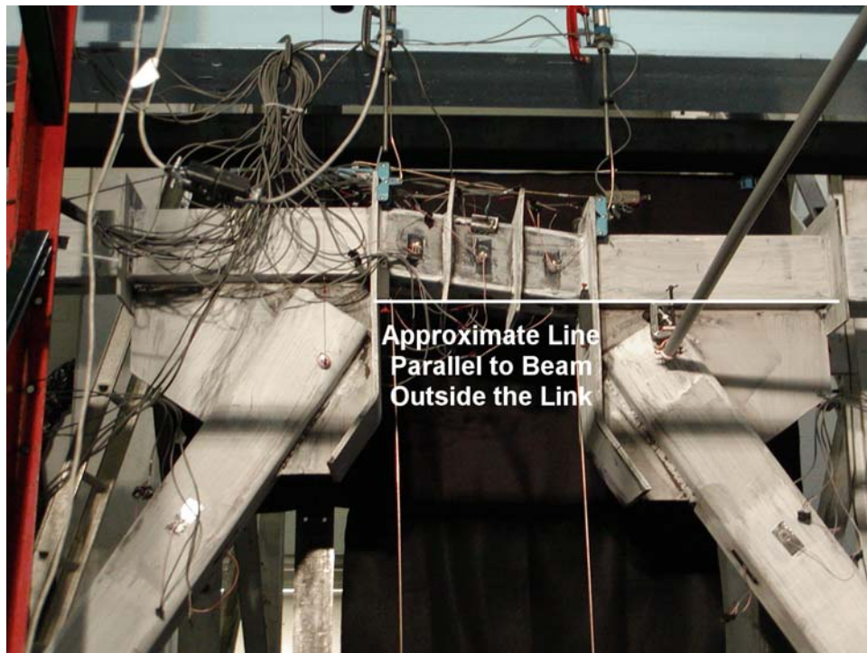
FIGURE 5-12 Deformed Link at 6\delta_y , 2.3\% Drift, 0.151 rads Rotation, Cycle 20
