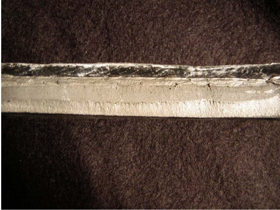
FIGURE 5-20 Fracture Surface on Brace-to-Beam Connection Side-2
