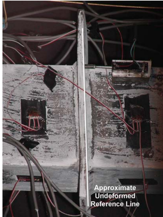
FIGURE 5-8 Curl of Link Stiffener at 4\delta_y , 1.52% Drift, 0.096 rads Rotation, Cycle 17
