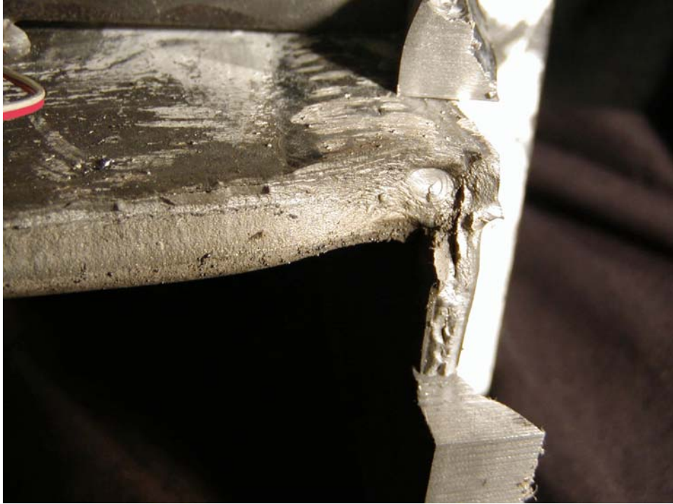
FIGURE 5-18 Fracture Surface on Link Side-3
