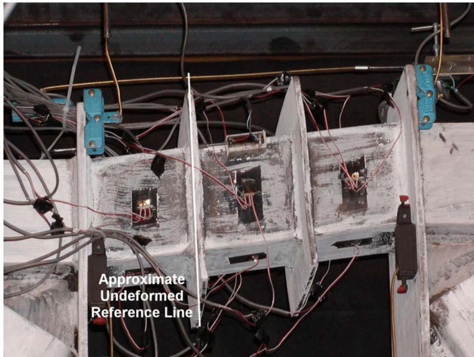
FIGURE 5-11 Curl of Link Stiffeners at -5\delta_y , -1.92\% Drift, -0.123 rads Rotation, Cycle 19
