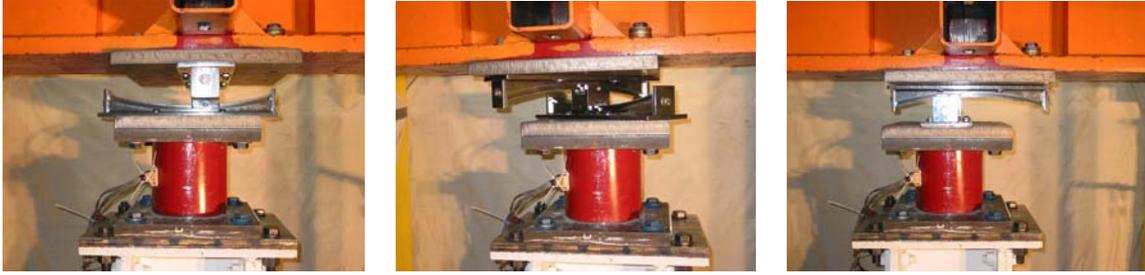
Figure 3-6: Views of XY-FP isolator during testing in 0°, 45°, and 90° orientation.
