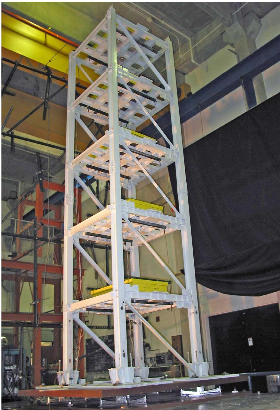
Figure 4-1: Photograph of tested five-story isolated model structure on the seismic simulator at the University at Buffalo.
