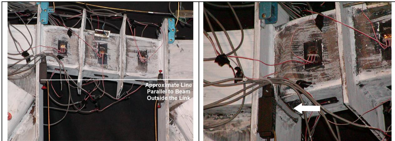
Figure 5a. Link Deformed at 0.123 rads of Rotation During Cycle 19
