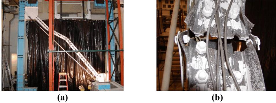
**FIGURE 2-2 Specimen By16-120 (Lee, 2003). (a) Buckled Shape and (b) Final Fracture of Member**
