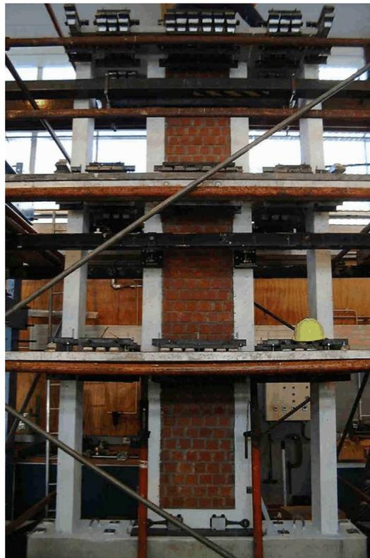
**FIGURE 2-14 Rocking Wall Specimen with Flexural Steel Yielding Devices at Uplifting Location (Toranzo et. al., 2001)**
