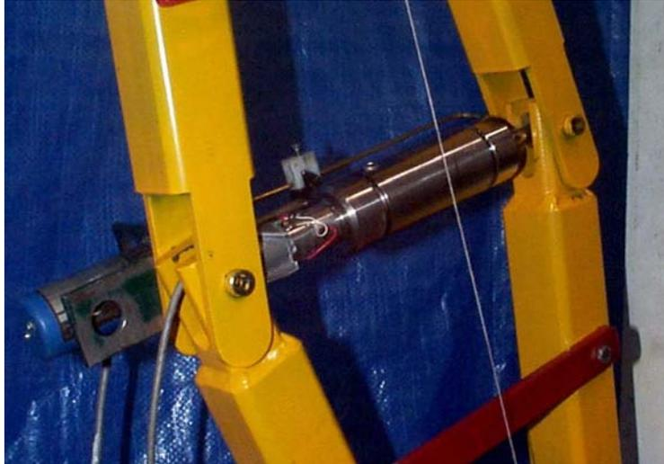
**Figure 3-4 Close-up of Damper-to-Brace Connection Detail**
