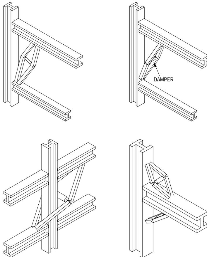
**Figure 2-5 Possible Installation Configurations of Scissor-Jack Damping System**
