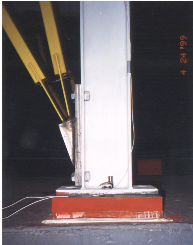
**Figure 3-3** Connection Details of Scissor-Braces to Frame, Scissors-to-Beam (*top*), and Scissors-to-Column (*bottom*) Connection Details
