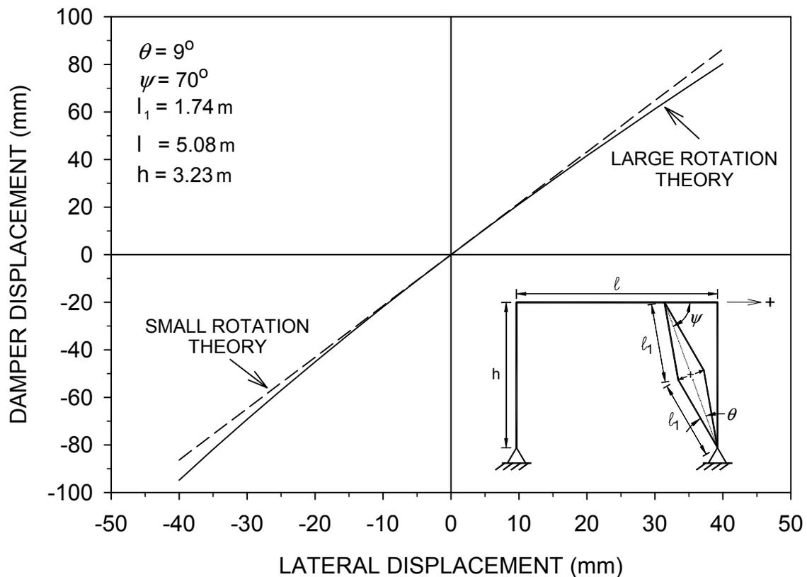
**Figure 2-8 Relation between Damper Displacement and Lateral Displacement**
