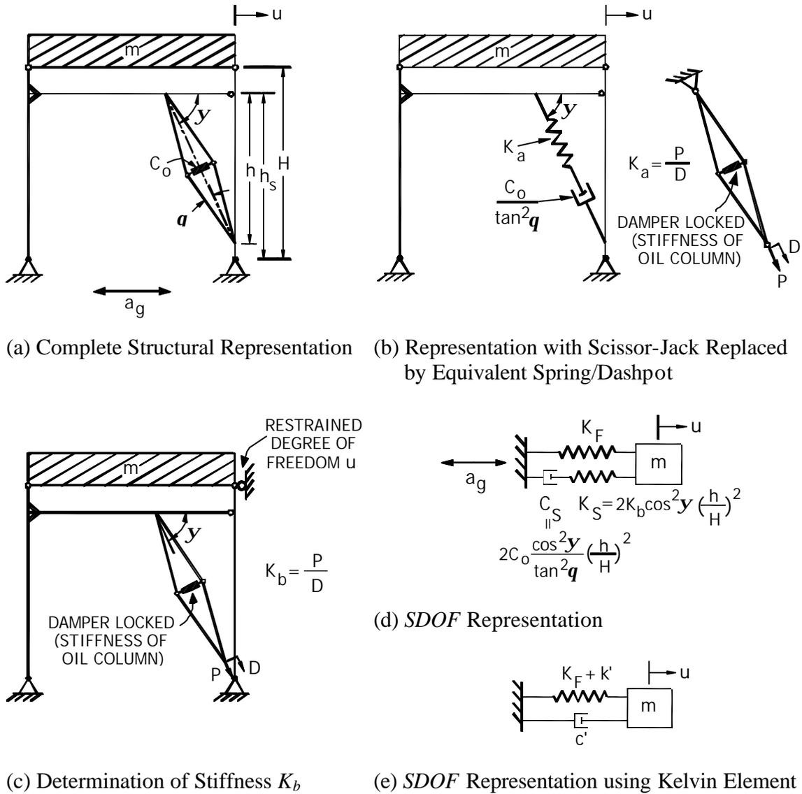
**Figure 6-2 Representation of Structure for Simplified Analysis**
