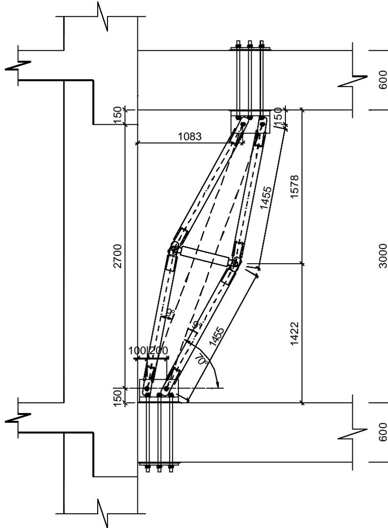
**Figure 7-2** Details of Scissor-Jack-Damper System for Building in Cyprus (typical for 2<sup>nd</sup> and 3<sup>rd</sup> floors; dimensions in mm)
