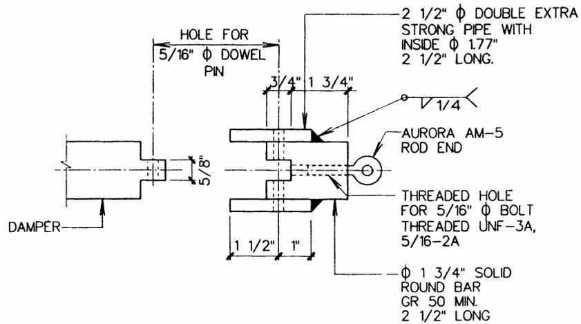
**FF DAMPER END CONNECTION AT JOINT (D)**
