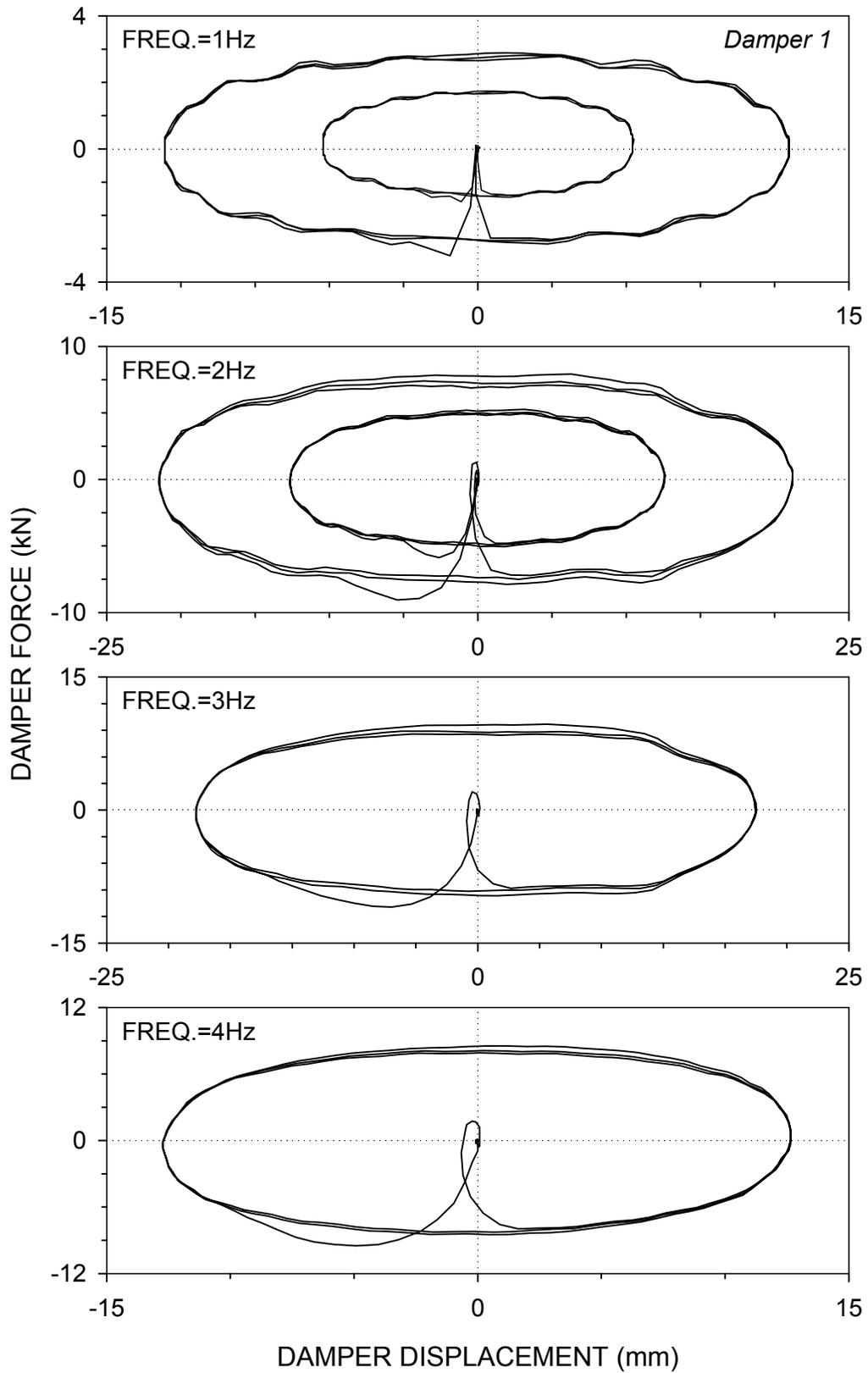
**Figure 3-8 Recorded Force-Displacement Loops of Fluid Viscous Damper**
