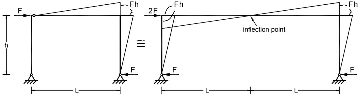
**Figure 3-5 Simplified Sketch of Tested Model and Equivalent Portal Frame of Double Bay Length**
