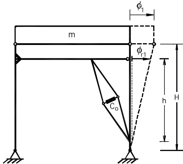
**Figure 6-3 Schematic of Tested Model Showing Modal Displacements**
