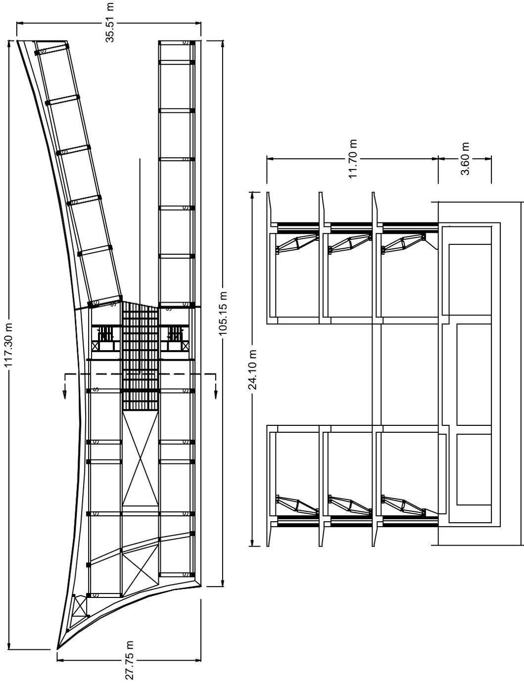
**Figure 7-1** Plan View of 1<sup>st</sup> Floor (*above*) and Elevation View of Building Showing Scissor-Jack-Damper System (*below*)
