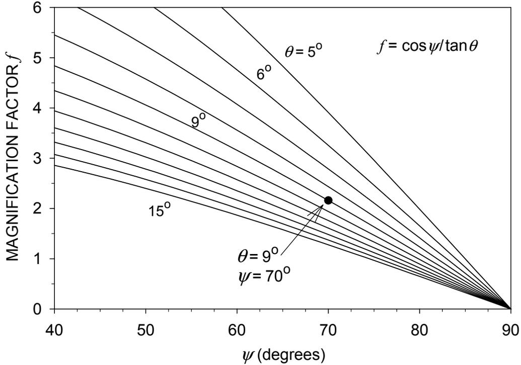
**Figure 2-7 Dependency of Magnification Factor on Scissor-Jack Geometry**
