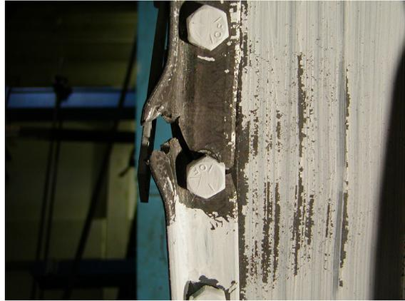
(h) Fracture at  $\delta=1.12''$ (28.5mm)
