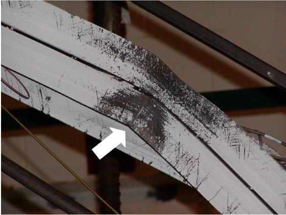
(g) Initial fracture at  $\delta=0.44"$  (11.1mm) near the mid-length of the specimen
