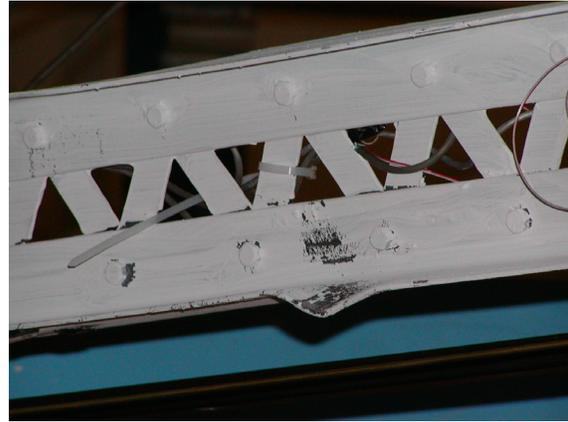
(b) Local buckling at  $\delta=0.13''$ (3.3mm) near the mid-length of the specimen
