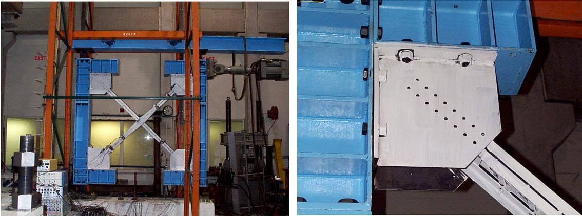
(a) Test set-up
