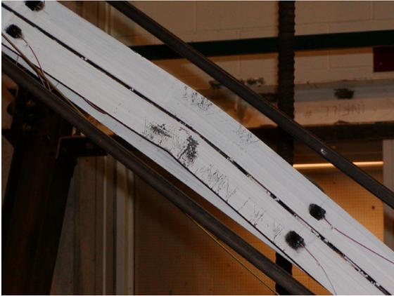
(a) Global buckling at  $\delta=0.13''$ (3.3mm) near the mid-length of the specimen
