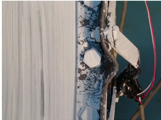
(j) Local and lacing buckling at  $\delta=1.12''$ (28.5mm)
