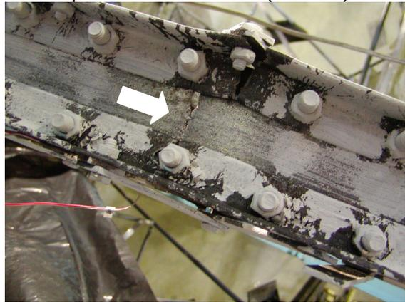
(j) Fracture at  $\delta=0.64''(16.3\text{mm})$
