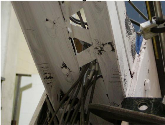
(c) Local buckling at  $\delta=0.13''$ (3.3mm) near the gusset-connection
