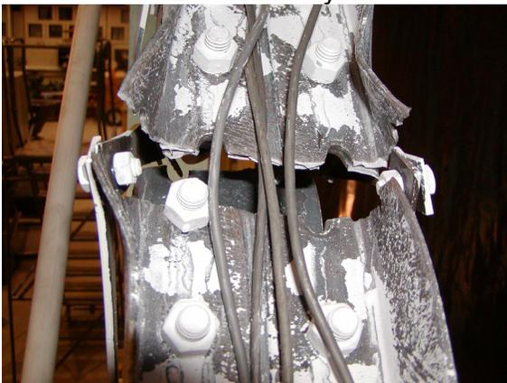
(k) Final fracture at  $\delta=1.40''$ (35.6mm)
