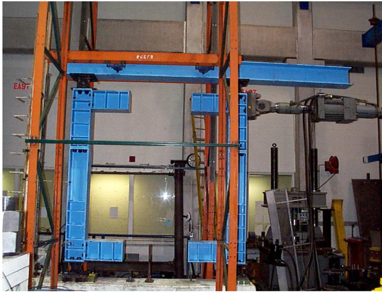
Figure 4.7 Test set-up for Bare Frame Test
