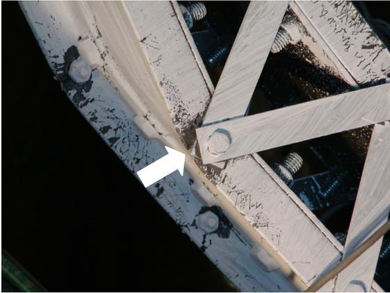
(g) Fracture at  $\delta=1.12''$ (28.5mm)
