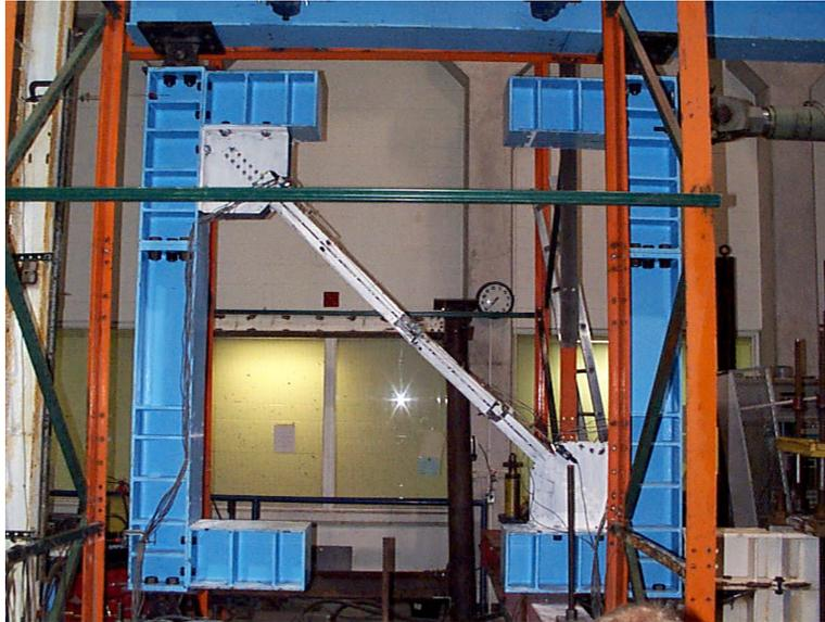
Figure 4.12 Test set-up for the Ay8-120 specimen
