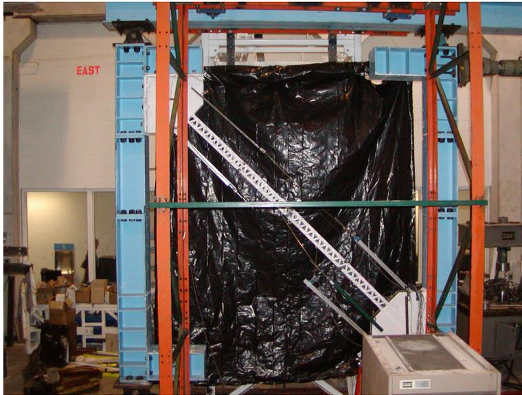
Figure 4.36 Test set-up for the Bx8-120 specimen
