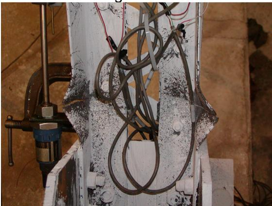
(k) Fracture at  $\delta=1.06"$  (26.8mm) near gusset-connection
