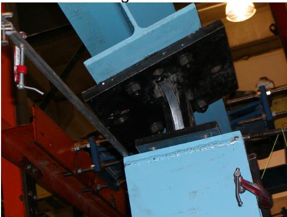
(e) Damaged hinge at  $\delta=0.35''$ (8.9mm)
