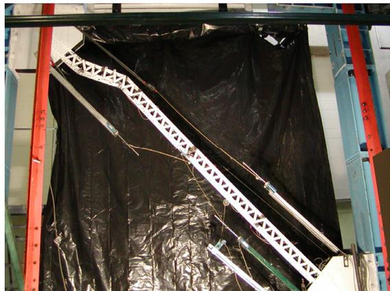
(l) Global fractured shape at  $\delta=0.96''(24.4\text{mm})$
