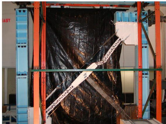
(l) Global fractured shape at  $\delta=1.63''$ (16.0mm)
