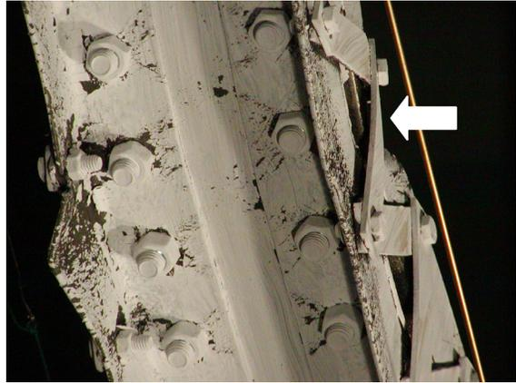
(h) Lacing buckling at  $\delta=0.68''(17.3\text{mm})$
