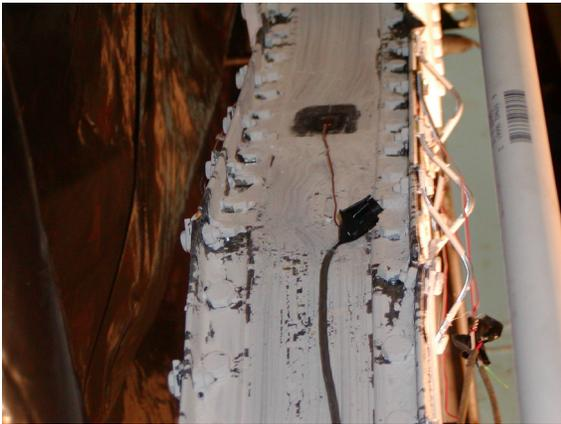
(i) Fracture and lacing buckling at  $\delta=0.7''$ (17.8mm)
