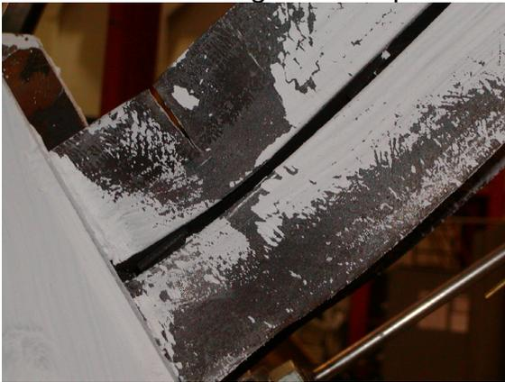
(i) Fracture at  $\delta=0.97"$  (24.5mm) near the gusset-connection
