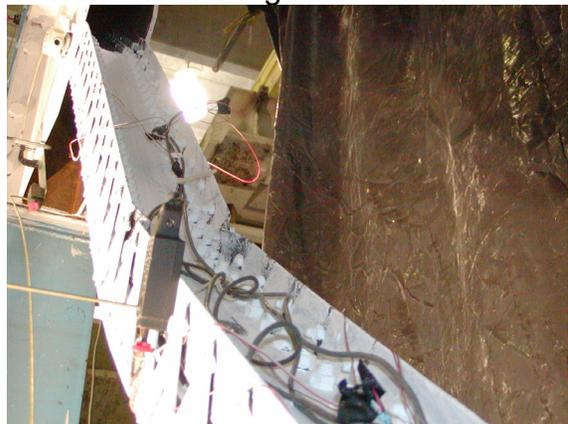
(f) Local buckling at  $\delta=0.34''$ (8.6mm) near the mid-length of the specimen
