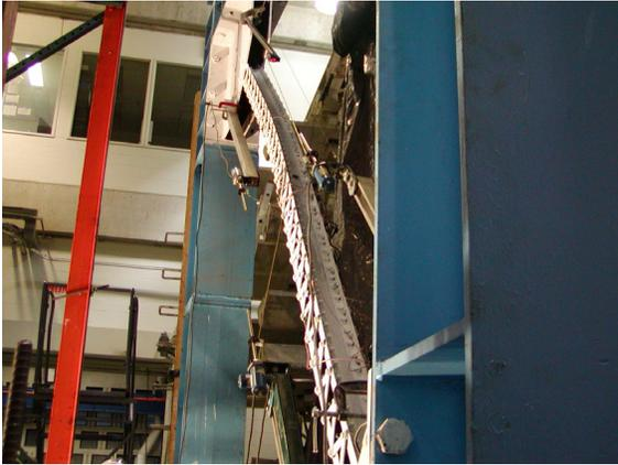
(a) Global out-of-plane buckling at  $\delta=0.16''$  (4.1mm)
