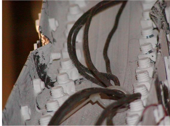
(b) Local buckling at  $\delta=0.17''$ (4.3mm) near the mid-length of the specimen
