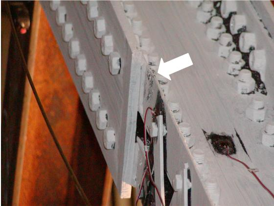
(a) Local buckling at  $\delta=0.16''(4.1\text{mm})$  near the middle connection plate
