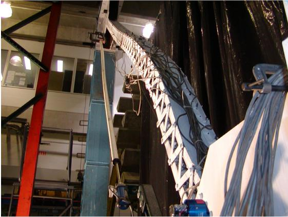
(a) Global buckling at  $\delta=0.28''(7.11\text{mm})$
