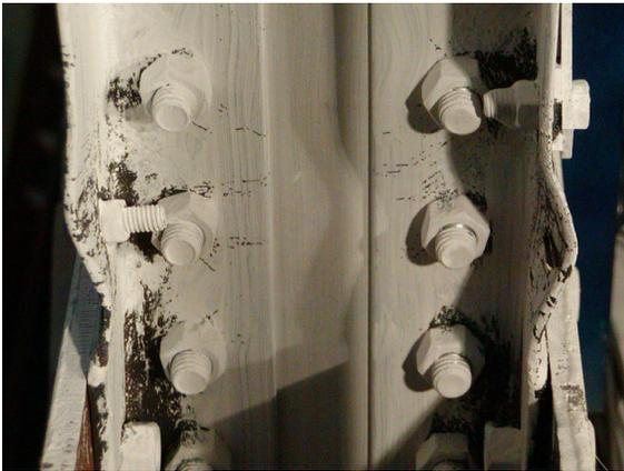
(c) Local buckling at  $\delta=0.17''$ (4.3mm) near the South gusset-connection
