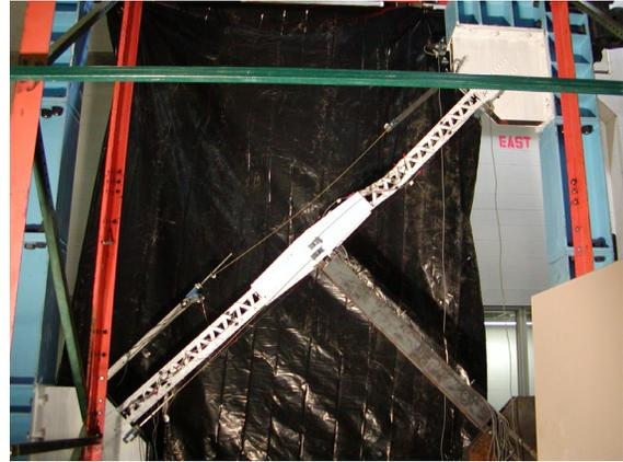
(b) Global in-plane buckling at  $\delta=0.27''$ (6.9mm)
