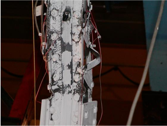
(g) Lacing buckling at  $\delta=0.45''$ (11.4mm)
