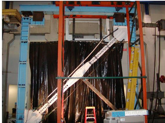
(j) Global fractured shape at  $\delta=0.60''$ (15.2mm)
