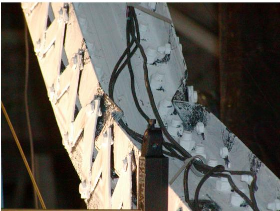
(k) Local buckling at  $\delta=0.86''(21.8\text{mm})$
