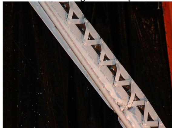
(f) Lacing buckling at  $\delta=0.56''$ (14.2mm)
