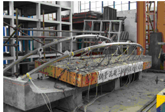
Figure 2. Model collapse during shaking table test
