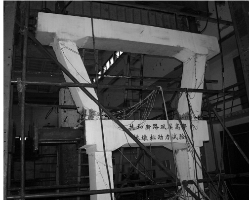
Figure 6. The collapse mechanism of the model after PSD test
