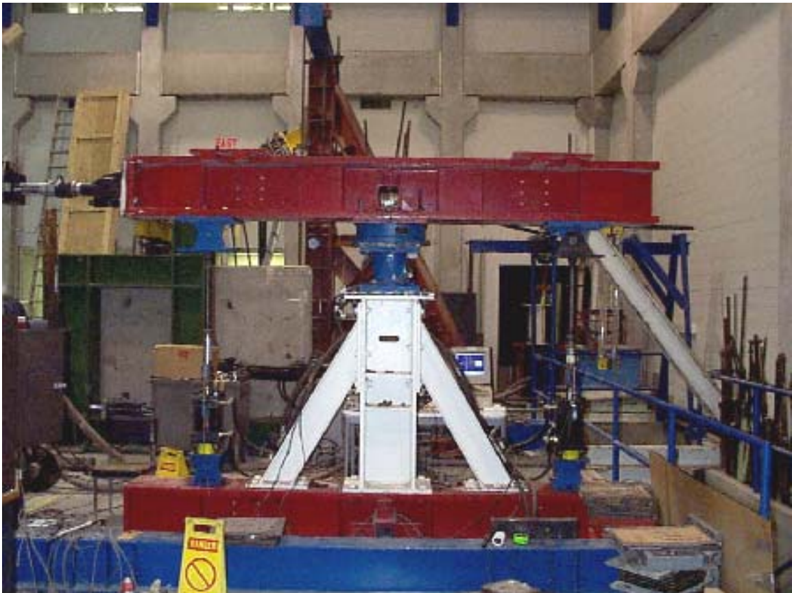
FIGURE 3-2 Photograph of Machine Used to Test Individual Isolators
