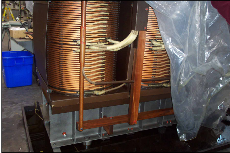
Figure 5. Internal components of a transformer
