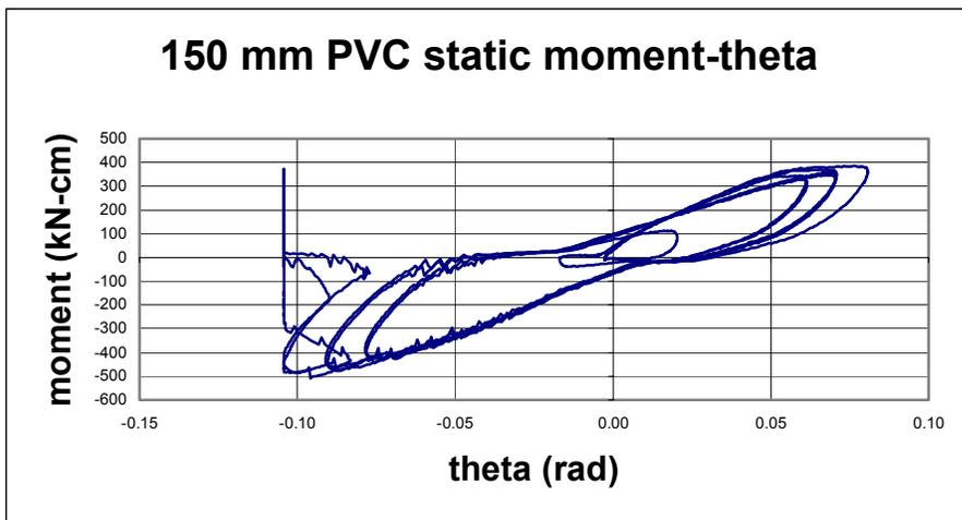
**Figure C-24 Static Moment-Theta for 150 mm PVC Pipe**
