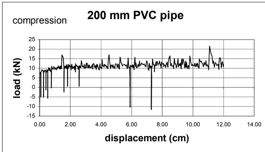
Figure A-19 Load-Displacement for 200 mm PVC Pipe
