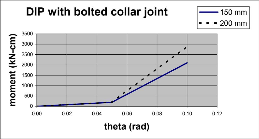
**Figure 4-23 Static Moment-Theta Plot for Ductile Iron Pipe with Bolted Collar Joints**
