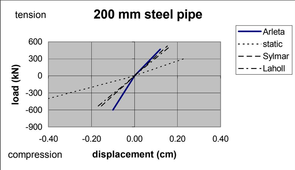
Figure 3-21 Load-Displacement Curves for 200 mm Steel Pipe
