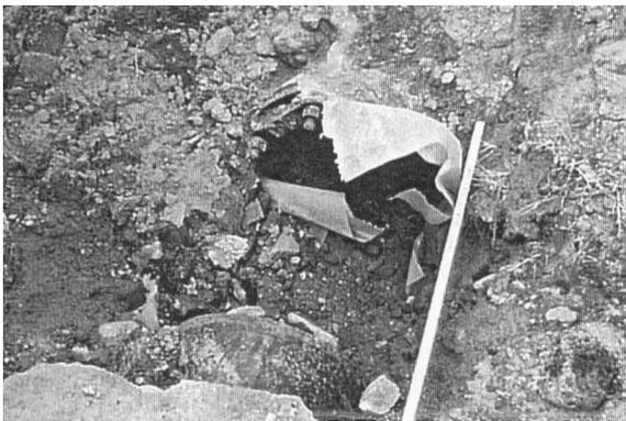
**Figure 1-7 Slip-Out of Joint on 300 mm Dia. Ductile Iron Pipe from the Kobe Earthquake (Ref: Iwamoto 1995)**
