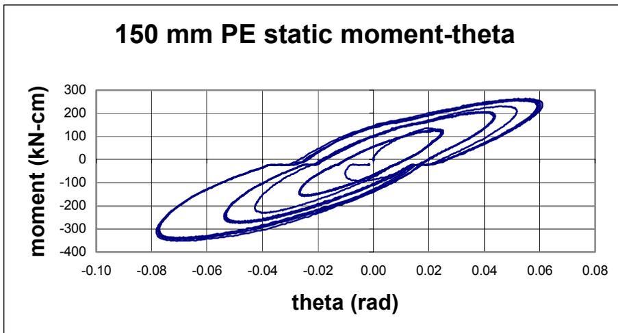
**Figure C-28 Static Moment-Theta for 150 mm PE Pipe**
