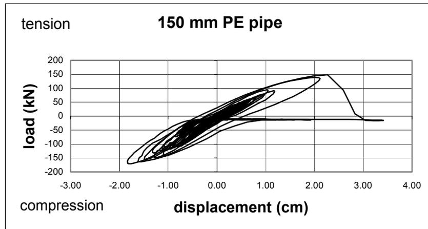
**Figure B-14 Load-Displacement for 150 mm PE Pipe**
