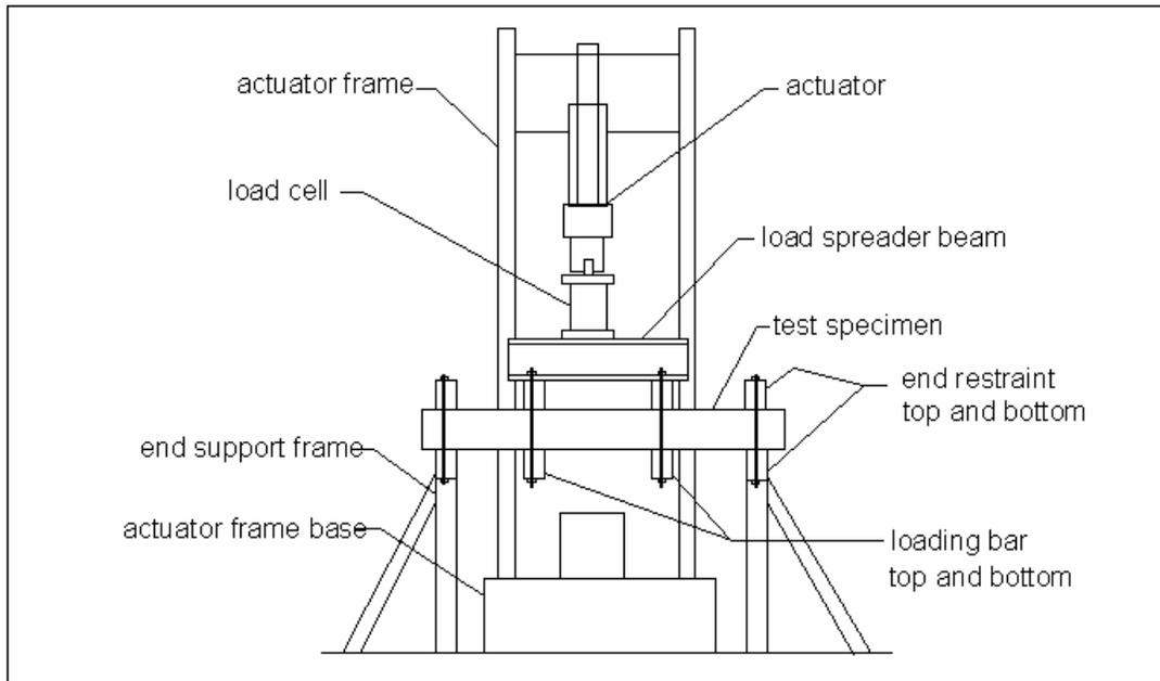
**Figure 4-3 Location of External Instrumentation for Bending Testing**
