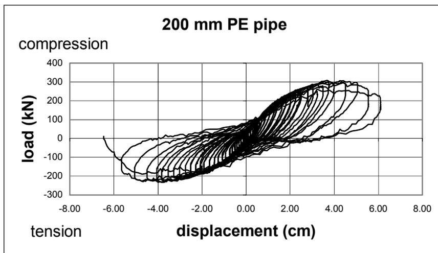
Figure A-22 Load-Displacement for 200 mm PE Pipe
