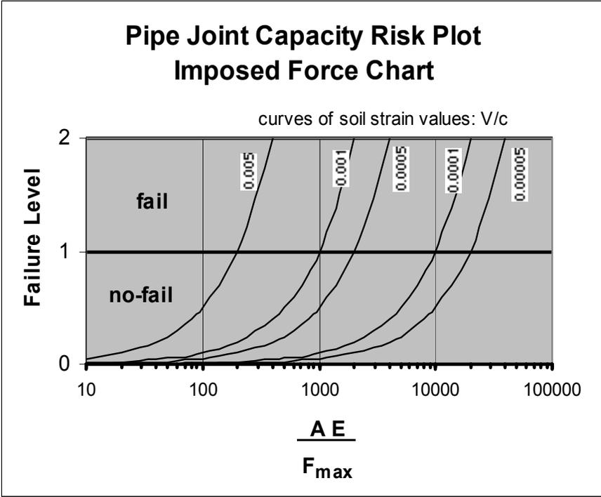
Figure 5-1 Pipe Joint Capacity Chart (see Eq. 5-2)
