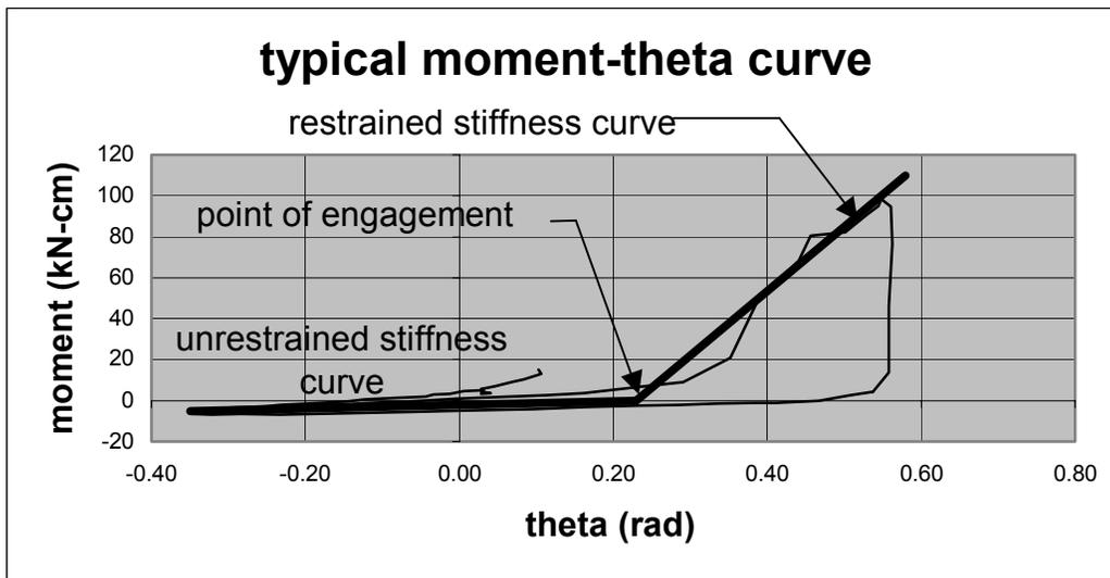
Figure 4-4 Typical Moment-Theta Plot with Approximated Straight-Line Curves
