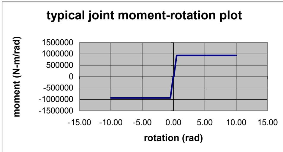
Figure 5-10 Laboratory Measured Typical Joint Moment-Rotation Plot
