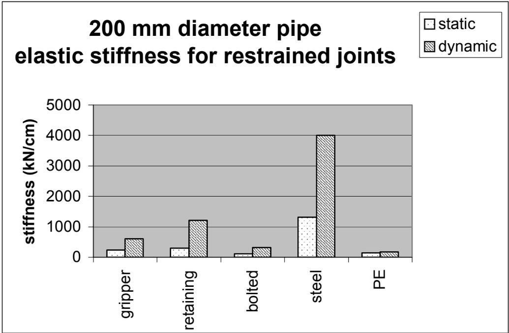
**Figure 3-38 Static-Dynamic Elastic Stiffness Comparison
