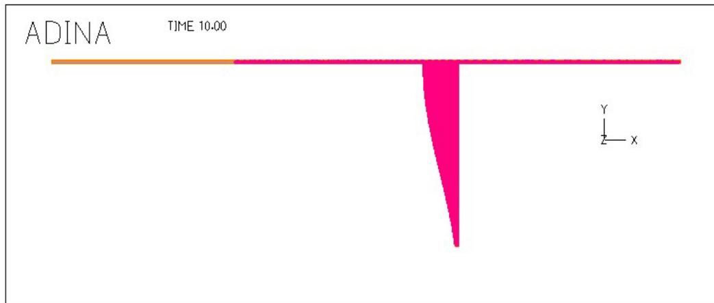
**Figure 5-14 Applied Displacement Amplitude Pattern on Tee Branch**
