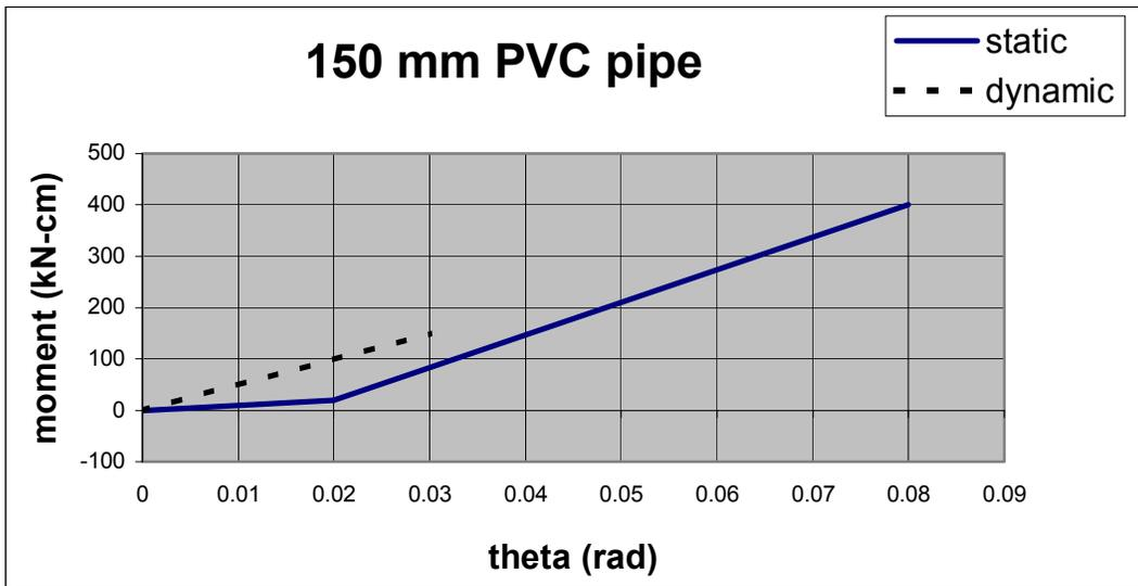
**Figure 4-16 Moment-Theta Plot for 150 mm Diameter PVC Pipe**
