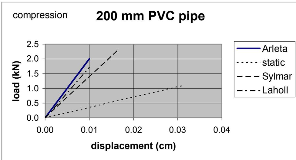
**Figure 3-23 Load-Displacement Curves for 200 mm PVC Pipe**
