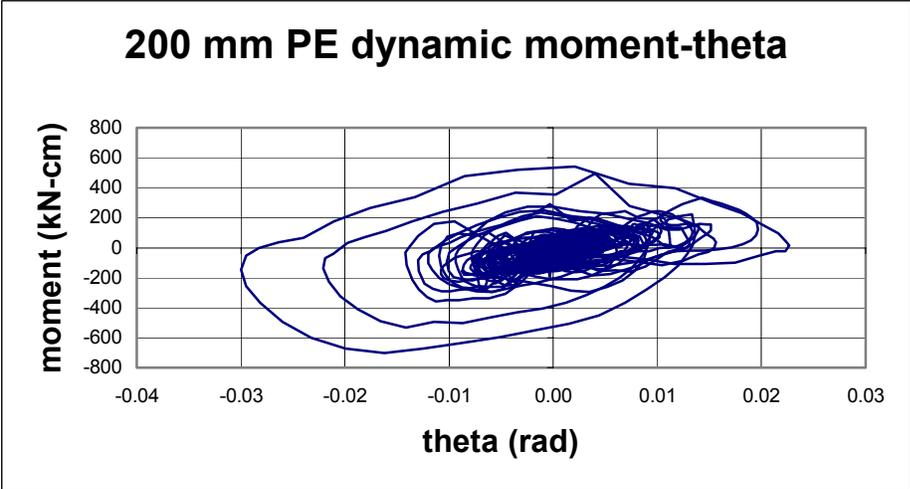
**Figure C-29 Dynamic Moment-Theta for 200 mm PE Pipe**
