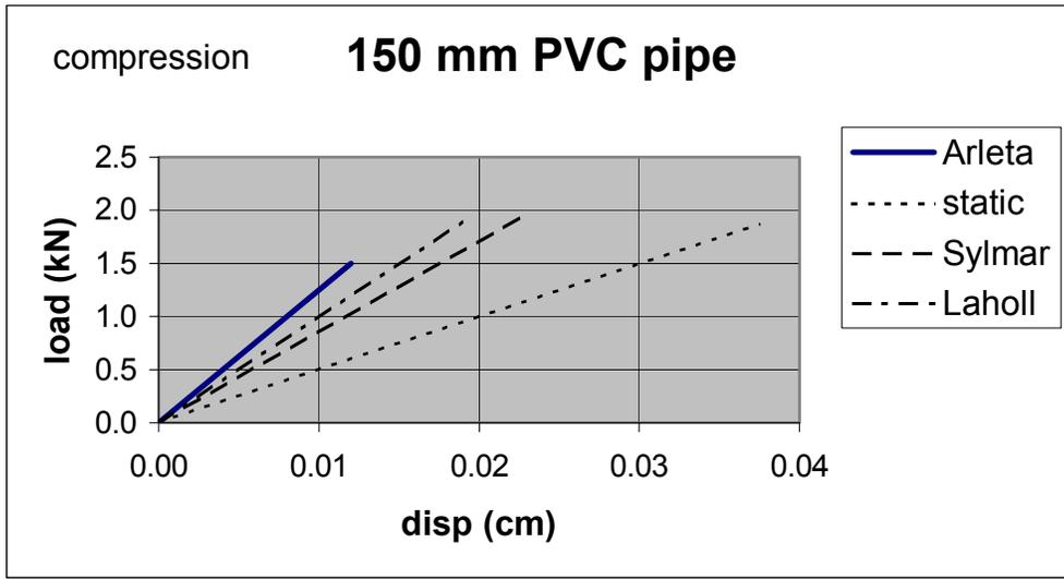
**Figure 3-22 Load-Displacement Curves for 150 mm PVC Pipe**
