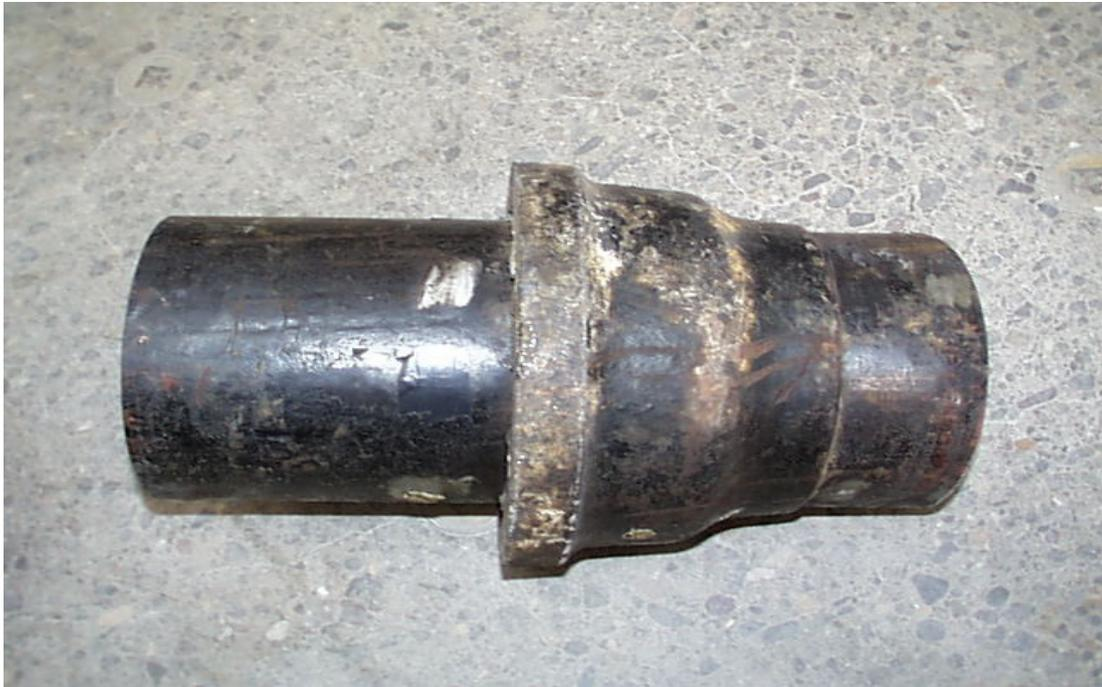
**Figure 1-10 Cast Iron Pipe with Lead-Caulked Joint**
