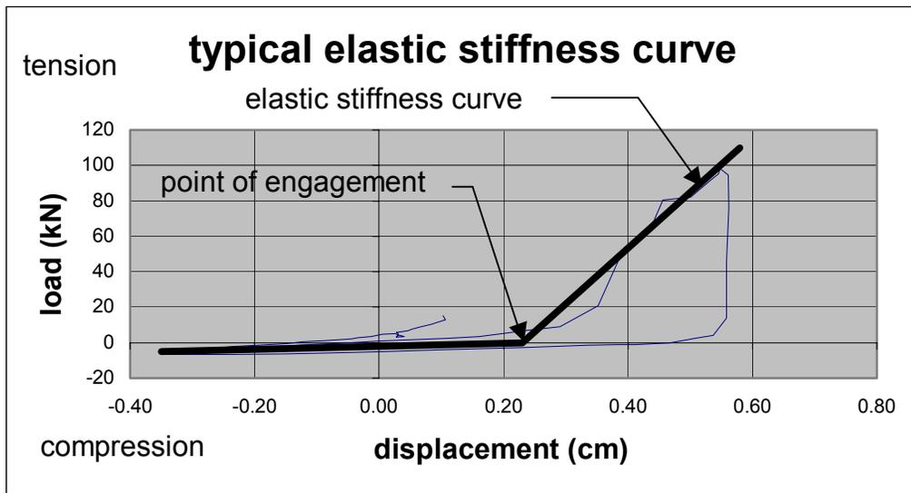
Figure 3-10 Typical Elastic Stiffness Curve for Restrained Joints
