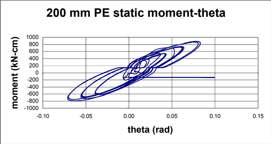
**Figure C-30 Static Moment-Theta for 200 mm PE Pipe**
