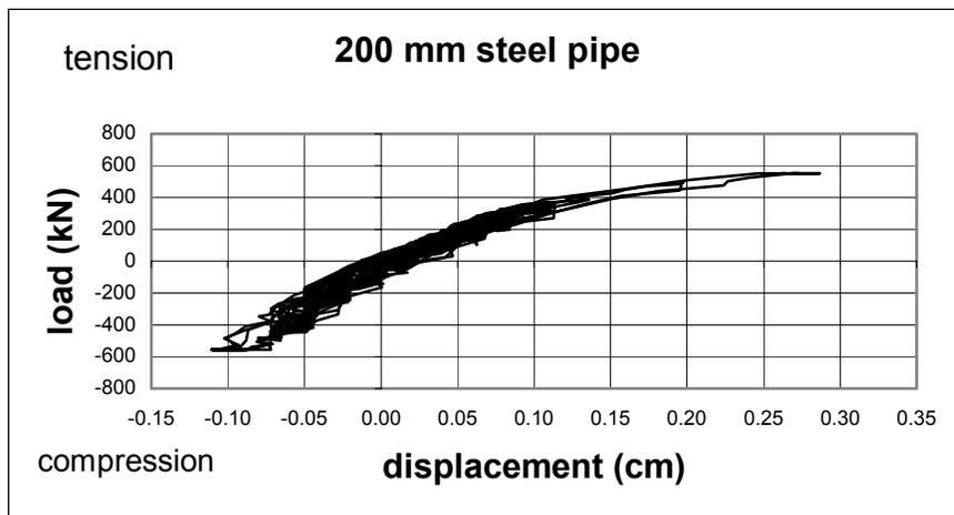
Figure B-11 Load-Displacement for 200 mm Steel Pipe
