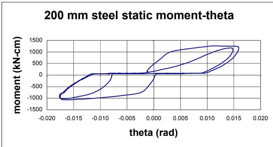
**Figure C-22 Static Moment-Theta for 200 mm Steel Pipe**
