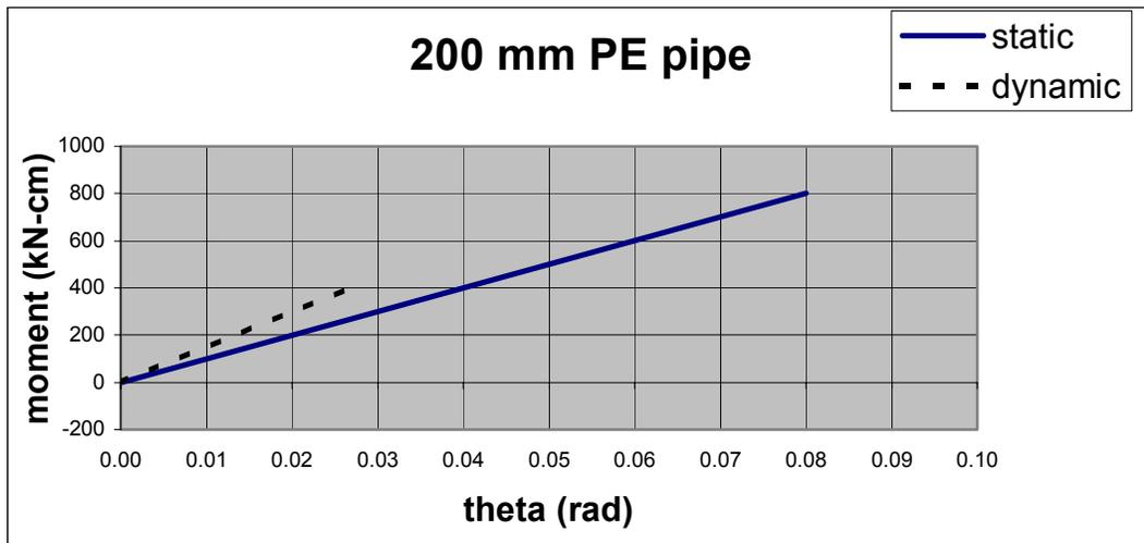
**Figure 4-19 Moment-Theta Plot for 200 mm Diameter PE Pipe**
