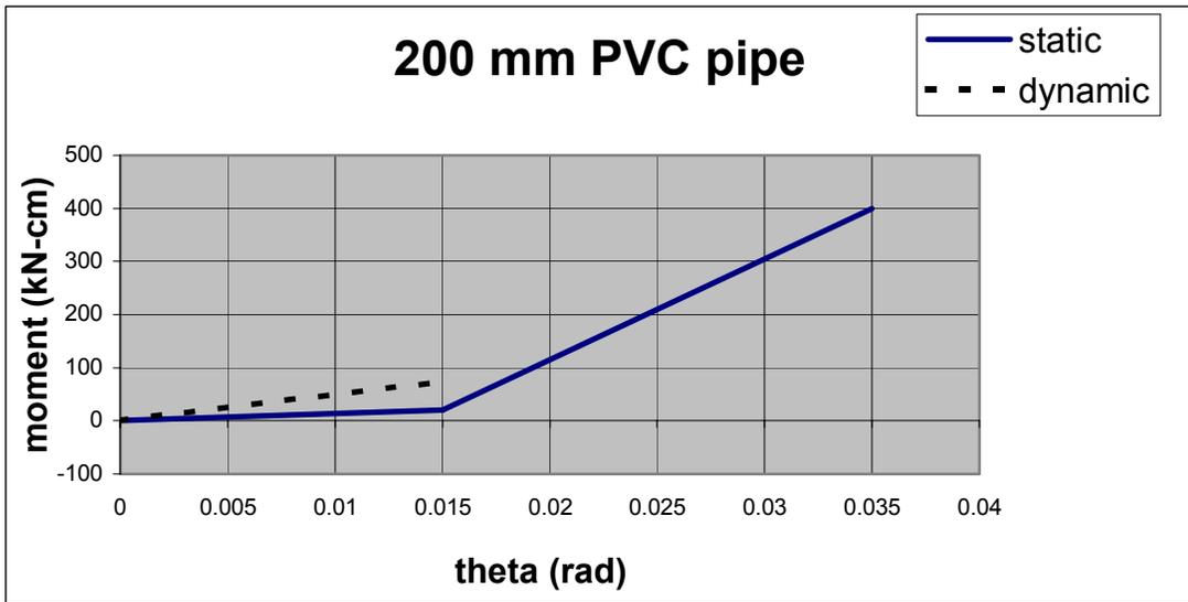
Figure 4-17 Moment-Theta Plot for 200 mm Diameter PVC Pipe
