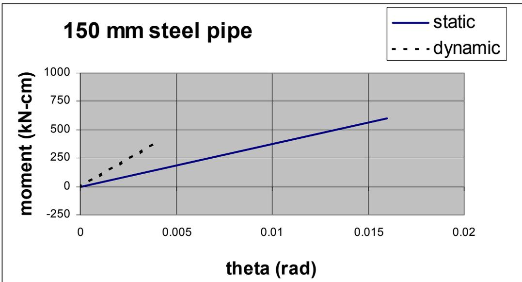
**Figure 4-14 Moment-Theta Plot for 150 mm Diameter Steel Pipe**
