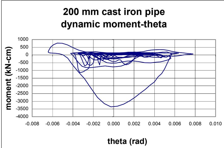
**Figure C-1 Dynamic Moment-Theta for 200 mm Cast Iron Pipe**
