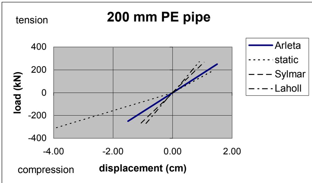
**Figure 3-25 Load-Displacement Curves for 200 mm PE Pipe**
