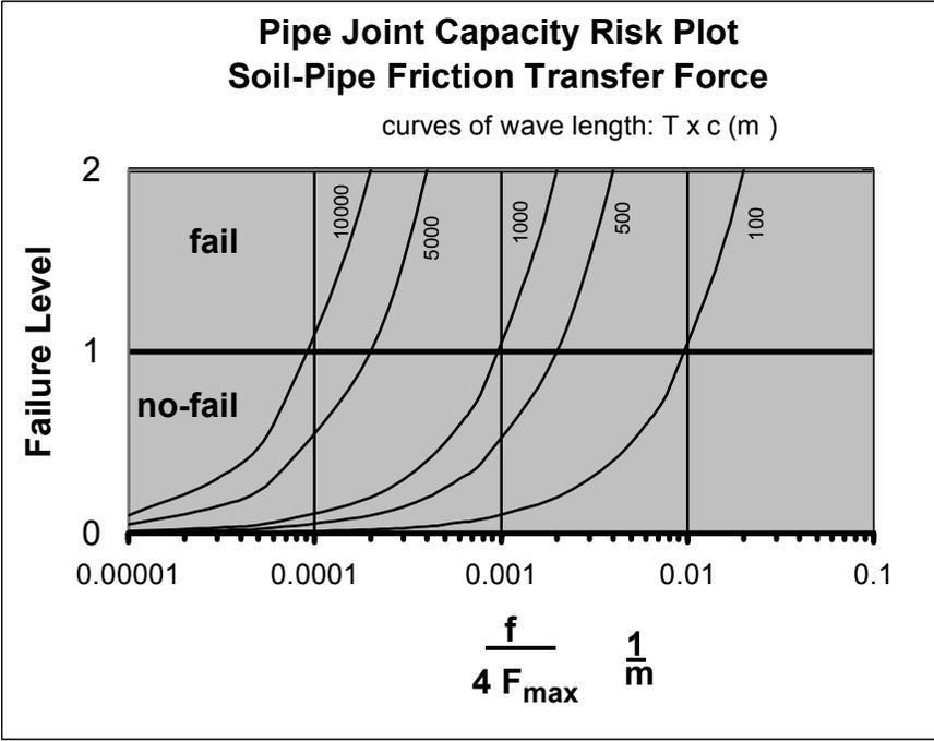
Figure 5-2 Pipe-Soil Friction Transfer Chart (see Eq. 5-3)
