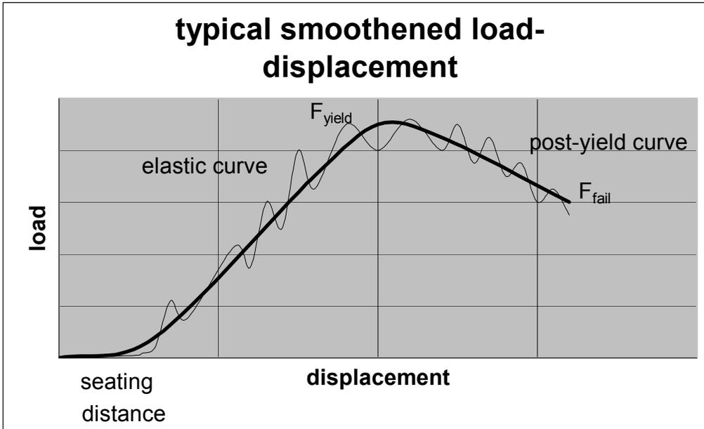
**Figure 2-4 Typical Smoothened Load-Displacement Plot Showing Key Zones and Points**
