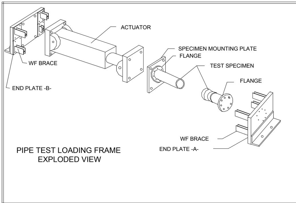
**Figure 2-2 Exploded View of Actuator, Test Specimen, and Loading Frame**
