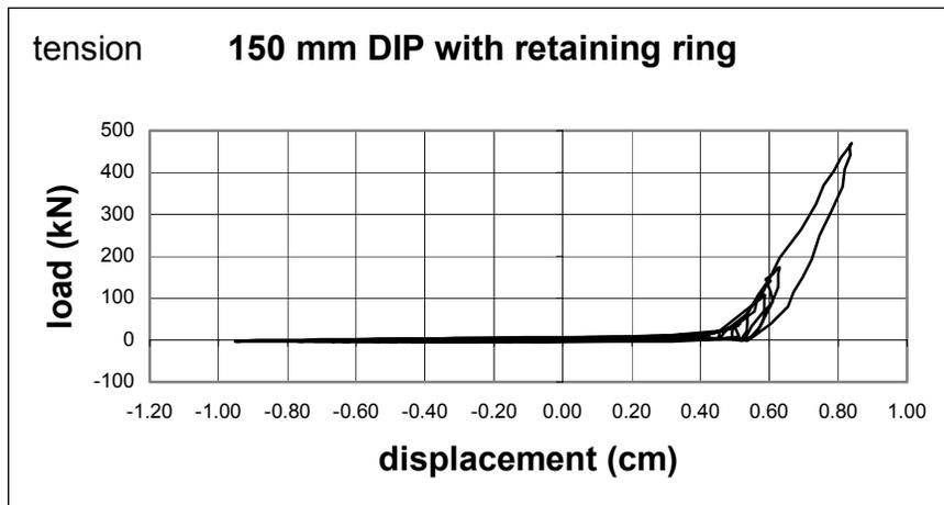
Figure B-6 Load-Displacement for 150 mm DIP with Retaining Ring Joint
