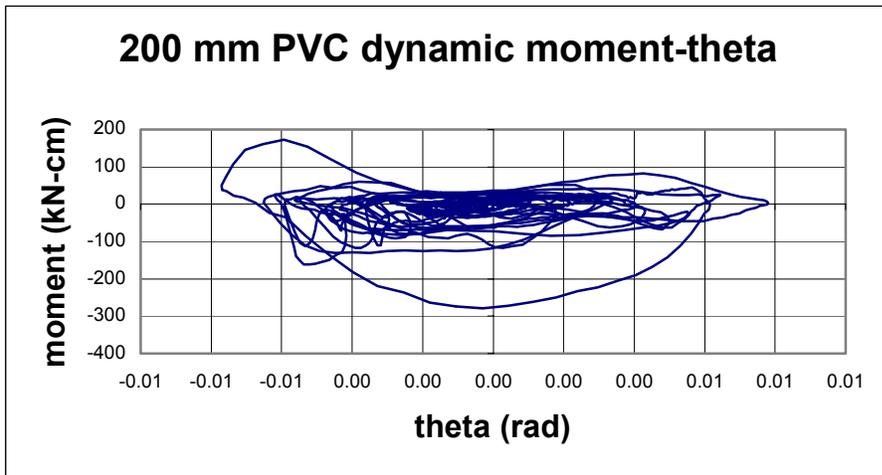
**Figure C-25 Dynamic Moment-Theta for 200 mm PVC Pipe**
