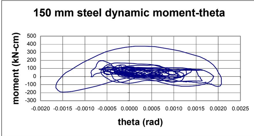
**Figure C-19 Dynamic Moment-Theta for 150 mm Steel Pipe**
