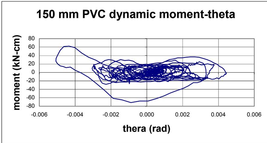
**Figure C-23 Dynamic Moment-Theta for 150 mm PVC Pipe**
