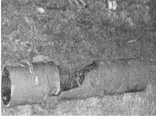
**Figure 1-1 Ruptured 150 mm Dia. Cast Iron Pipe from the Northridge Earthquake (Ref: LADWP 1999)**
