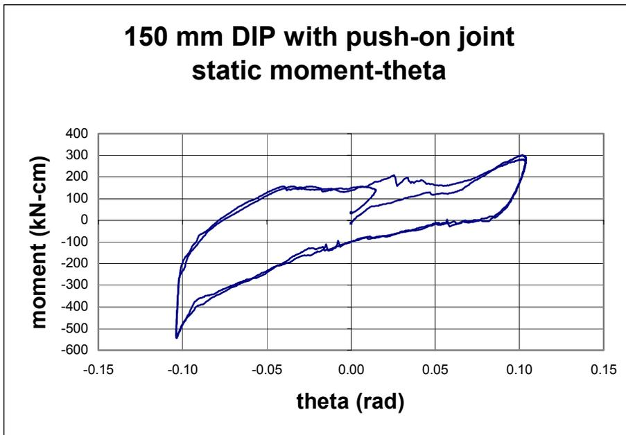
**Figure C-4 Static Moment-Theta for 150 mm DIP with Push-On Gasket**
