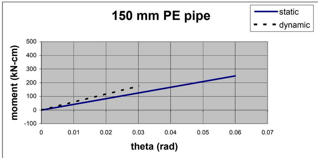
Figure 4-18 Moment-Theta Plot for 150 mm Diameter PE Pipe
