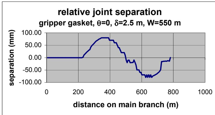
**Figure 5-27 Joint Separation for Gripper Gasket Joints on the Main Branch Loaded in the  $\theta = 0$  Direction (Global X)**
