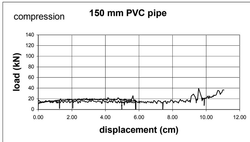
Figure A-18 Load-Displacement for 150 mm PVC Pipe
