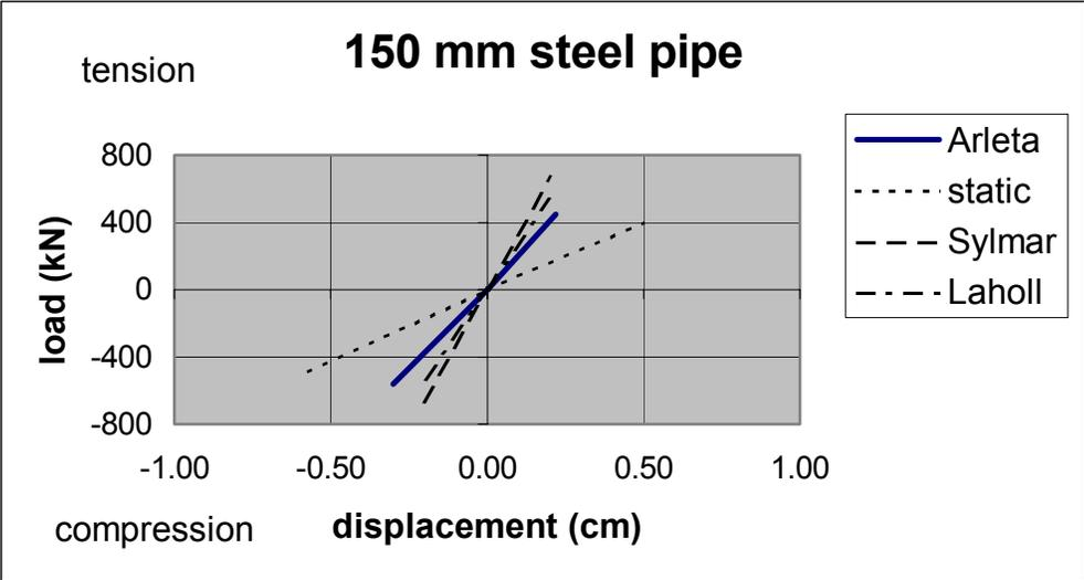
Figure 3-20 Load-Displacement Curves for 150 mm Steel Pipe
