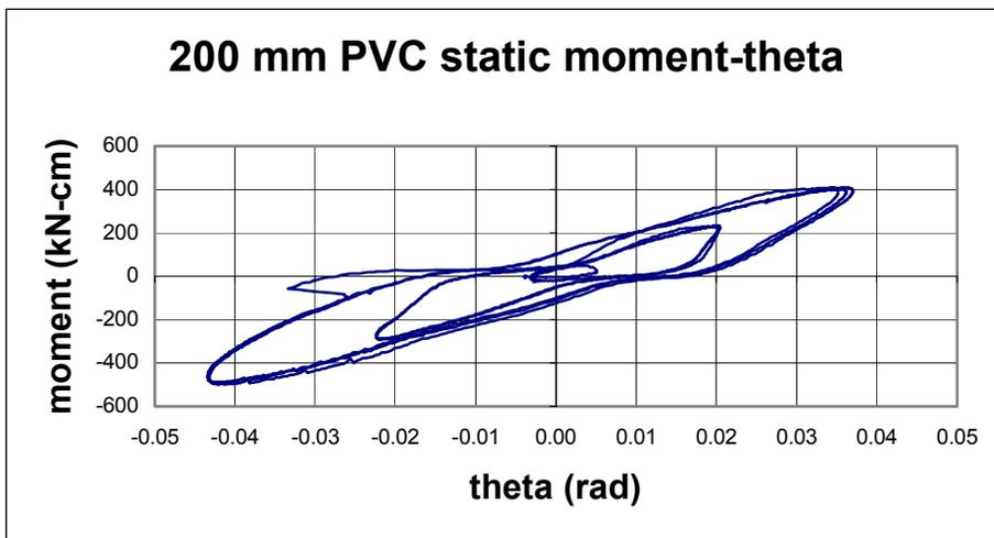
**Figure C-26 Static Moment-Theta for 200 mm PVC Pipe**
