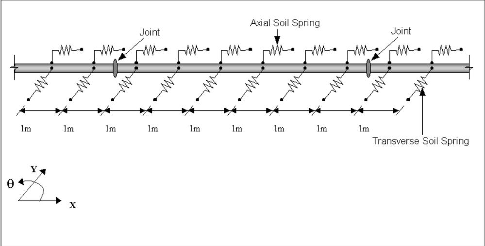
**Figure 5-5 Piping System Elements (Ref: Kuruswamy 2002)**
