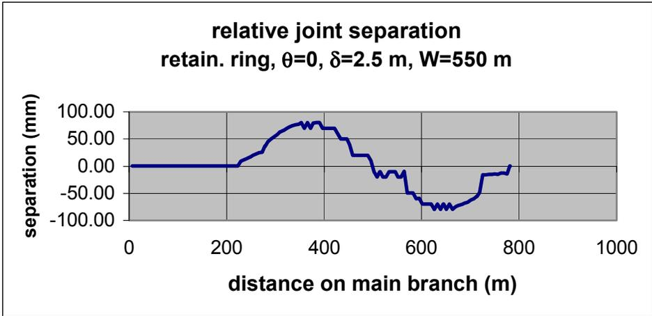
**Figure 5-23 Joint Separation for Retaining Ring Joints on the Main Branch Loaded in the  $\theta = 0$  Direction (Global X)**
