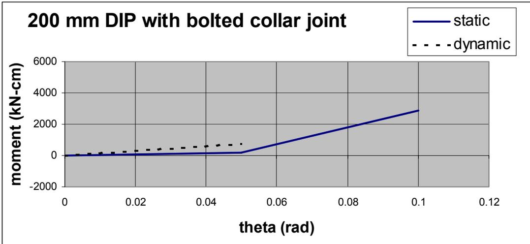
**Figure 4-13 Moment-Theta Plot for 200 mm Diameter Ductile Iron Pipe with Bolted Collar Joint**
