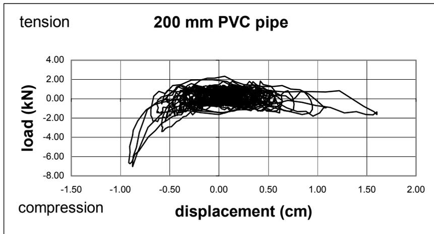
Figure B-13 Load-Displacement for 200 mm PVC Pipe
