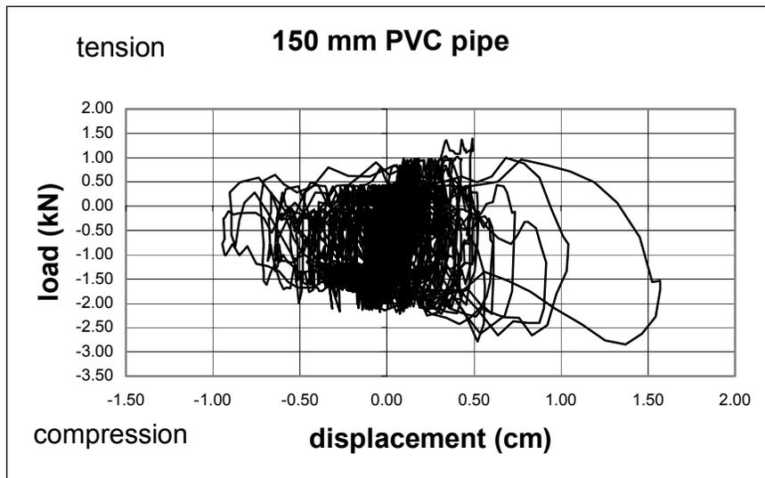
Figure B-12 Load-Displacement for 150 mm PVC Pipe
