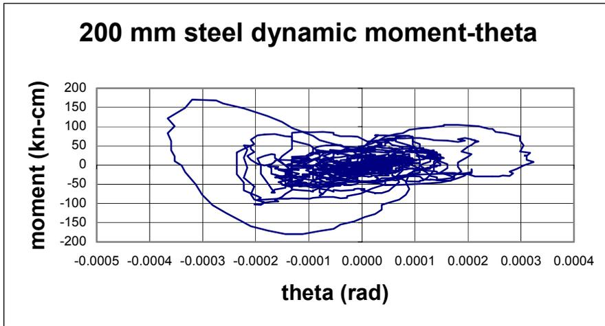
**Figure C-21 Dynamic Moment-Theta for 200 mm Steel Pipe**
