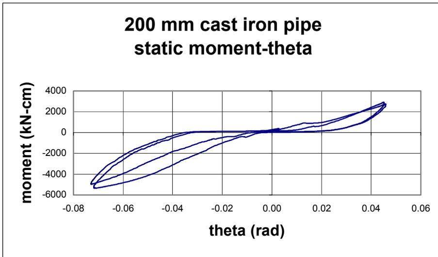
**Figure C-2 Static Moment-Theta for 200 mm Cast Iron Pipe**
