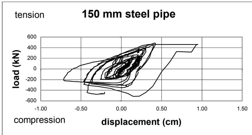
Figure B-10 Load-Displacement for 150 mm Steel Pipe
