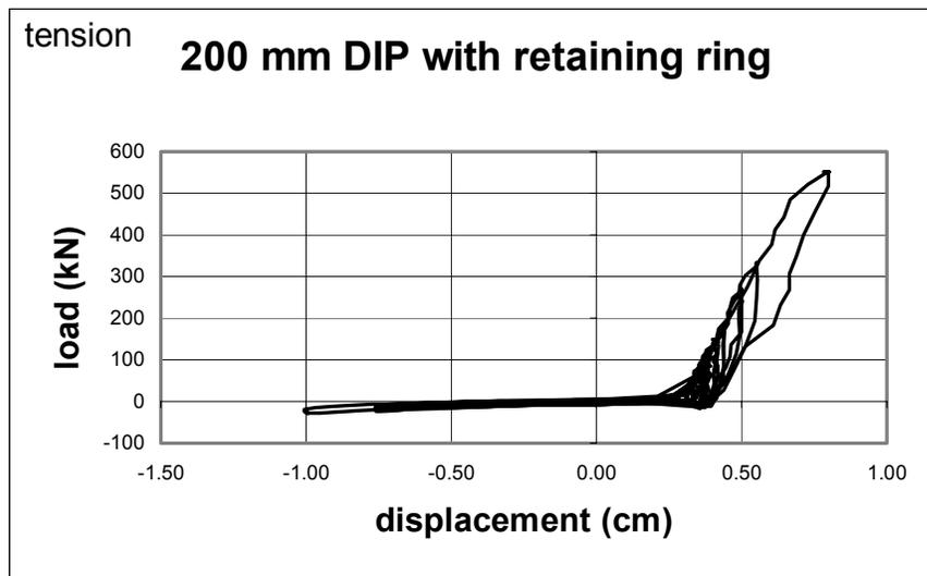
Figure B-7 Load-Displacement for 200 mm DIP with Retaining Ring Joint
