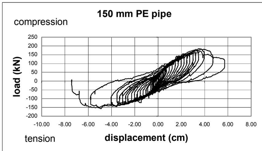
Figure A-21 Load-Displacement for 150 mm PE Pipe
