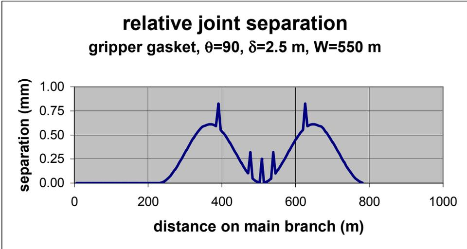
**Figure 5-29 Joint Separation for Gripper Gasket Joints on the Main Branch Loaded in the  $\theta = 90$  Direction (Global Y)**
