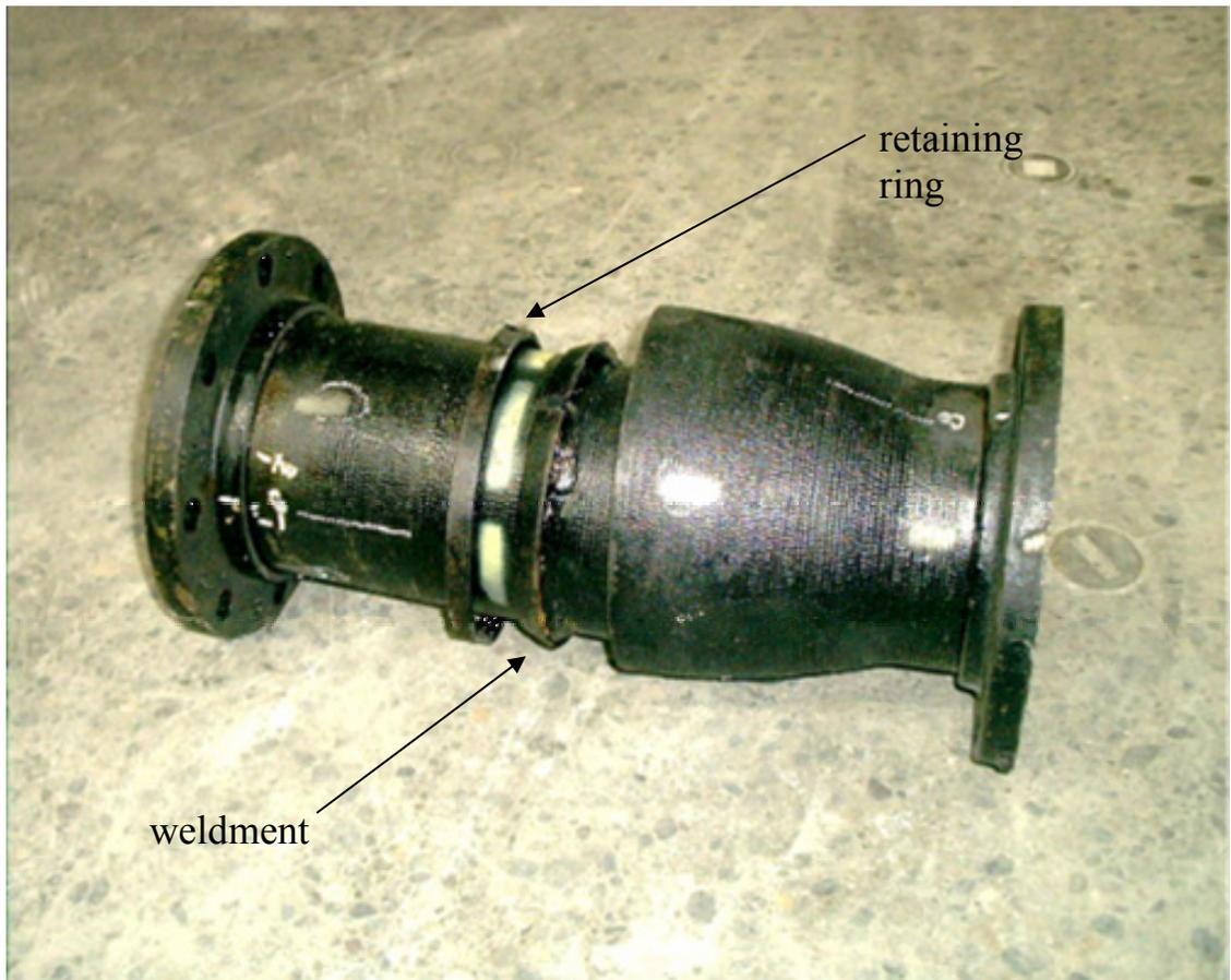
**Figure 1-12 Ductile Iron Pipe with Retaining Ring**
