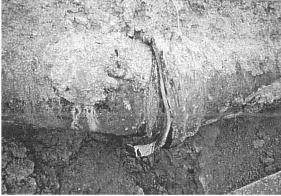
**Figure 1-5 Slip-Out of Joint on 450 mm Dia. Cast Iron Pipe from the Kobe Earthquake (Ref: Iwamoto 1995)**
