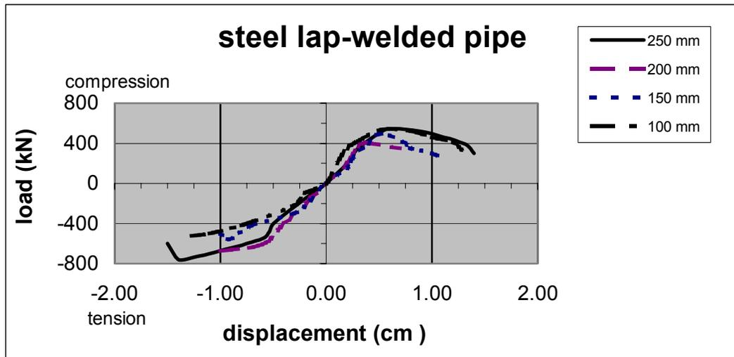
**Figure 2-12 Load-Displacement for Steel Pipe with Lap-Welded Joints**
