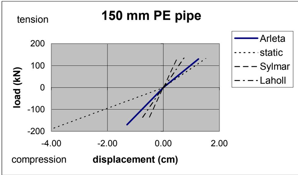
**Figure 3-24 Load-Displacement Curves for 150 mm PE Pipe**
