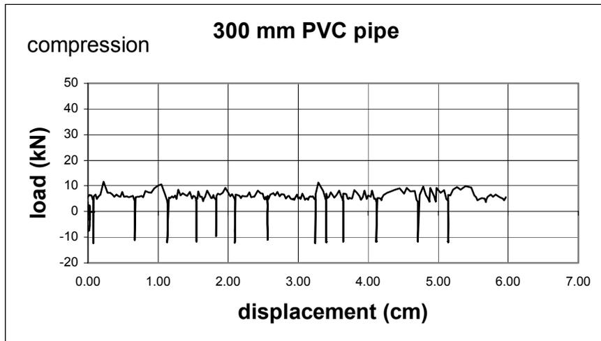
Figure A-20 Load-Displacement for 300 mm PVC Pipe
