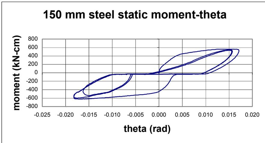
**Figure C-20 Static Moment-Theta for 150 mm Steel Pipe**
