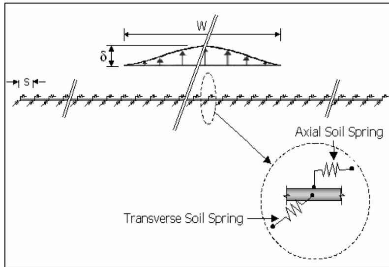
**Figure 5-7 Straight Piping System Model with Soil Springs
