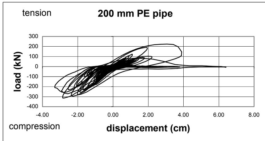
Figure B-15 Load-Displacement for 200 mm PE Pipe
