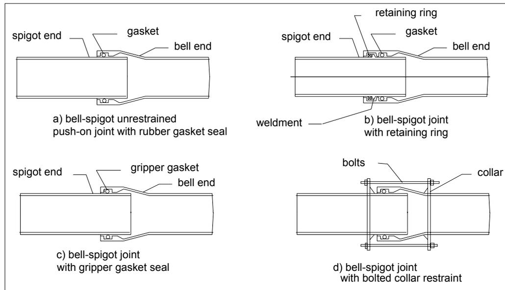
**Figure 1-9 Joint Types for Ductile Iron Pipe**
