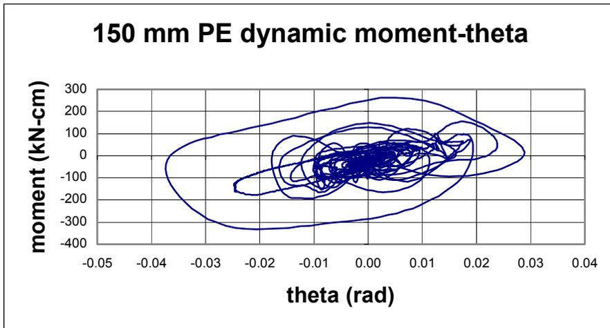
**Figure C-27 Dynamic Moment-Theta for 150 mm PE Pipe**
