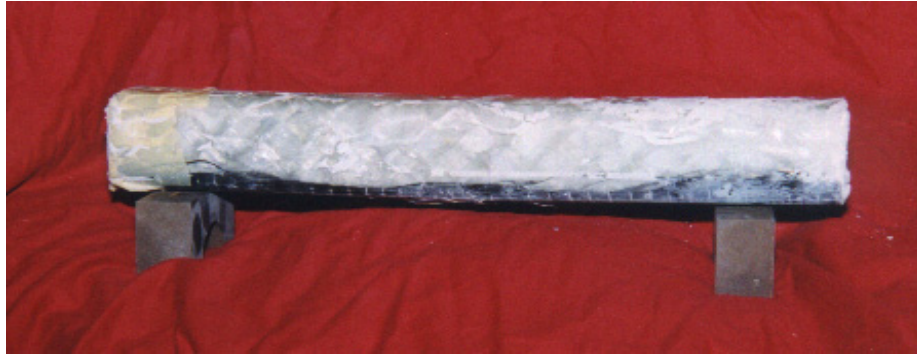
Figure 6 Picture of concrete filled hybrid GFRP/CFRP tube after failure
