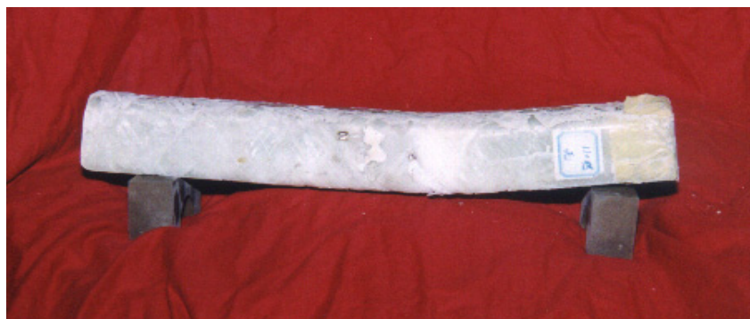
Figure 5. Picture of concrete filled GFRP tube after failure
