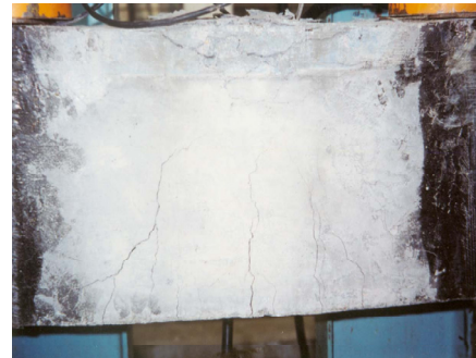
Figure 4 Flexural failure of SBF1
