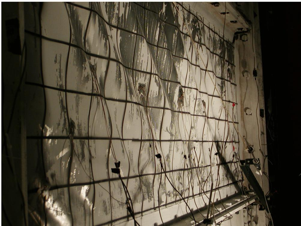
**FIGURE 5-44 Infill Buckling (Specimen F2, Cycle 18,  $+5\delta_y$ )**
