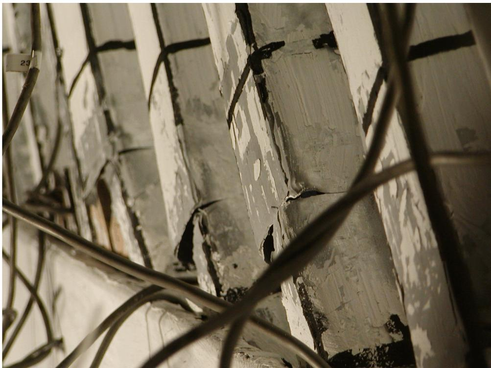
**FIGURE 5-24 Fractures Along Line 2 (Specimen C1, Cycle 16, +3 $\delta_y$ )**
