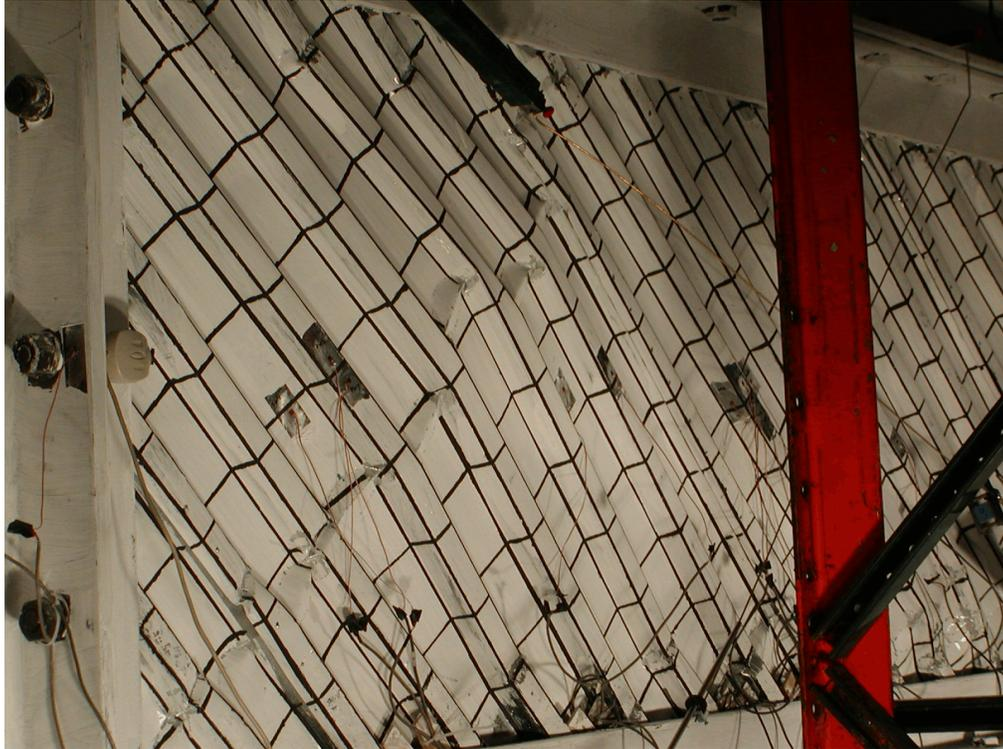
**FIGURE 5-19 North Section (Specimen C1, Cycle 15,  $-2\delta_y$ )**
