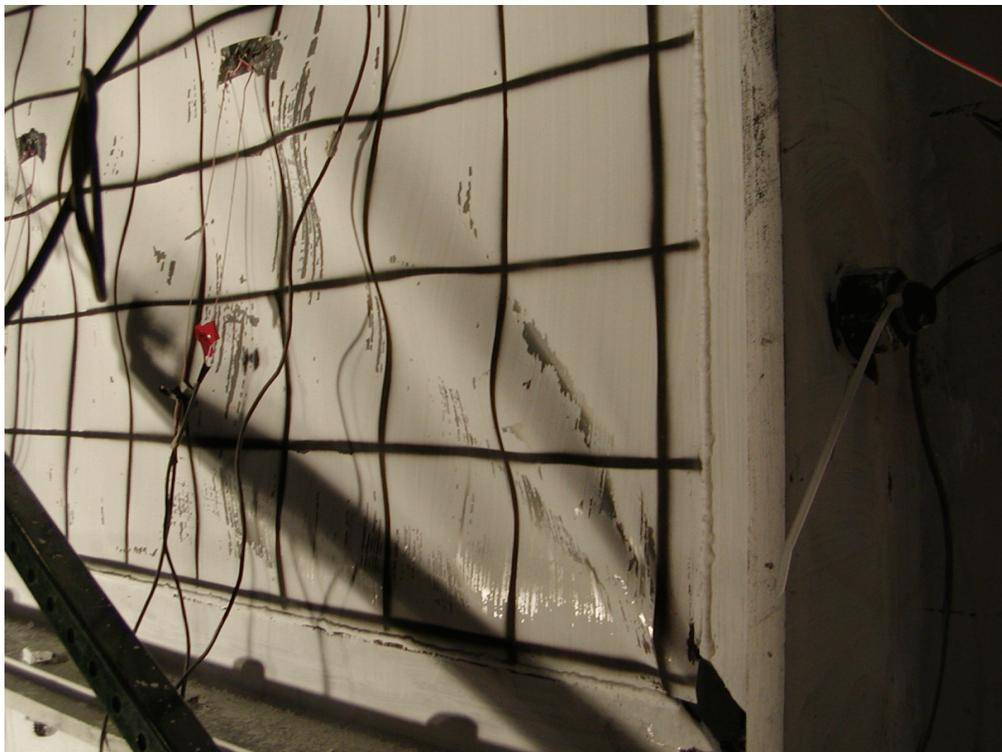
**FIGURE 5-42 Plastic Fold in Lower South Corner
