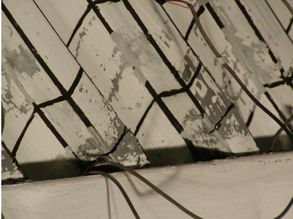
**FIGURE 5-23 Fractures Along Line 2 (Specimen C1, Cycle 16, +3 $\delta_y$ )**
