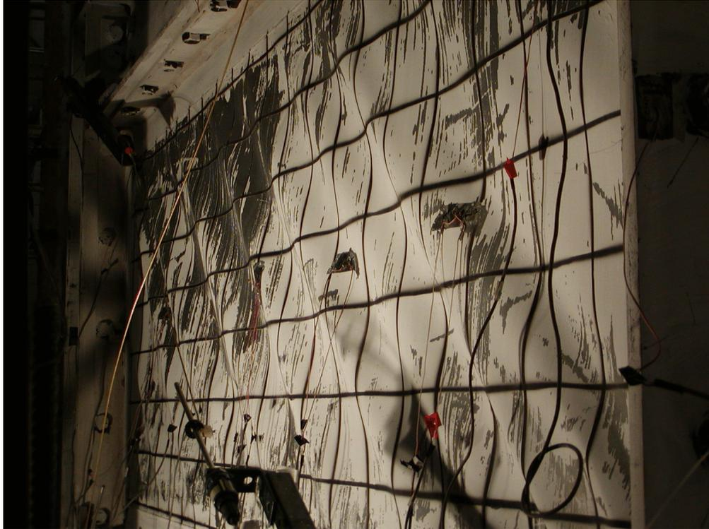
**FIGURE 5-49 Infill Buckling (Specimen F2, Cycle 20,  $+6\delta_y$ )**
