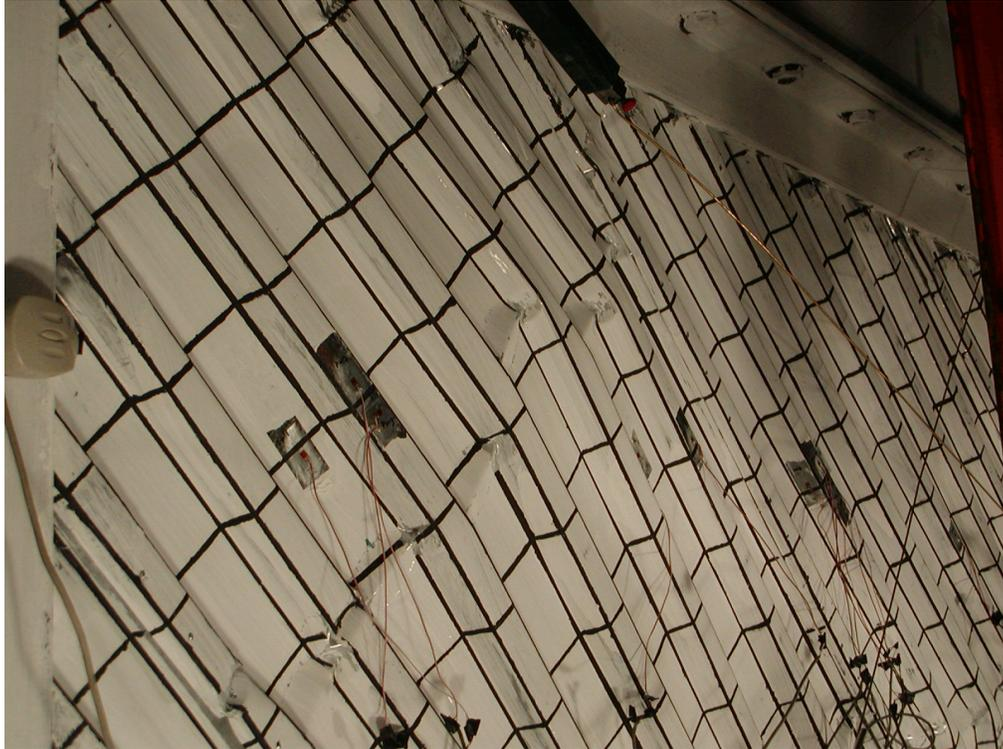
**FIGURE 5-17 Local Buckling Along Line 1
