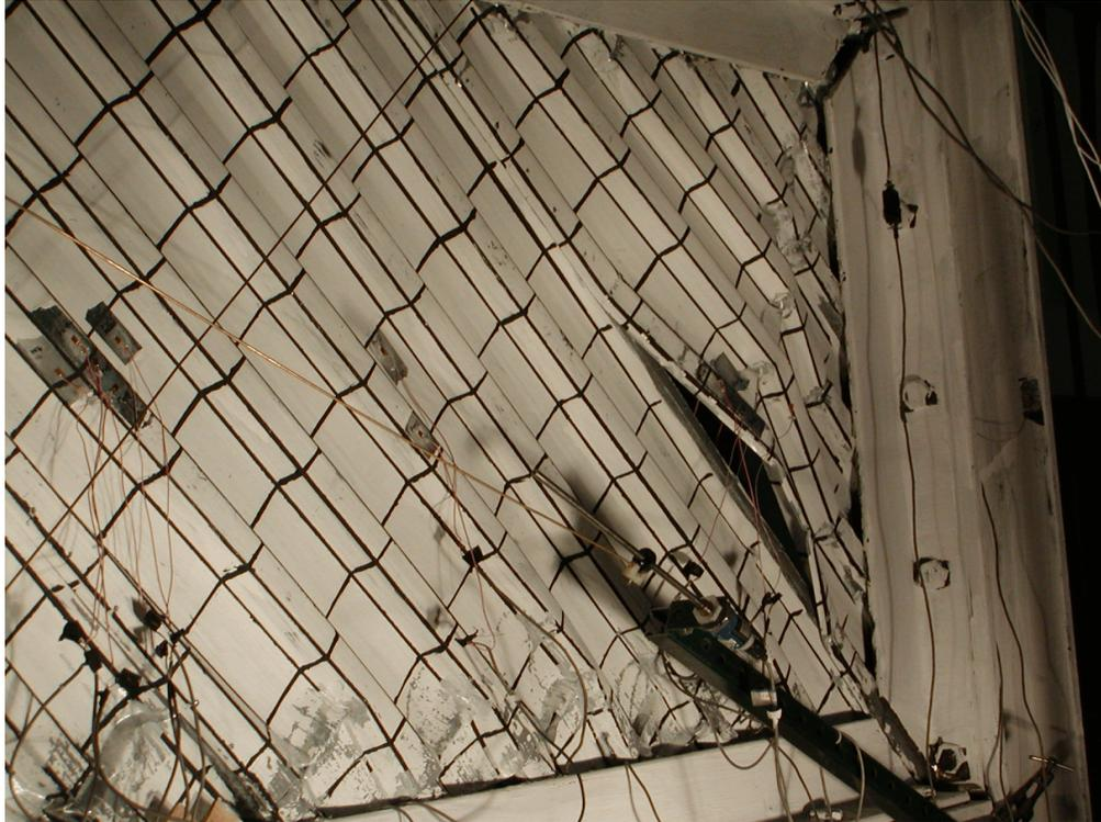
**FIGURE 5-27 Local Buckling Along Lines 2 and 3
