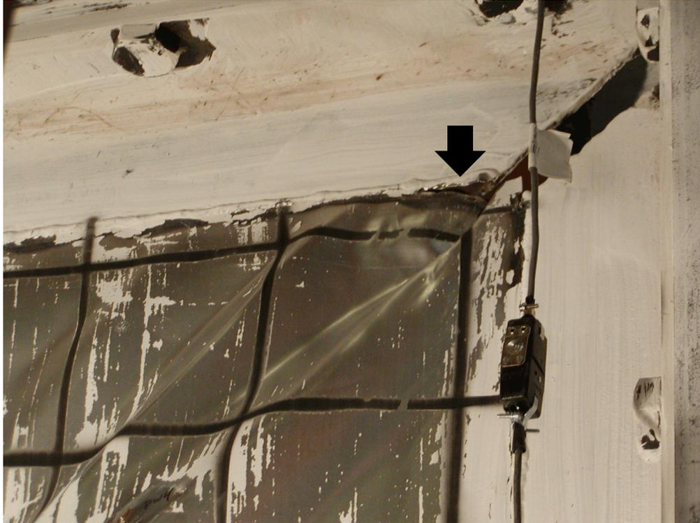
**FIGURE 5-55 Infill Fracture in Upper South Corner
