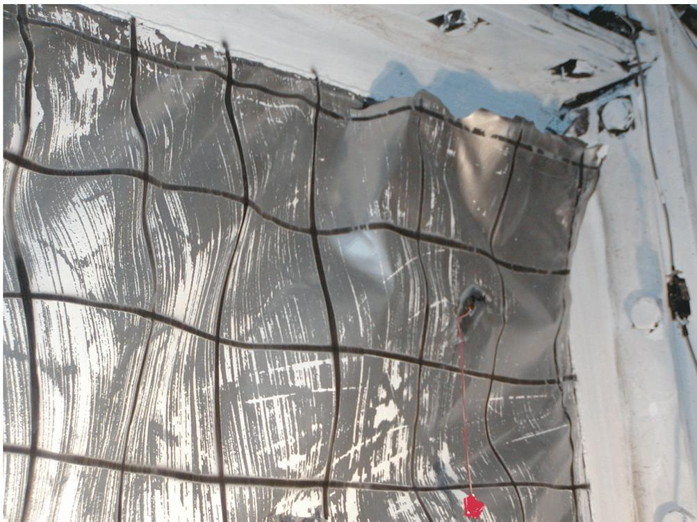
**FIGURE 5-66 Infill Fracture in Upper South Corner
