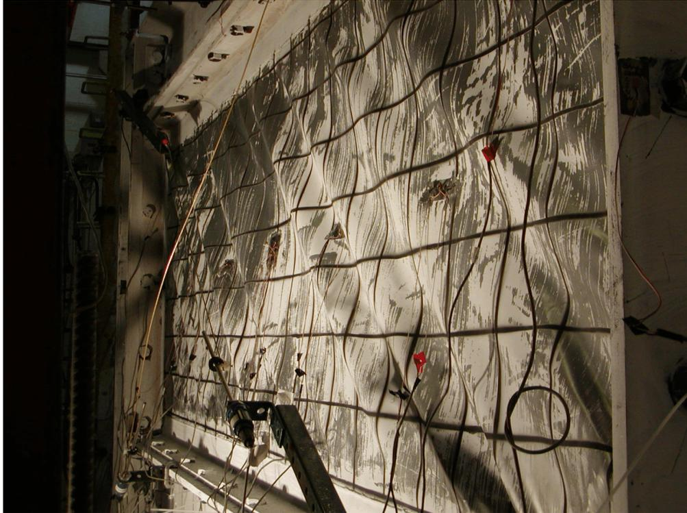
**FIGURE 5-63 Infill Buckling (Specimen F2, Cycle 29,  $+12\delta_y$ )**
