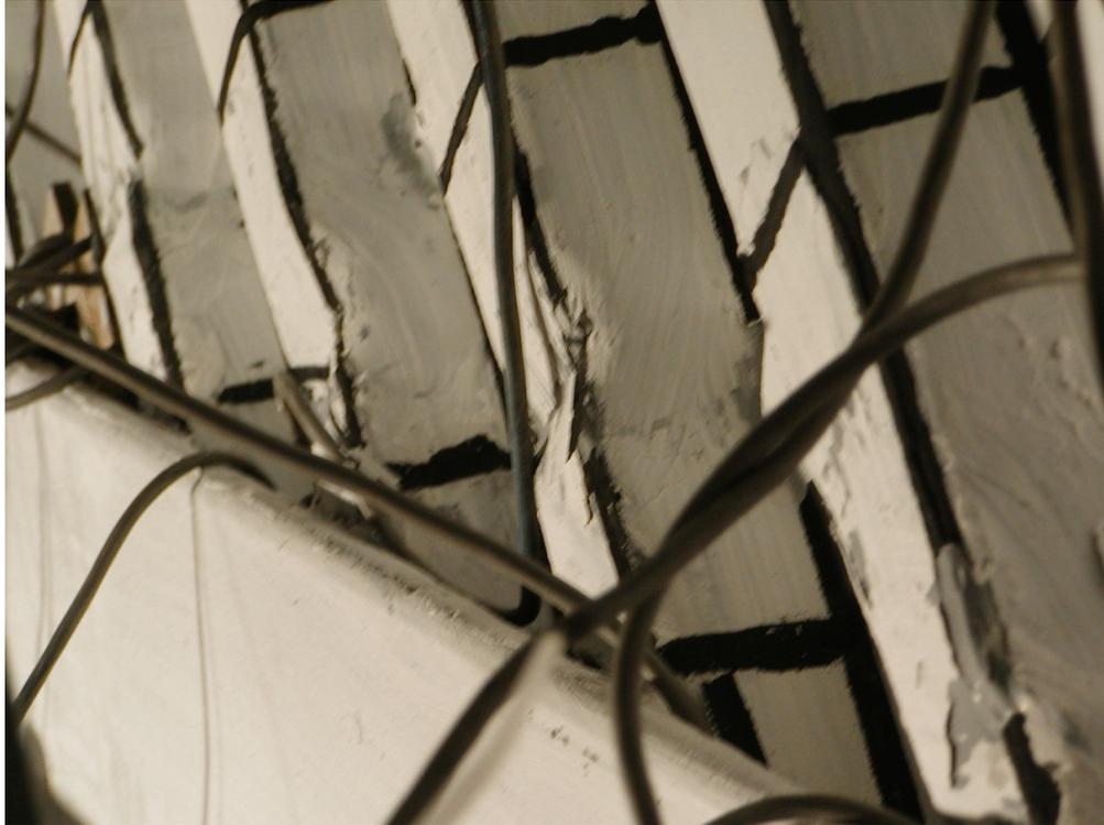
**FIGURE 5-11 Local Buckling Along Line 2
