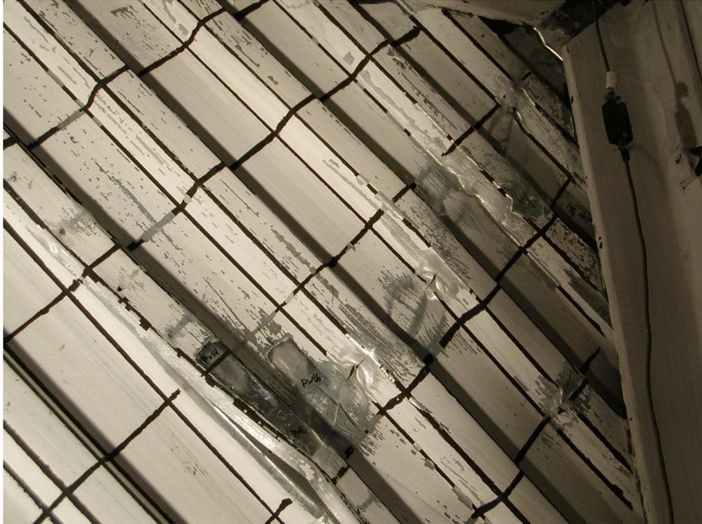
**FIGURE 5-31 Fractures Along Line 3 (Specimen C1, Cycle 19,  $+4\delta_y$ )**
