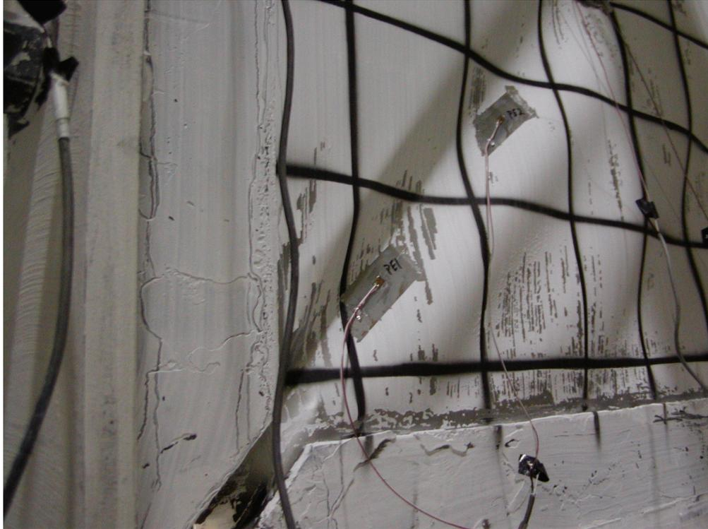
**FIGURE 5-43 Plastic Folds in Lower South Corner
