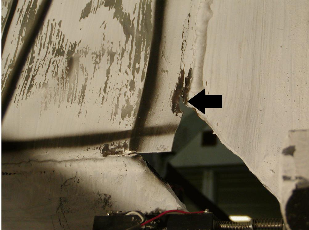
**FIGURE 5-45 Infill Fracture in Lower South Corner
