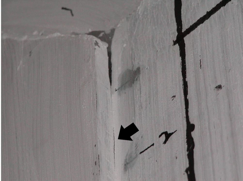
**FIGURE 5-5 Epoxy Crack - Top of South Column
