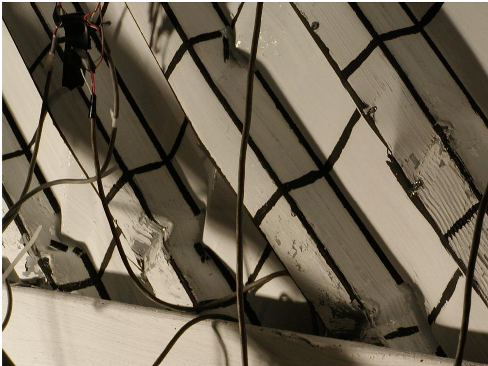
**FIGURE 5-14 Local Buckling Along Line 2
