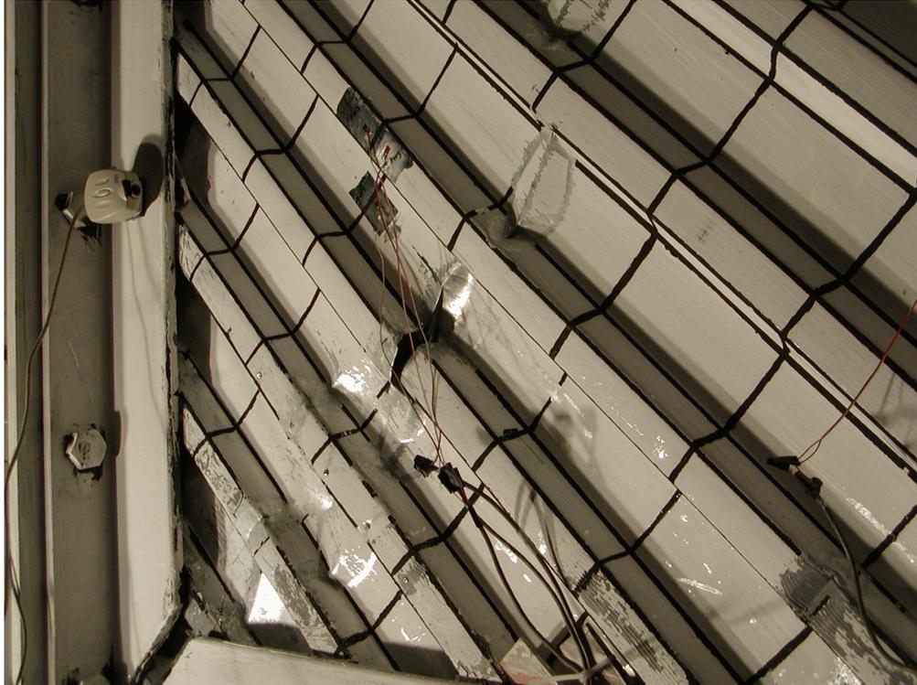
**FIGURE 5-29 Fractures Along Line 1 (Specimen C1, Cycle 19, +4 $\delta_y$ )**
