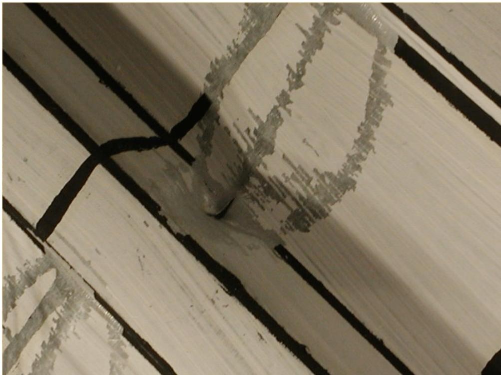
**FIGURE 5-28 Fracture Along Line 1 (Specimen C1, Cycle 18,  $+3\delta_y$ )**
