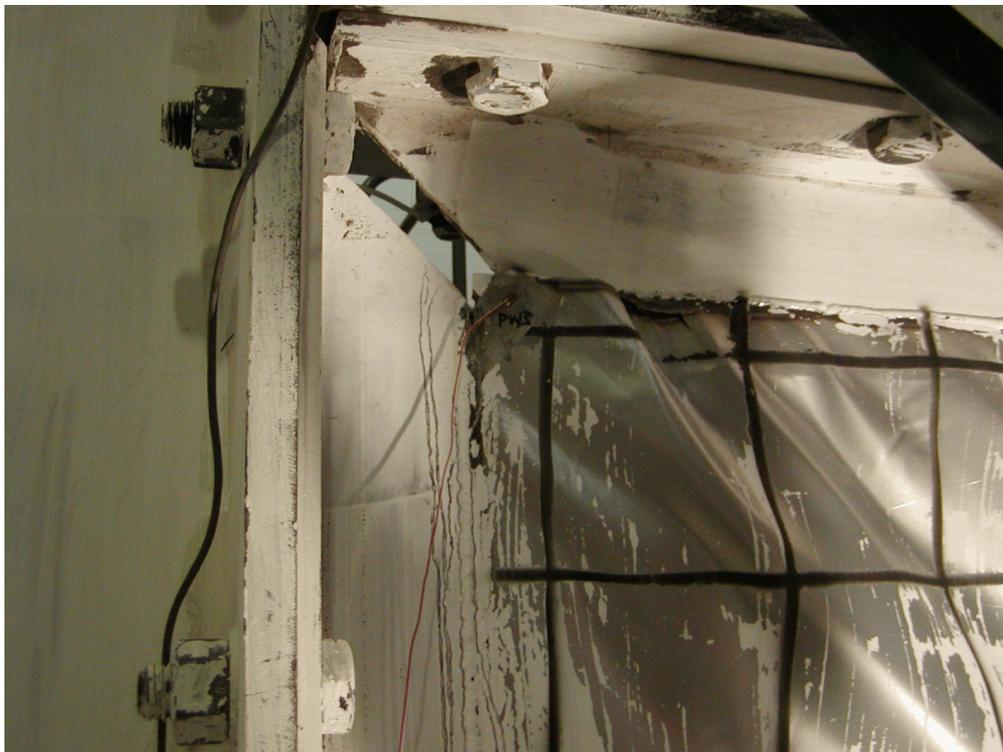
**FIGURE 5-60 Infill Fracture in Upper North Corner
