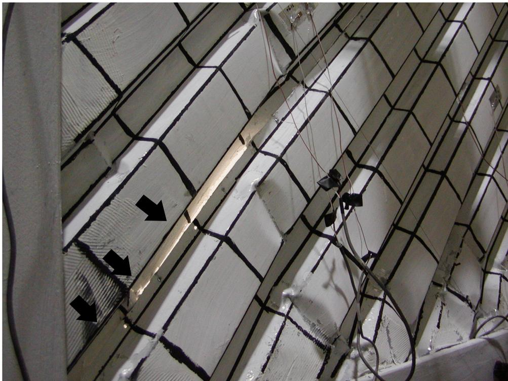
**FIGURE 5-22 Failed Pop-rivets (Specimen C1, Cycle 13,  $-2\delta_y$ )**
