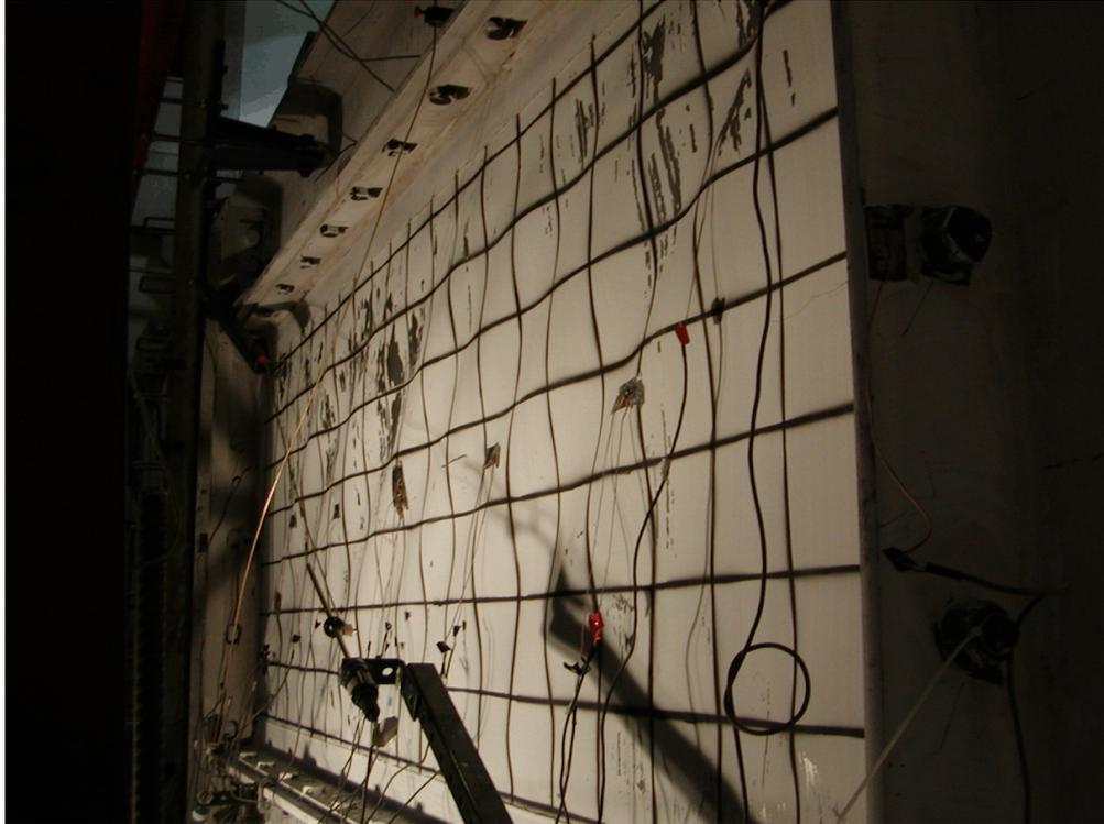
**FIGURE 5-35 Infill Buckling (Specimen F2, Cycle 15,  $-3\delta_y$ )**
