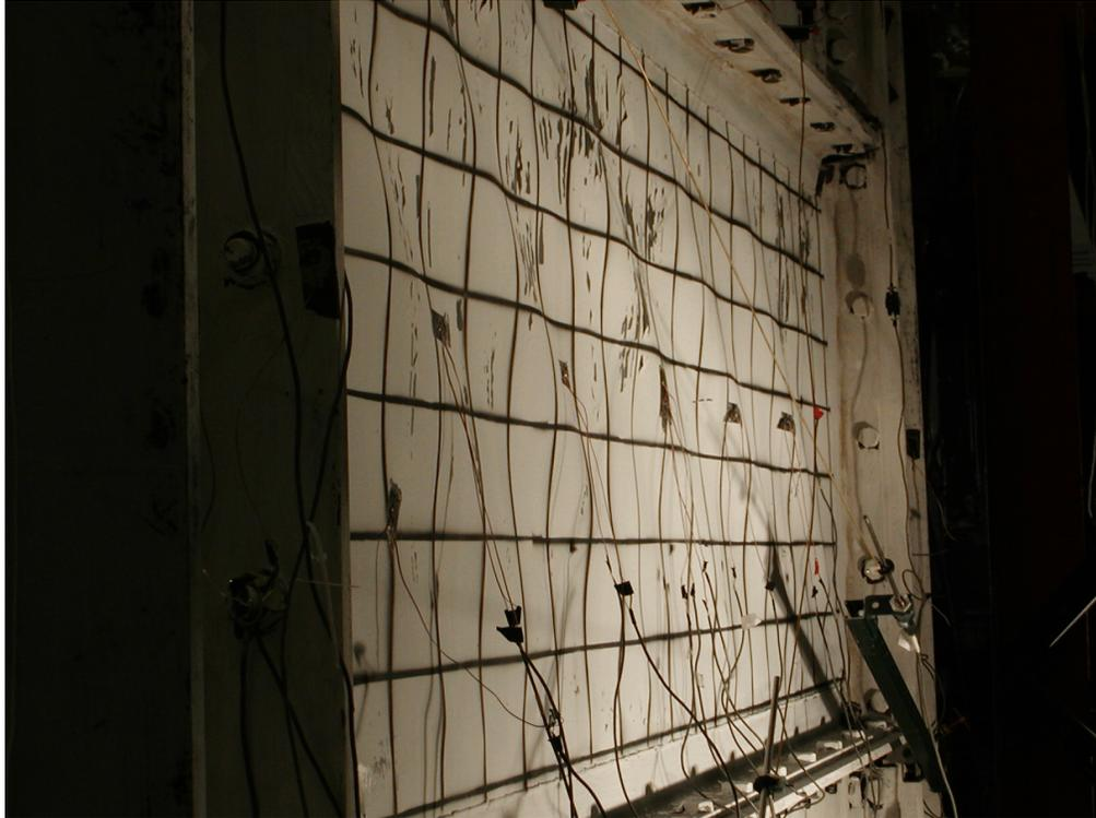
**FIGURE 5-33 Infill Buckling (Specimen F2, Cycle 12, +2 $\delta_y$ )**
