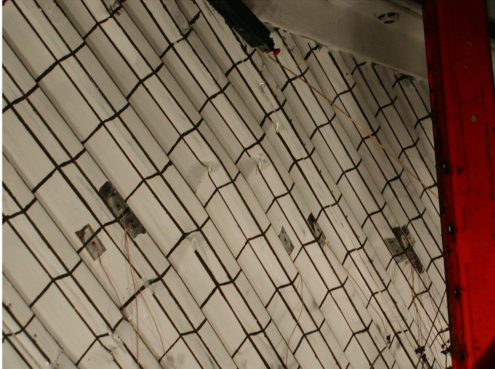
**FIGURE 5-13 Local Buckling Along Line 1
