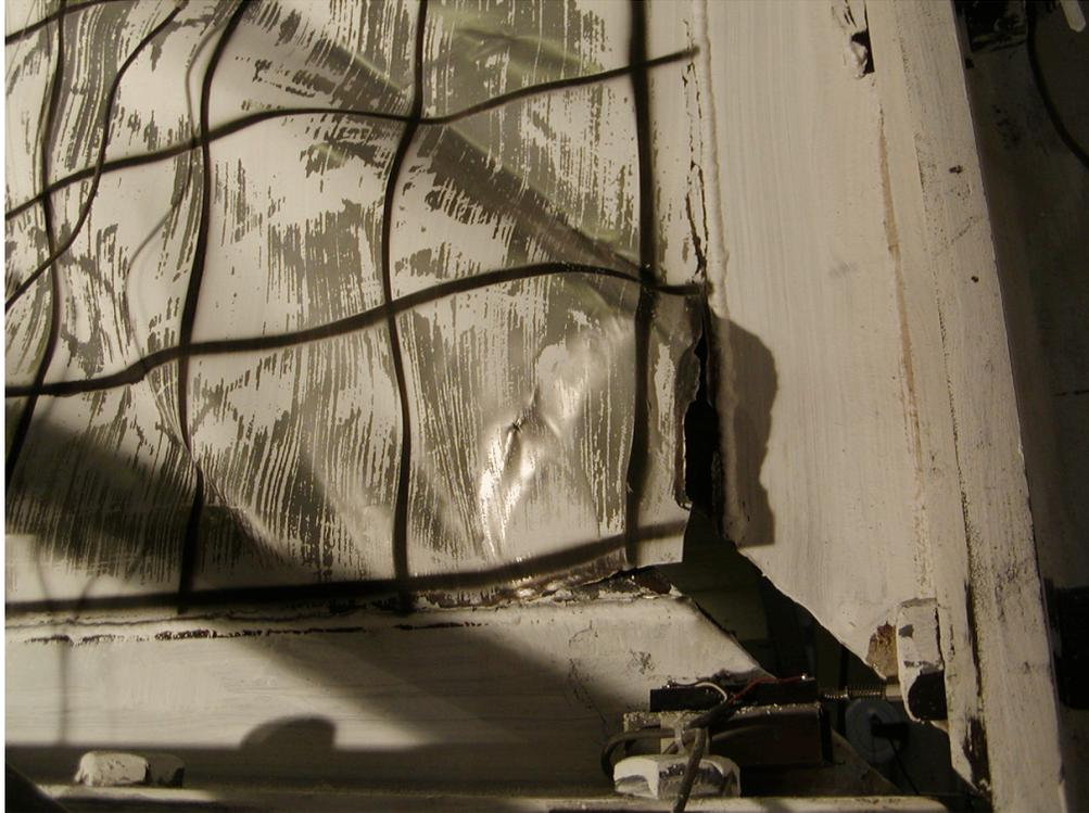
**FIGURE 5-59 Infill Fracture in Lower South Corner
