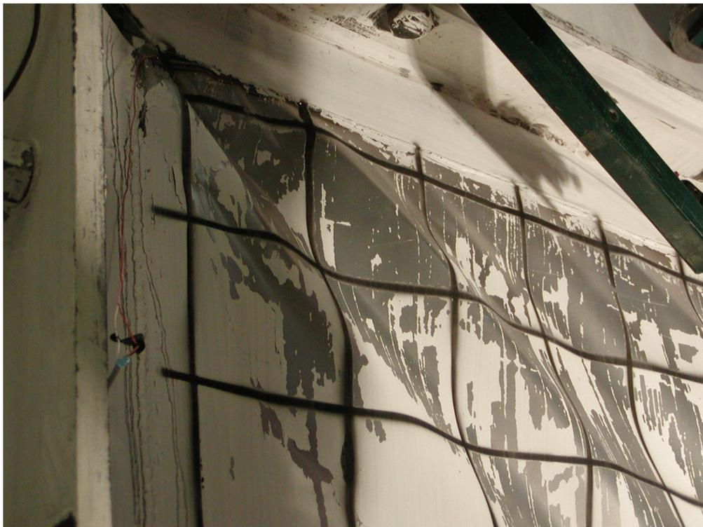
**FIGURE 5-48 Plastic Fold in Upper North Corner
