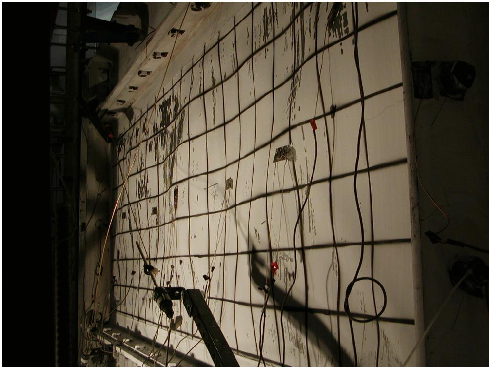
**FIGURE 5-36 Residual Buckling at Zero Load (Specimen F2, Cycle 15)**
