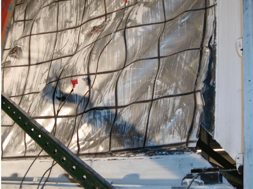
**FIGURE 5-67 Infill Fracture in Lower South Corner
