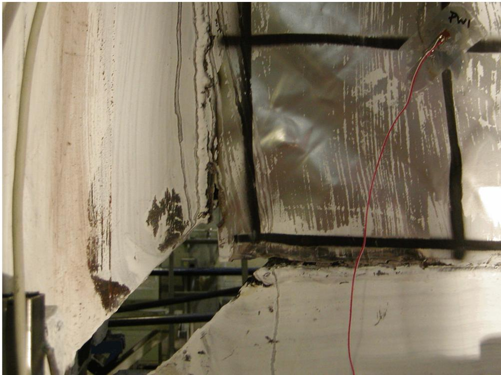
**FIGURE 5-62 Infill Fracture in Lower North Corner (Specimen F2, Cycle 26, +10 $\delta_y$ )**
