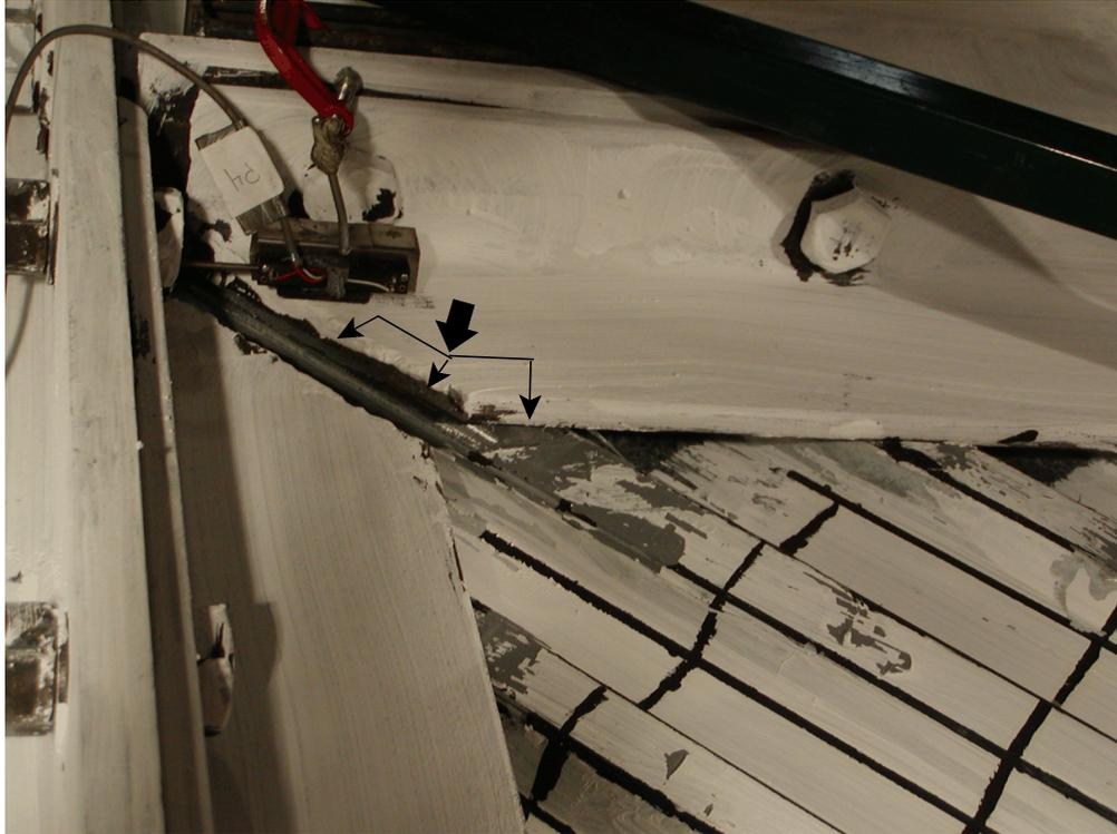
**FIGURE 5-25 Epoxy Crack in Upper North Corner
