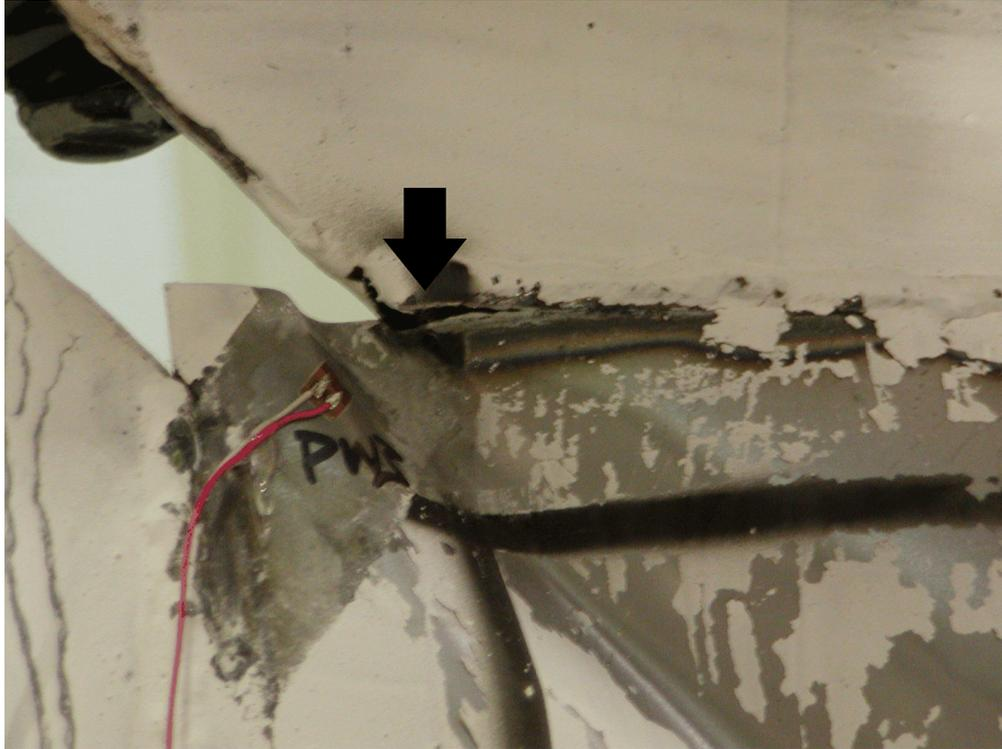
**FIGURE 5-41 Infill Fracture in Upper North Corner
