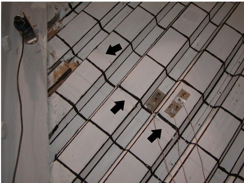
**FIGURE 5-12 Local Buckling Along Line 3
