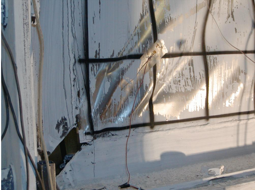
**FIGURE 5-47 Plastic Fold in Lower North Corner
