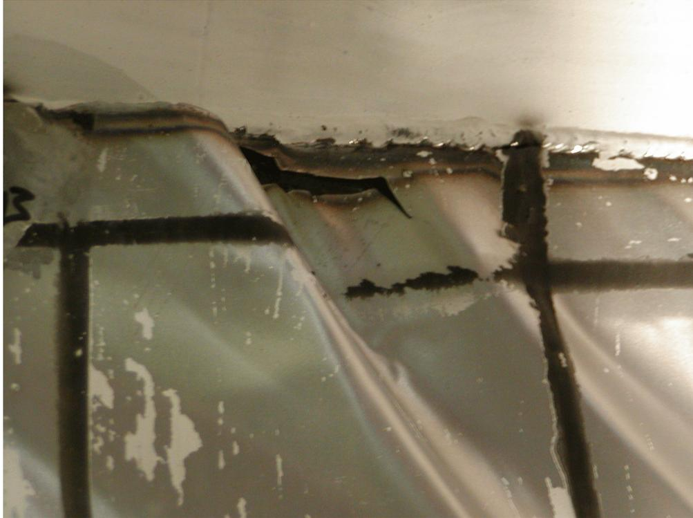
**FIGURE 5-61 Infill Fracture in Upper North Corner Redirecting Towards Center of Infill (Specimen F2, Cycle 26, +10 $\delta_y$ )**
