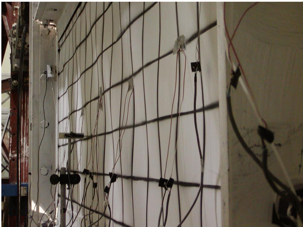
**FIGURE 5-32 Infill Buckling (Specimen F2, Cycle 9,  $-1\delta_y$ )**
