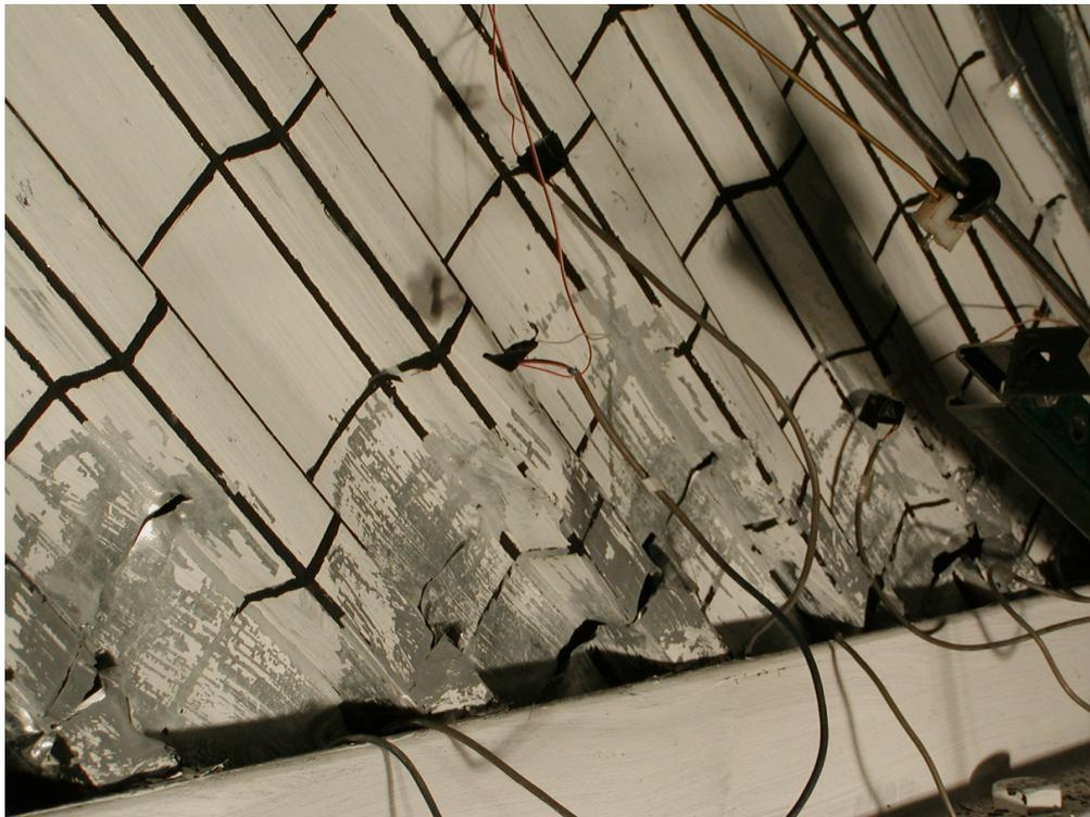
**FIGURE 5-30 Fractures Along Line 2 (Specimen C1, Cycle 19, +4 $\delta_y$ )**
