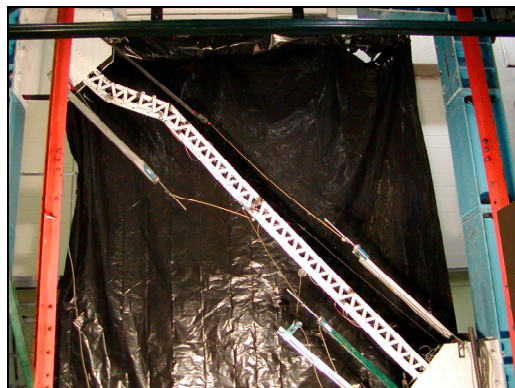
Figure 20. Global buckling for Bx8-120
