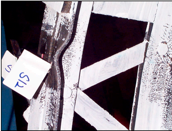
Figure 21. Buckling for Ay8-60
