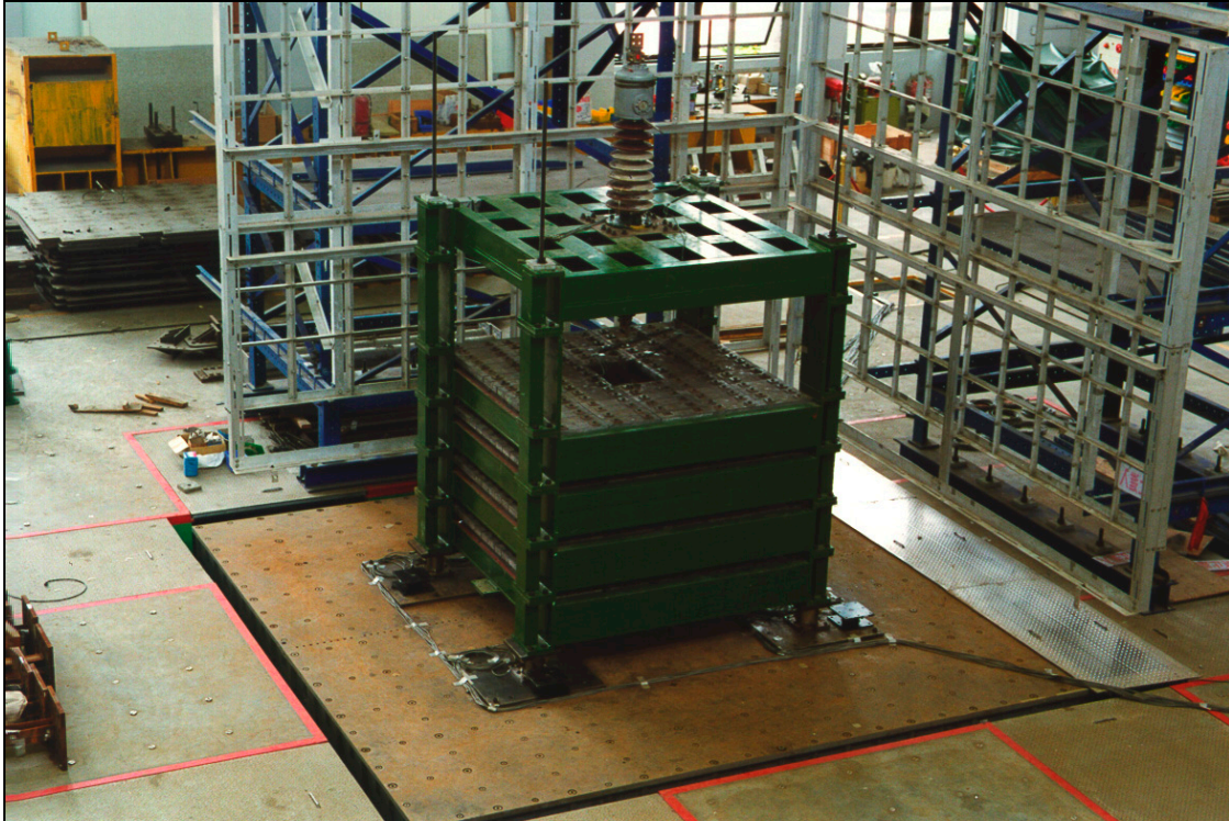
Figure 1. Experimental model of transformer-bushing on shaking table
