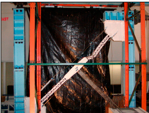
Figure 19. Global buckling for Bx8-60
