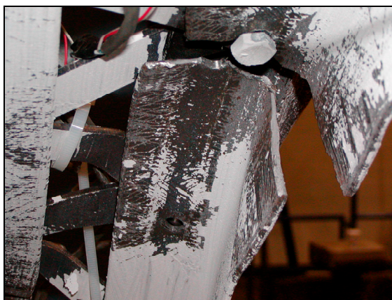
Figure 25. Buckling of Bx8-60
