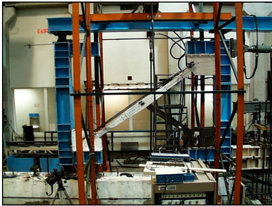
Figure 5. Test set-up for specimen Ay16-60
