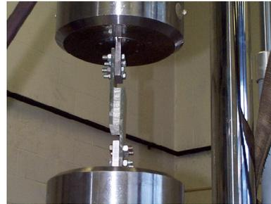
(b) Visco-elastic Material Test
