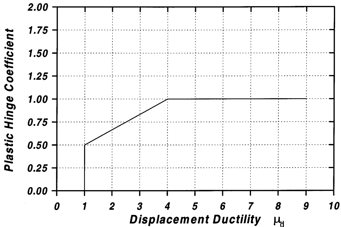
Figure 5-12 Plastic Hinge Coefficient vs. Displacement Ductility
