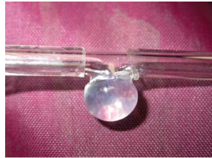
Figure 9: Picture of aneurysm model post fibrin injection and after delivery system removal
