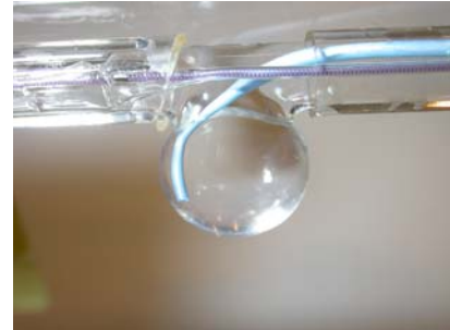
Figure 6: Picture of glass aneurysm model with steam shaped microcatheter placed in dome
