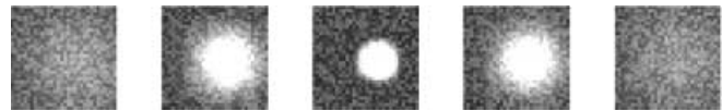
Fig. 10. A simulated single particle image (30 \mu\text{m} ) on selected planes (separated by 100 \mu\text{m} along z ). The image area shown consists of 32 \times 32 pixels
