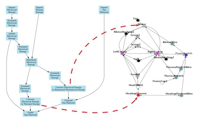
Fig. 2 The functional model (left) and CFG (right) for a hair dryer are shown. Two of the rules that are empirically extracted from the graphs are captured by the dashed arrows.
