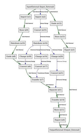
Fig. 5 Functional model of a peanut sheller
