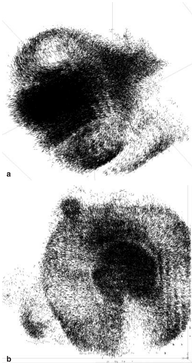
Fig. 9a, b. Detailed 3D velocity vector field after particle pairing: a side view. b top view. Approximately 92,000 velocity vectors are inhomogeneously distributed. A velocity vector field on a regular grid can be generated from this data by interpolation
