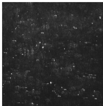
Figure 13: One plane of reconstructed particle images in a 9 \times 9 \text{ cm}^2 area out of the 3D holographic image volume, viewed by the CCD camera.
