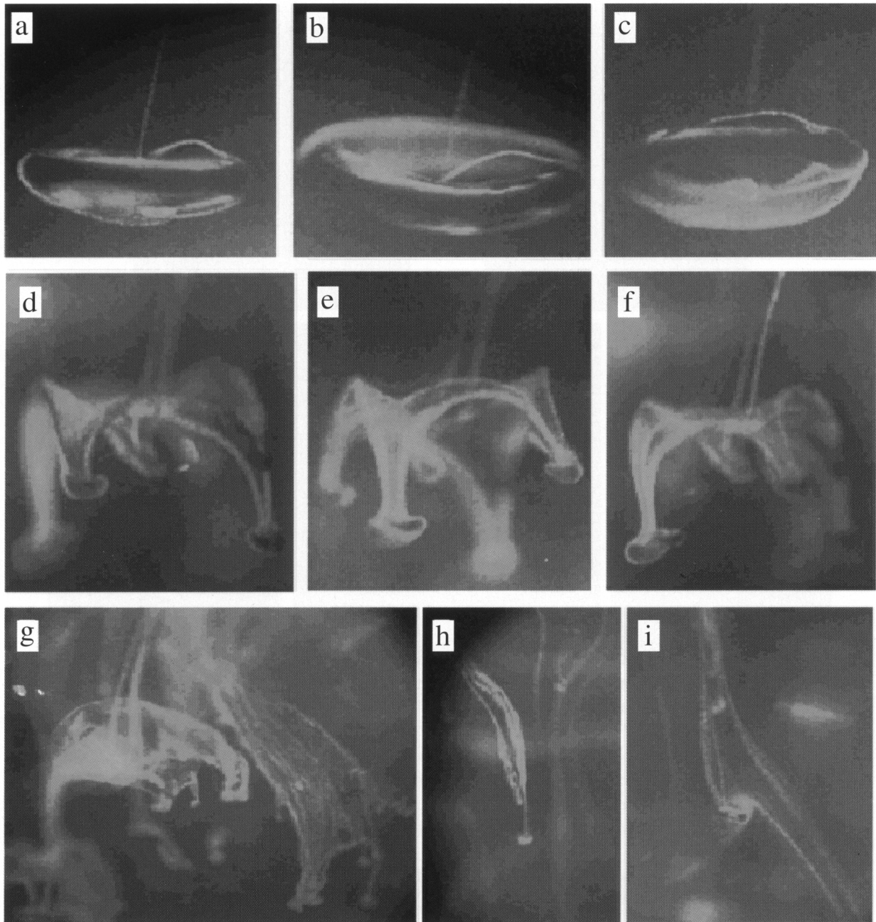
Fig. 2. Holographic images of polymer-suspension drop falling in water undergoing vortex-ring instability, photographed from 3D images reconstructed from IROV holograms:
