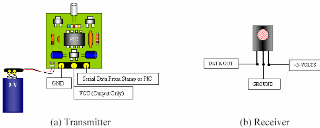
Figure 3: IR Communications Components and Setup.
