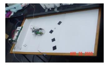
Assembly of the Mobile Robot: We began the project by assembling the mobile BOE BOT robot. This involved fixing the wheel and trying to get it properly aligned and giving it a motion.
