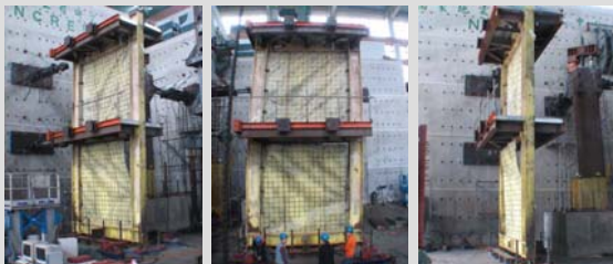
Specimen after interstory drift of 5%
