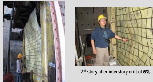
1 st Story after interstory drift of 5%
