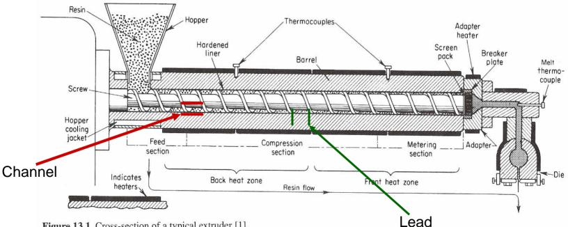
Figure 13.1 Cross-section of a typical extruder [1].
