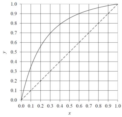
Guess  $x_D = 0.96 \rightarrow x_B = 0.04$  by overall mass balance (0.96, 0.96)  $F x_F = D x_D + B x_B$  $x_F = (D/F) x_D + [1 - (D/F)] x_B$ (050, 0.50)  $x_B = [x_F - (D/F) x_D] / [1 - (D/F)]$ = 0.480
