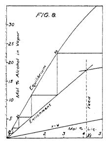
ration can be attained, but only with an infinite number of perfect plates; and finally, if the lines intersect at any point above x = y line and below the equilibrium curve, as point c, the separation can be effected with a finite number of plates. As the only means of moving the intersection from a to c is by increasing the overflow, by definition the minimum overflow is that overflow for which the rectifying line will intersect the  $x = x_l$  line at point b.
