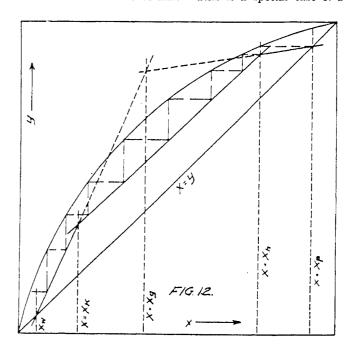
two-feed column where the second feed is one of the layers formed in the decanter. If this second feed is not at the boiling point the enrichment line for that part of the column below the entrance of the decanted feed must be modified as described under the section "Feed Not at Boiling Point."
